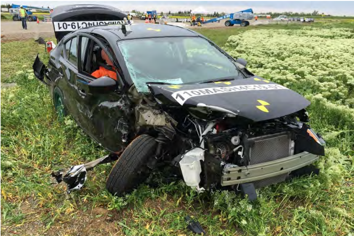
Figure 5-13 Test 4-10 Test Vehicle Damage (Front Right)
