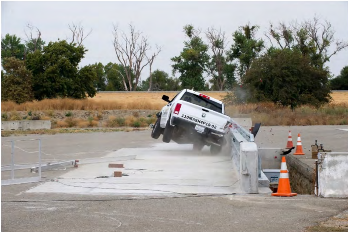
Figure 6-5 Test 4-11 Upstream Impact View
