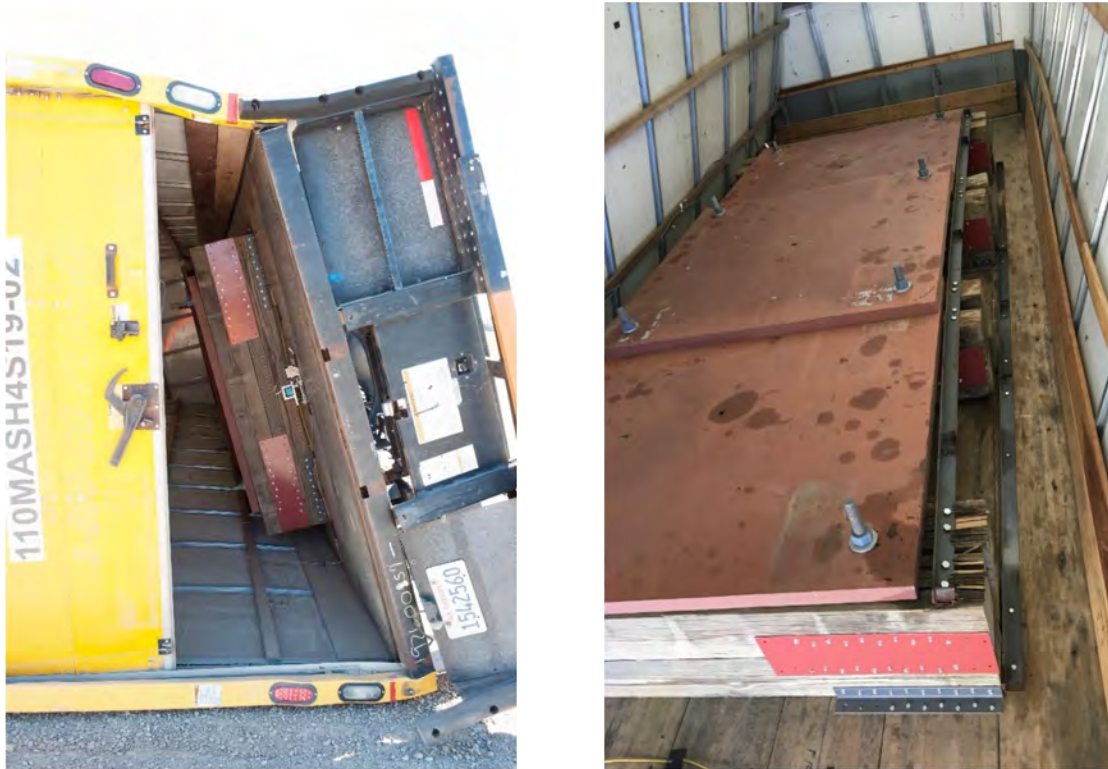
Figure 7-16 MASH 4-12 Test Vehicle Ballast After Impact
