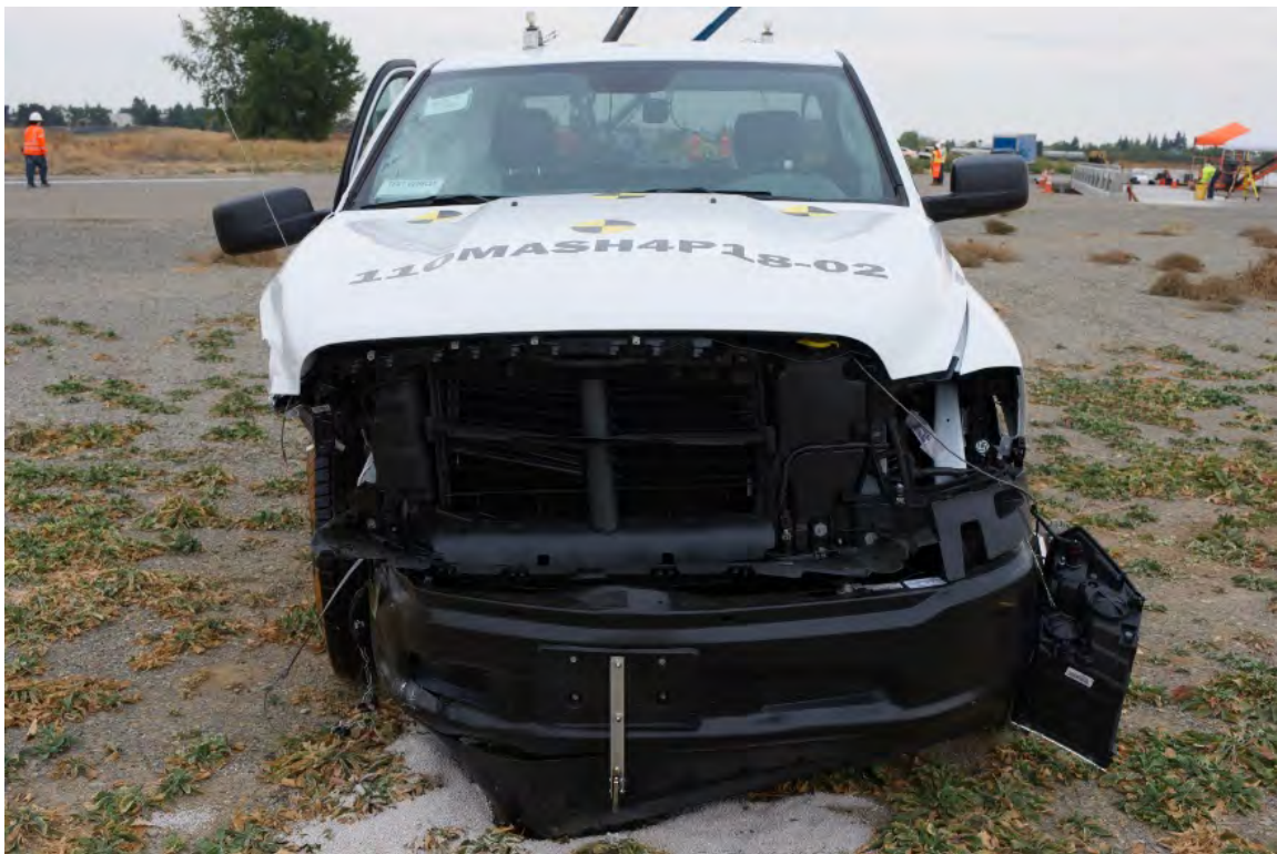
Figure 6-12 Test 4-11 Test Vehicle Damage (Front)
