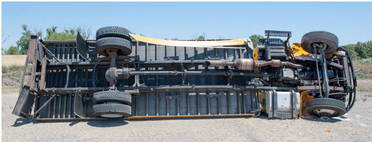
Figure 7-15 MASH 4-12 Test Vehicle Undercarriage After Impact
