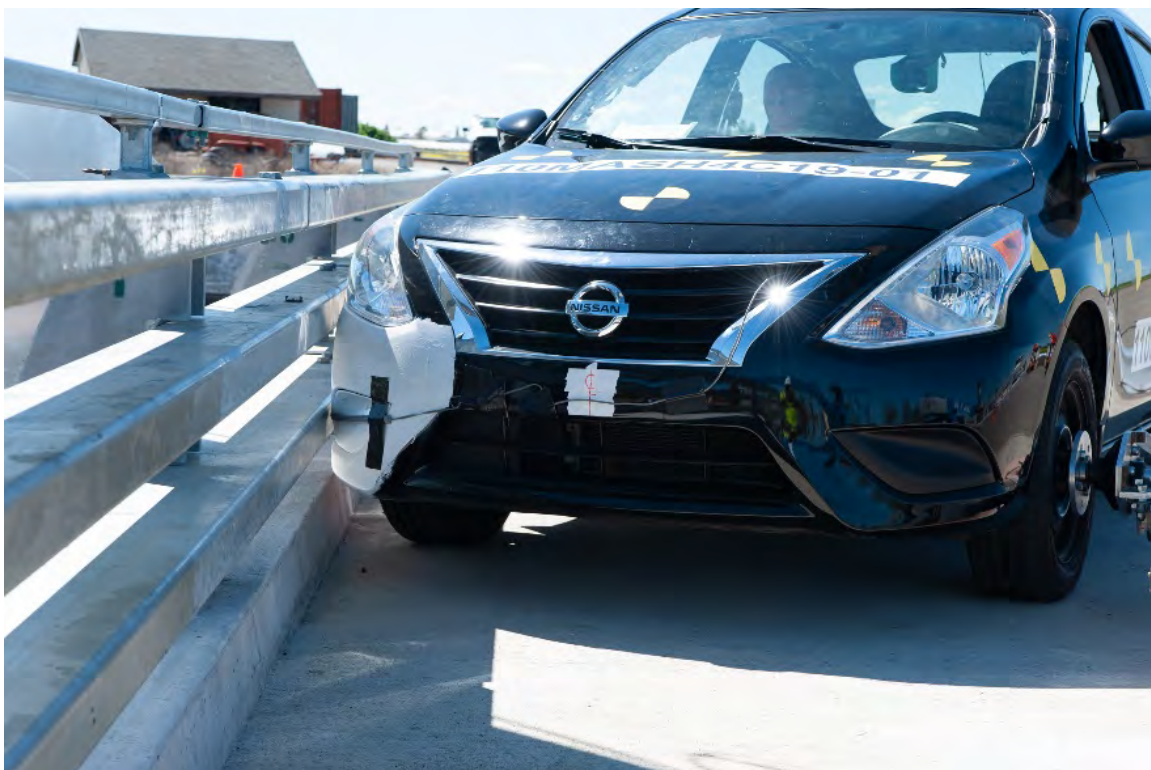
Figure 4-6 MASH 4-10 Test Vehicle at Impact Point
