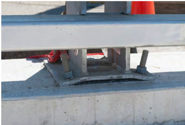
Figure 7-12 Test 4-12 Post 3 Bent Bottom Plate Close Up Post-Test
