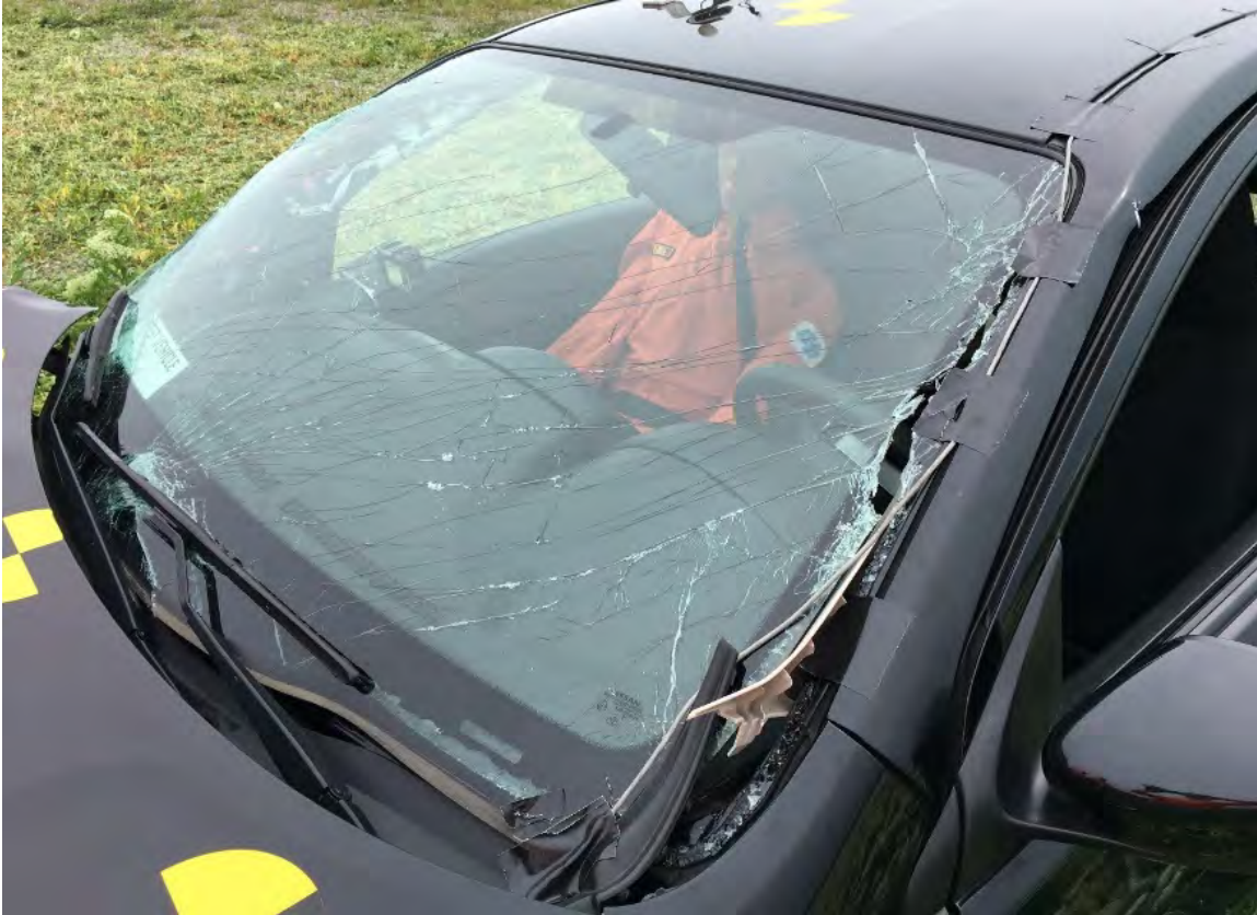
Figure 5-16 Test 4-10 Test Vehicle Windshield Separation
