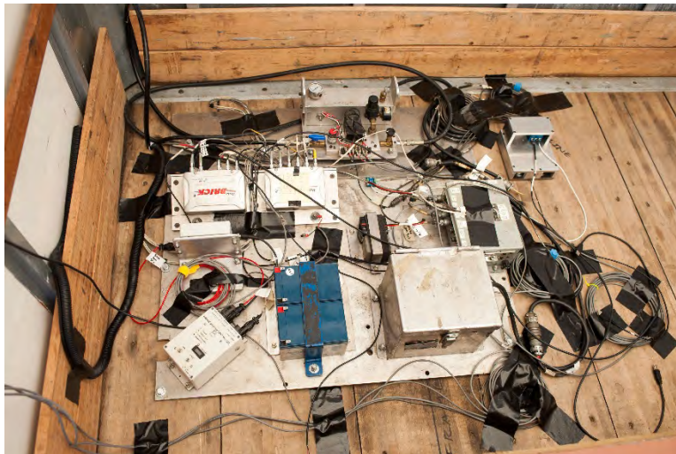
Figure 9-7 Test 4-12 Accelerometers, Angular Rate Sensors, and other Instrumentation in Cargo Box
