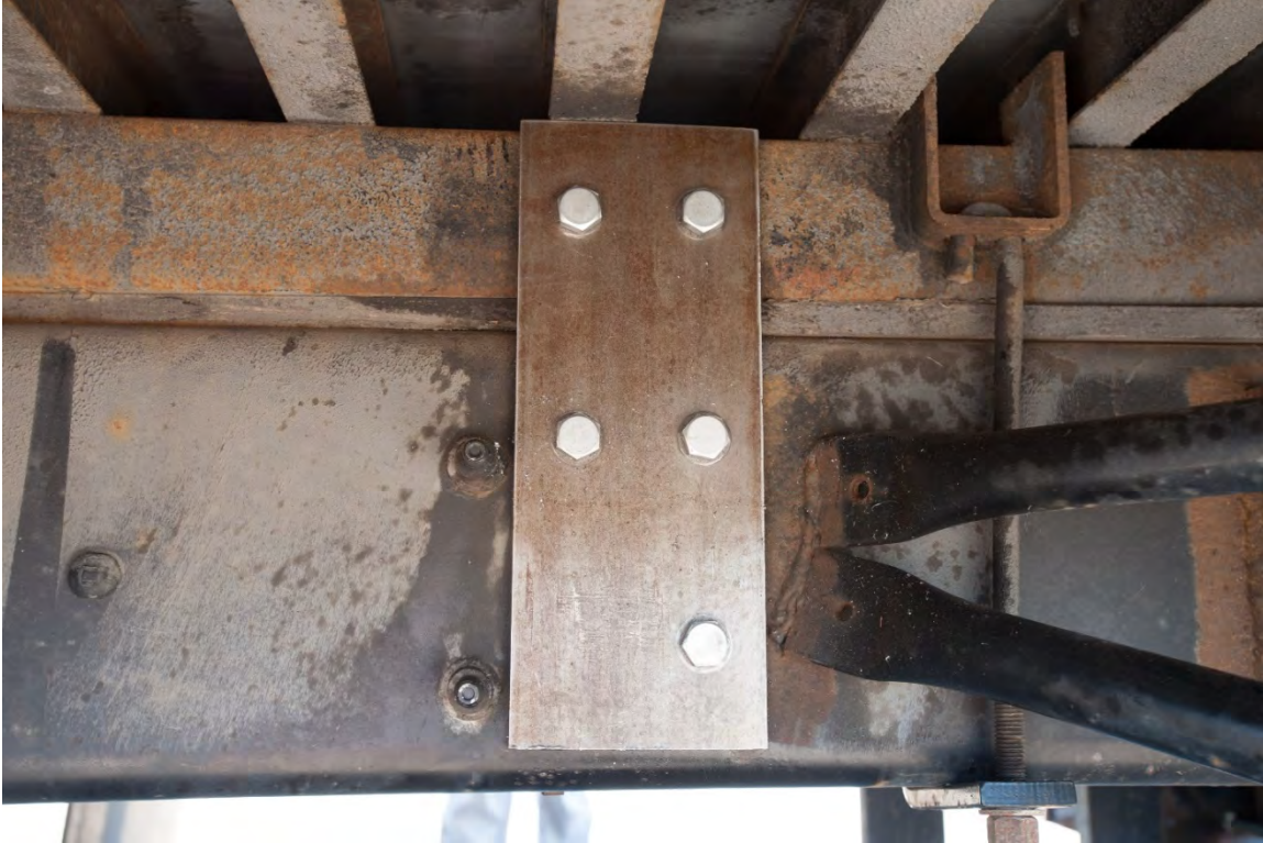
Figure 4-24 MASH 4-12 Test Vehicle Rear Shear Plate
