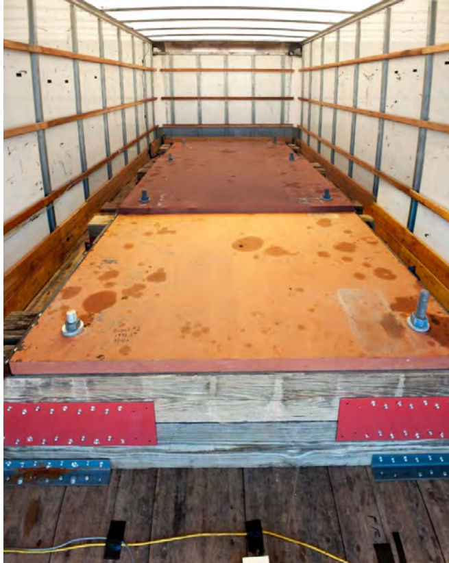
Figure 4-20 MASH 4-12 Test Vehicle Ballast in Cargo Box
