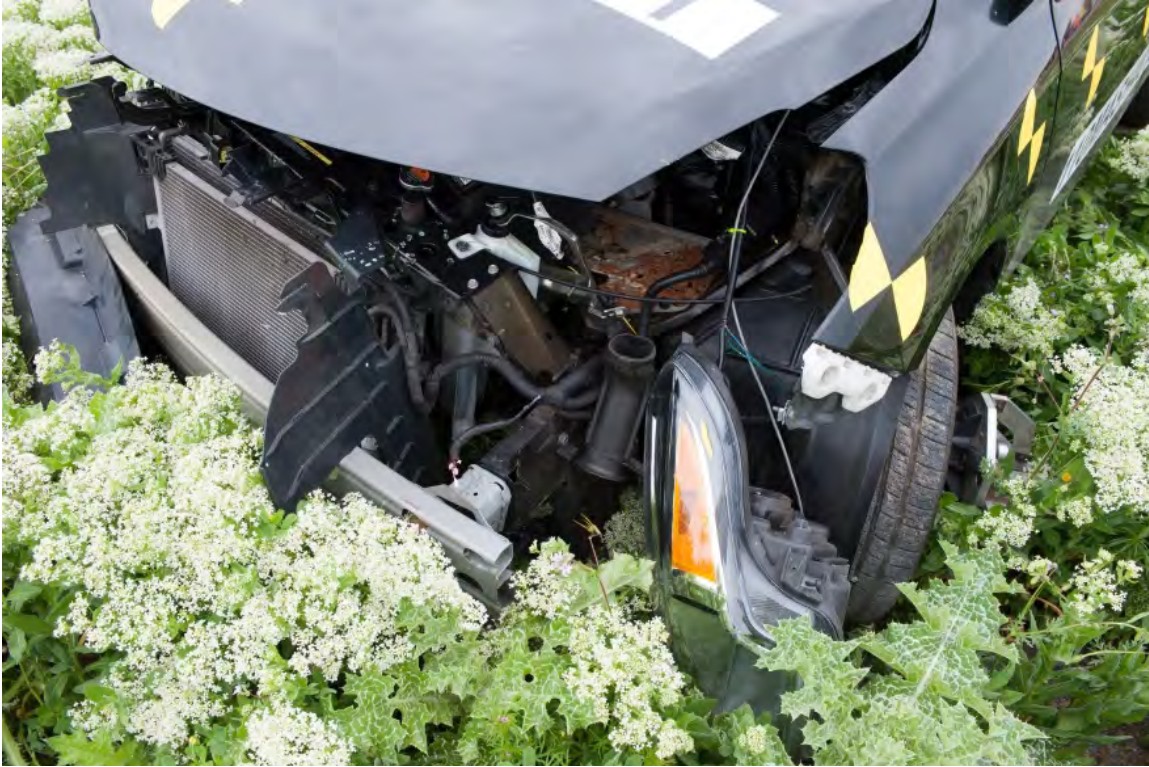
Figure 5-12 Test 4-10 Test Vehicle Damage (Front Left)
