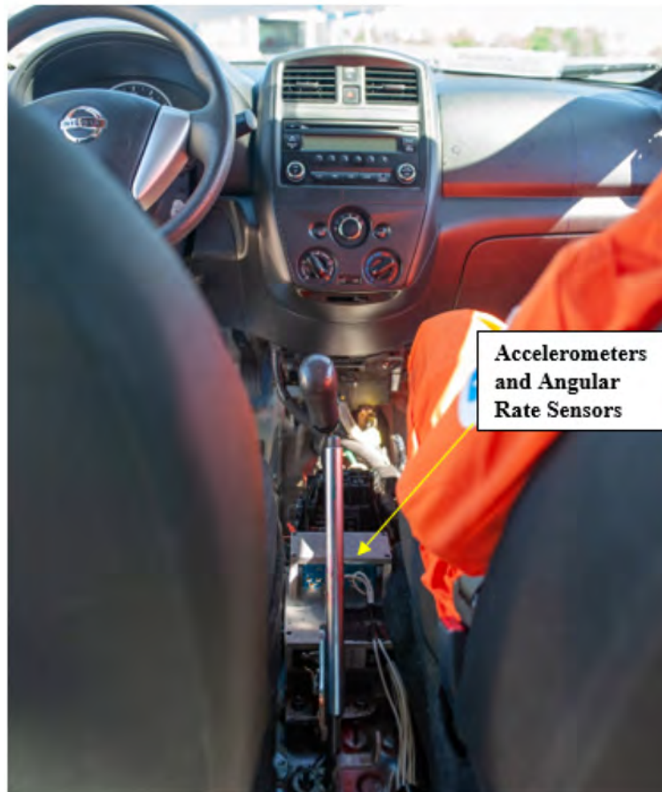
Figure 9-2 Test 4-10 Vehicle Dummy and Instrumentation
