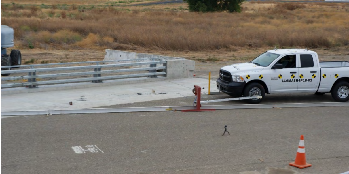
Figure 9-9 Guide Arm Releasing from Test Vehicle
