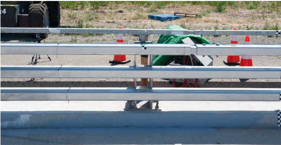
Figure 7-2 Test 4-12 ST-75 Post 5 Downstream of Impact Point Pre-Test
