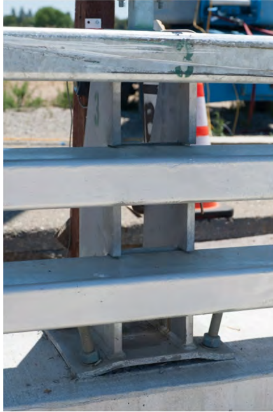
Figure 7-11 Test 4-12 ST-75 Post 3 Post-Test
