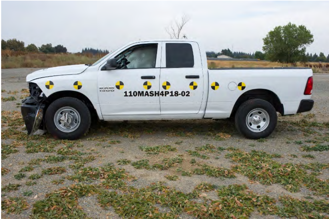
Figure 6-11 Test 4-11 Test Vehicle Damage (Left Side)
