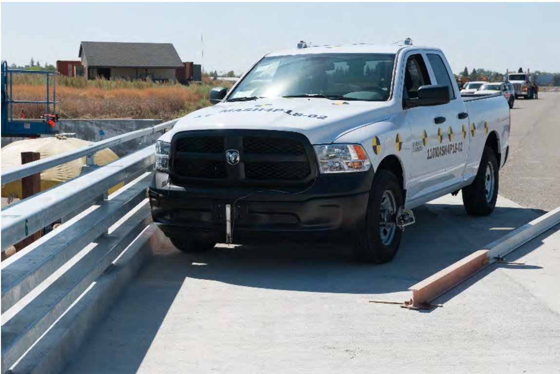
Figure 4-13 MASH 4-11 Test Vehicle at Impact Point
