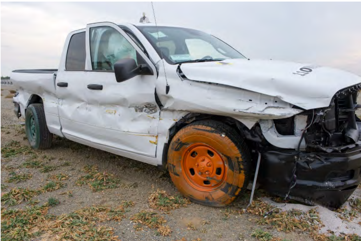
Figure 6-10 Test 4-11 Test Vehicle Damage (Front Right)
