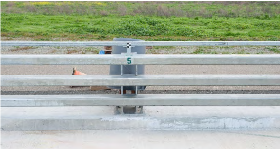
Figure 5-2 Test Article Downstream of Impact Area Pre-Test 4-10
