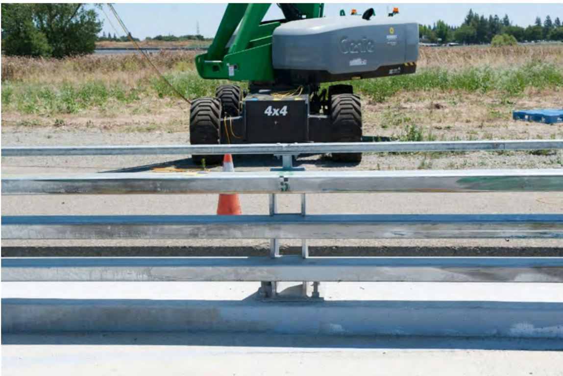
Figure 7-10 Test 4-12 ST-75 Post 5 Downstream of Impact Point Post-Test
