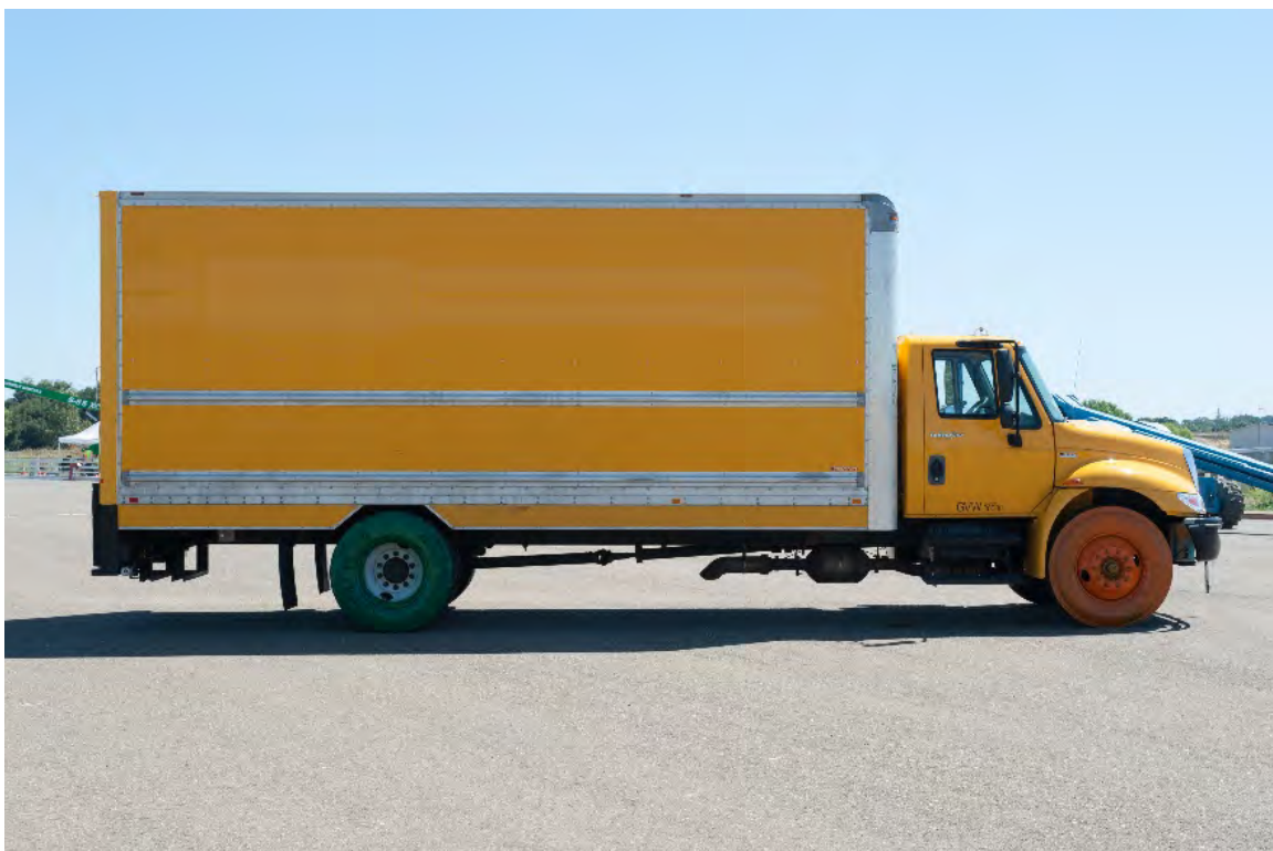
Figure 4-15 MASH 4-12 Test Vehicle Passenger Side
