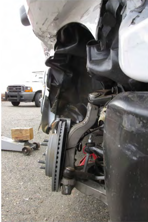
Figure 6-15 Test 4-11 Test Vehicle Front Right Suspension (with wheel removed)
