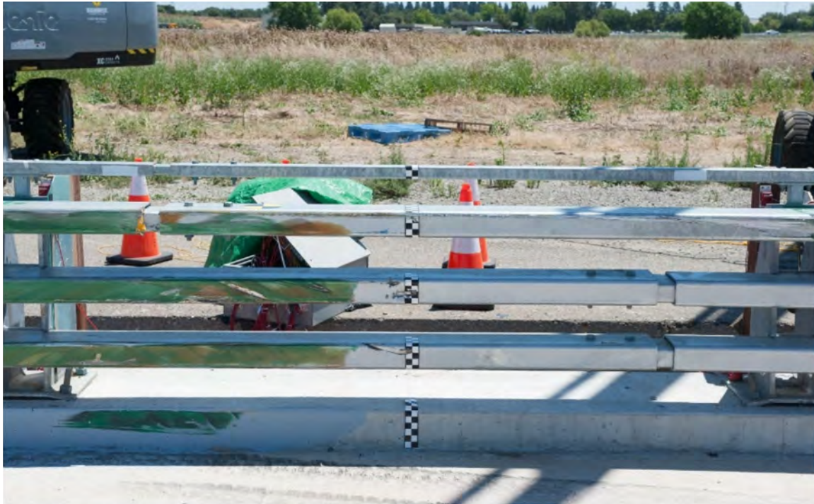
Figure 7-8 Test 4-12 Vehicle Marks on ST-75 Impact Point Between Posts 3 and 4 Post-Test
