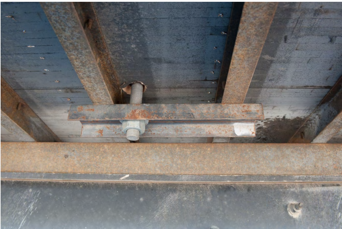
Figure 4-23 MASH 4-12 Test Vehicle Ballast Mounting Plate
