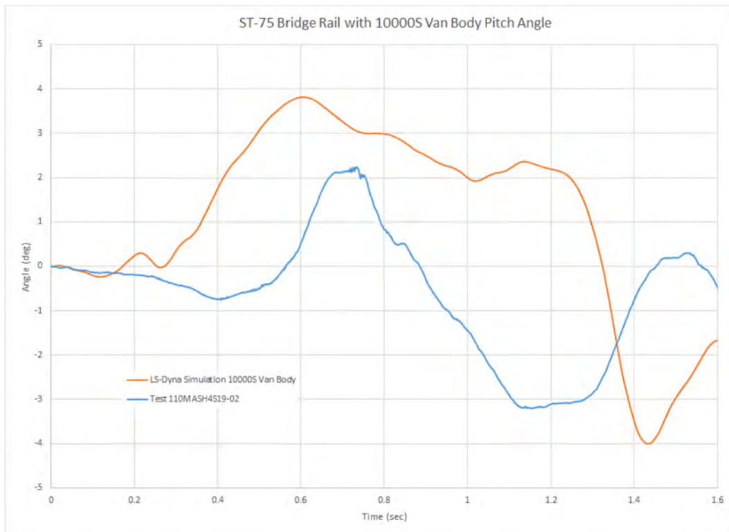
Figure 14-33 Graph of Pitch Angles for Full Scale and FE Model TRAP Results for 10000S Single Unit Truck
