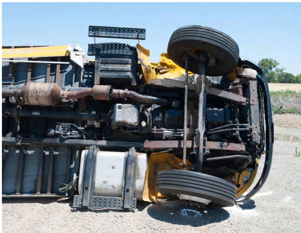
Figure 7-17 MASH 4-12 Test Vehicle Front Undercarriage and Suspension After Impact
