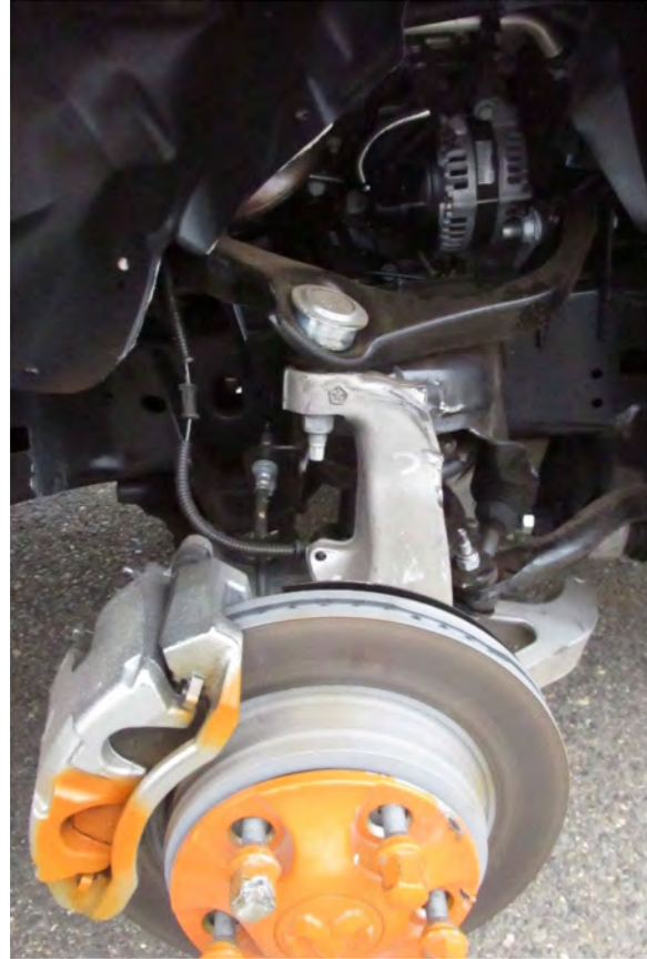
Figure 6-15 Test 4-11 Test Vehicle Front Right Suspension (with wheel removed)
