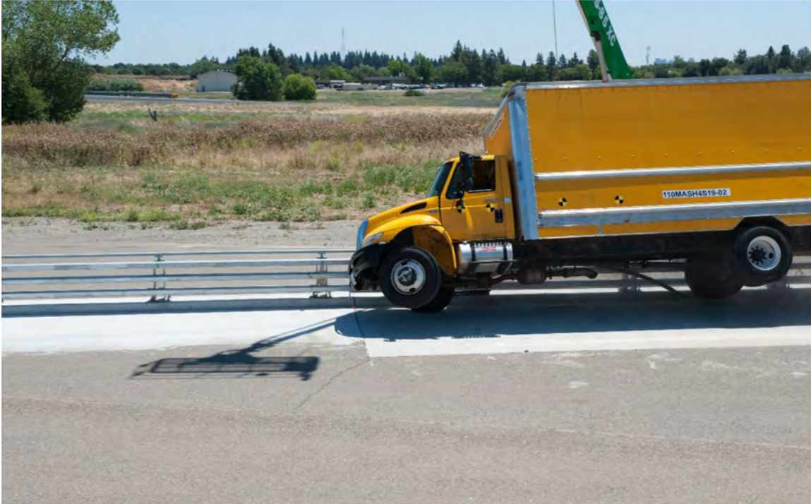
Figure 7-5 Test 4-12 Across Camera Impact View
