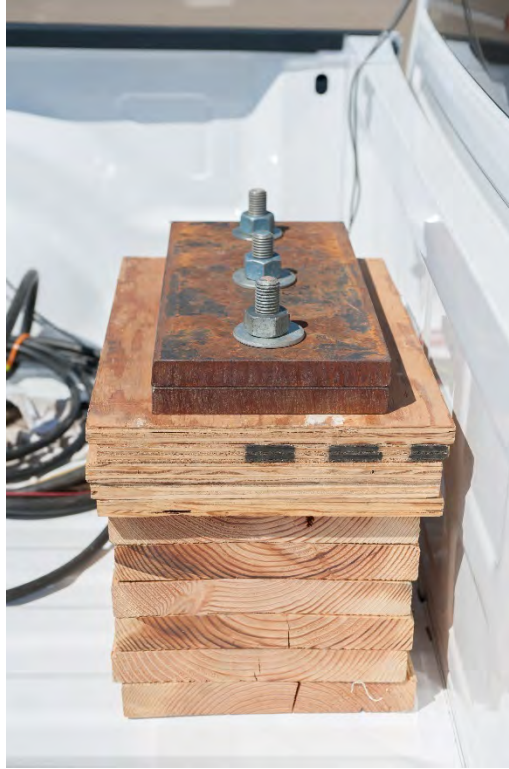
Figure 4-12 MASH 4-11 Test Vehicle Ballast
