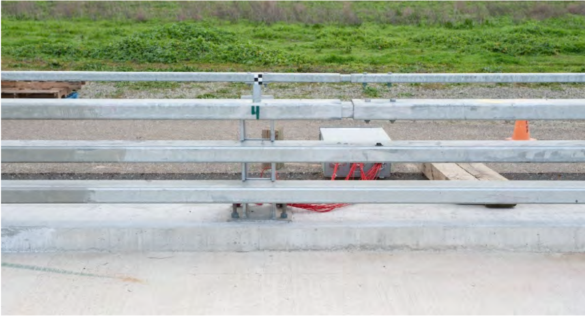
Figure 5-1 Test Article Impact Area Pre-Test 4-10
