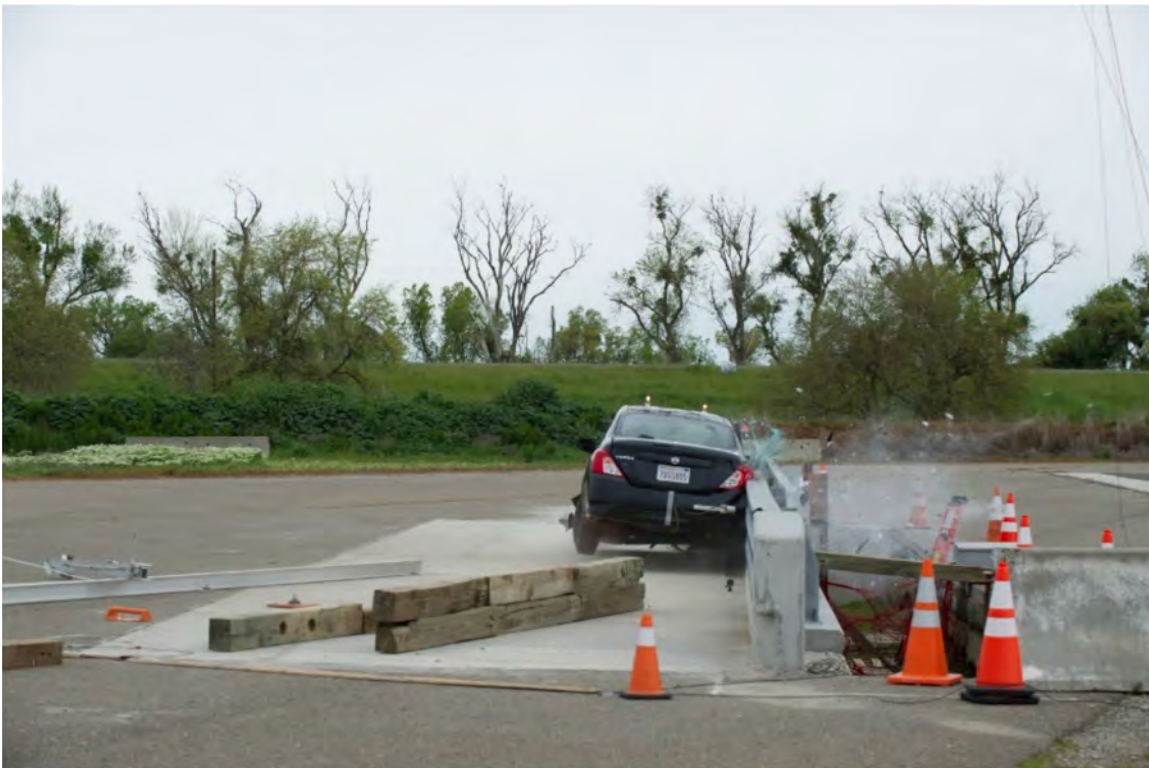
Figure 5-4 Test 4-10 Upstream Camera Impact View
