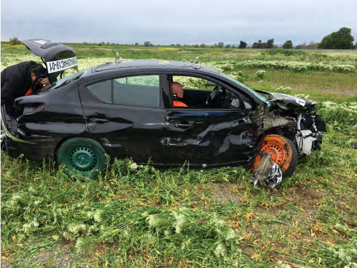
Figure 5-10 Test 4-10 Test Vehicle Damage (Right Side)
