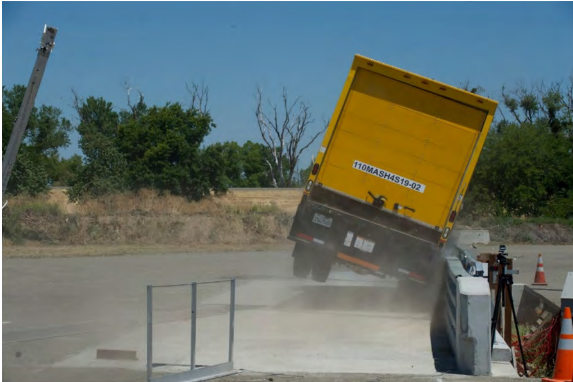
Figure 7-7 Test 4-12 Upstream Camera Impact View
