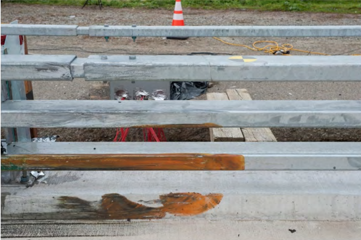
Figure 5-7 Test 4-10 Vehicle Marks on ST-75 Impact Point Post-Test
