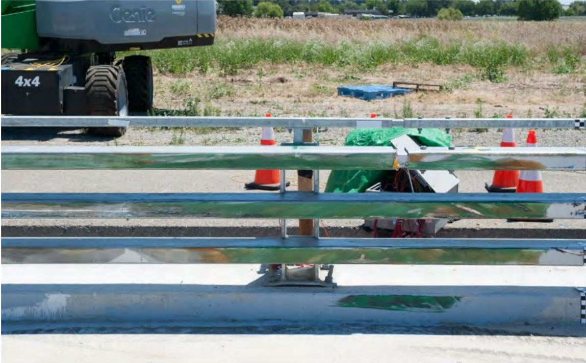
Figure 7-9 Test 4-12 Vehicle Marks on ST-75 at Post 4 Downstream of Impact Point Post-Test
