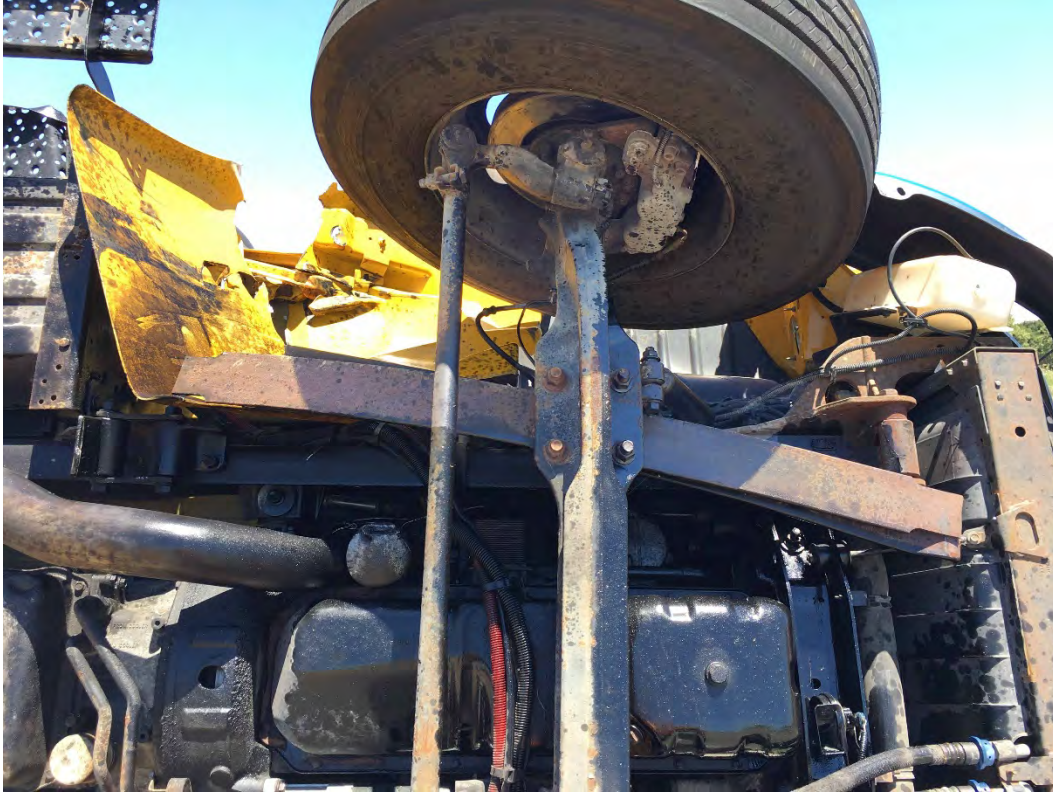
Figure 7-18 MASH 4-12 Test Vehicle Undercarriage and Suspension After Impact
