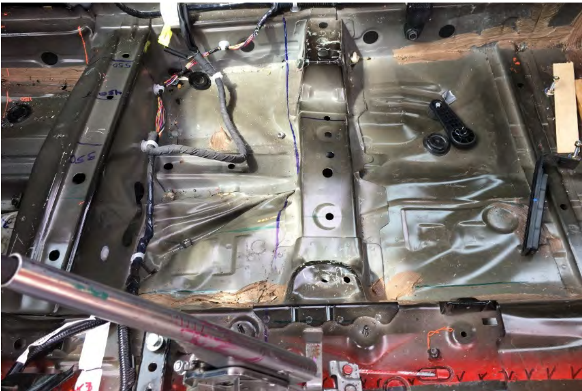
Figure 5-15 Test 4-10 Test Vehicle Occupant Compartment Deformation (Front Seat Area)
