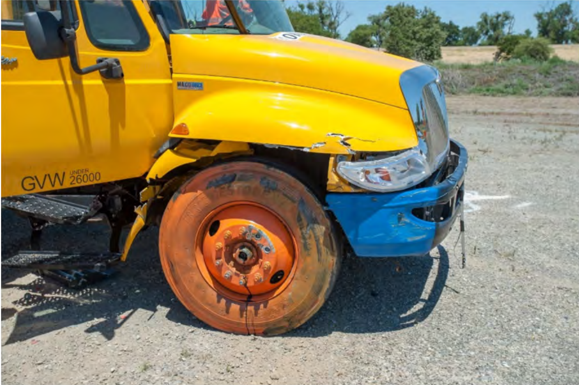
Figure 7-20 Test 4-12 Test Vehicle (Front Right) Post-Test (righted)
