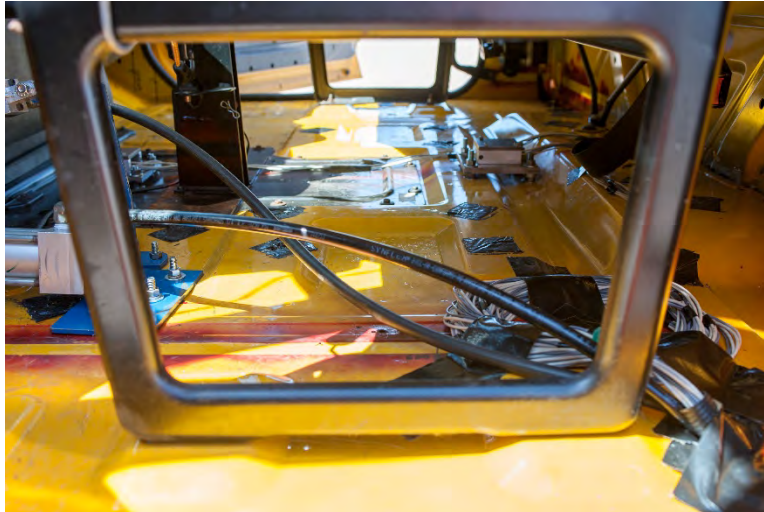
Figure 9-6 Test 4-12 Accelerometers and Angular Rate Sensors in Cab
