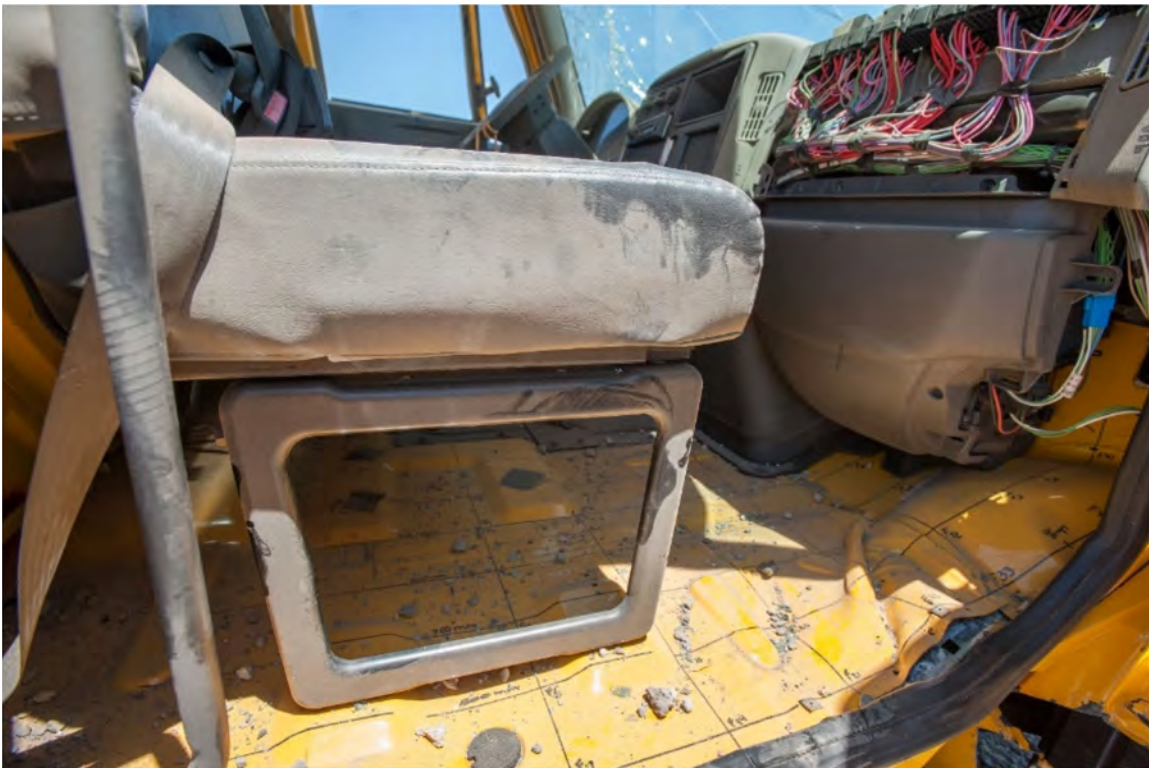
Figure 7-27 Test 4-12 Test Vehicle Occupant Compartment Deformation Post-Test
