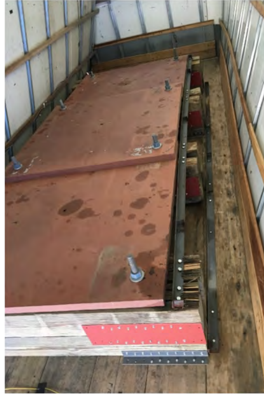
Figure 7-16 MASH 4-12 Test Vehicle Ballast After Impact
