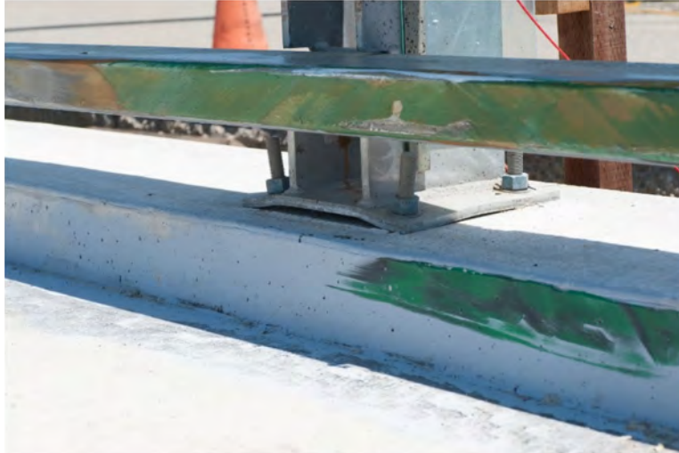
Figure 7-13 Test 4-12 Post 4 Bent Bottom Plate Close Up Post-Test
