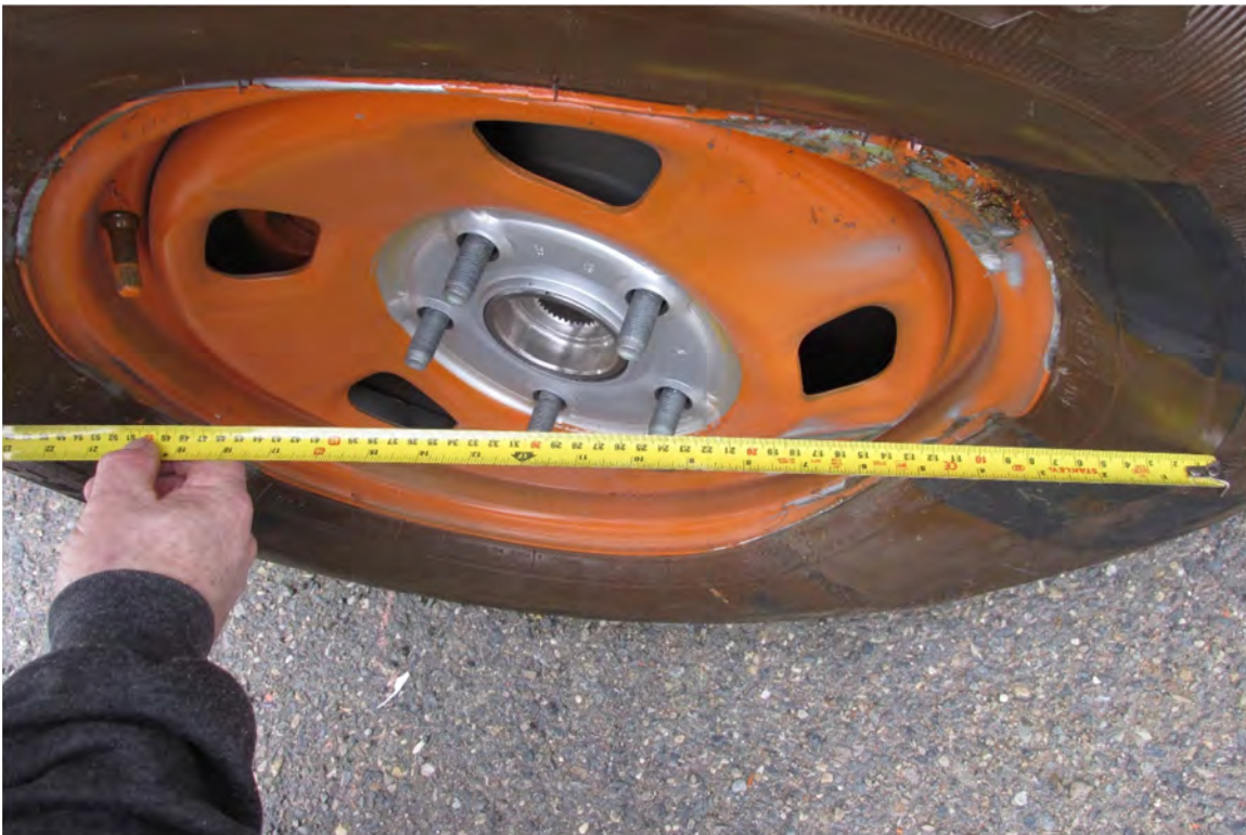
Figure 6-14 Test 4-11 Test Vehicle Front Right Wheel Deformation
