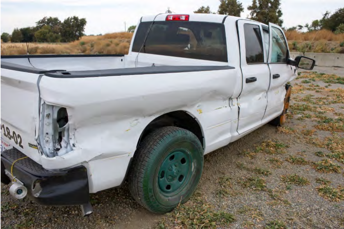
Figure 6-9 Test 4-11 Test Vehicle Damage (Rear Right)
