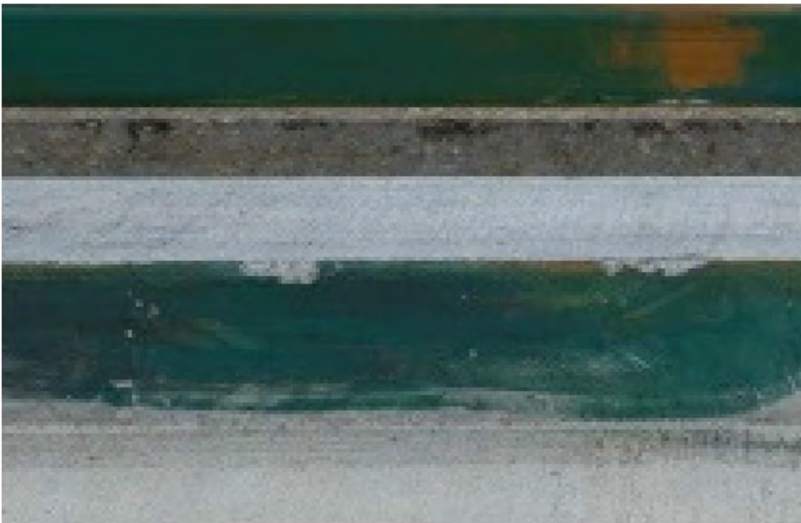
Figure 6-7 Test 4-11 Minor Concrete Spalling of Concrete Curb Post-Test
