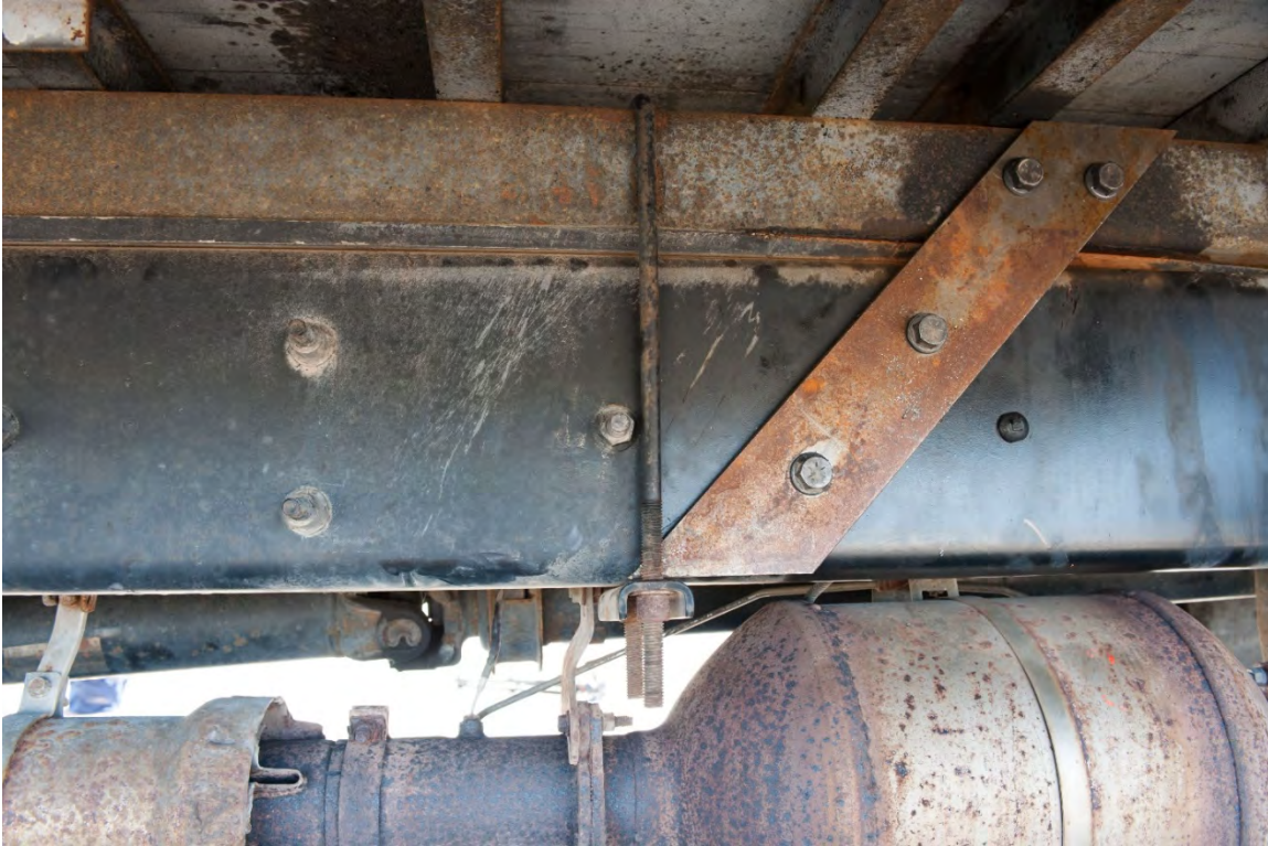
Figure 4-22 MASH 4-12 Test Vehicle Front Shear Plate
