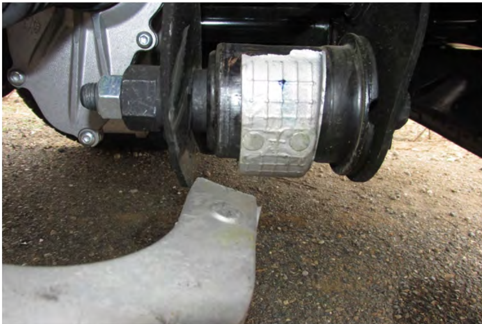
Figure 6-16 Test 4-11 Test Vehicle Front Right Suspension Lower Control Arm Connector Fracture
