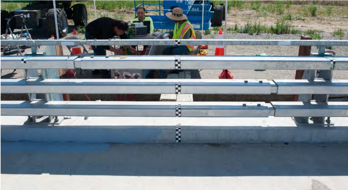
Figure 7-1 Test 4-12 ST-75 Impact Area with Checkered Tape at Impact Point Pre-Test
