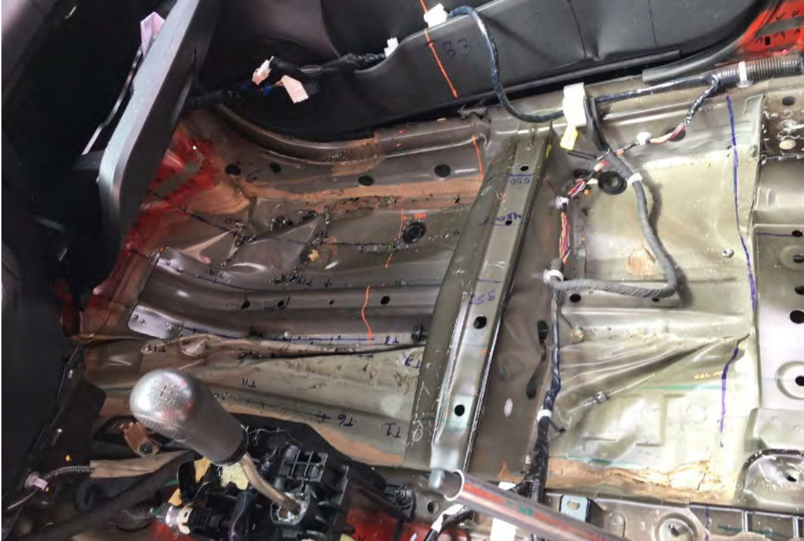
Figure 5-14 Test 4-10 Test Vehicle Occupant Compartment Floorboard Deformation
