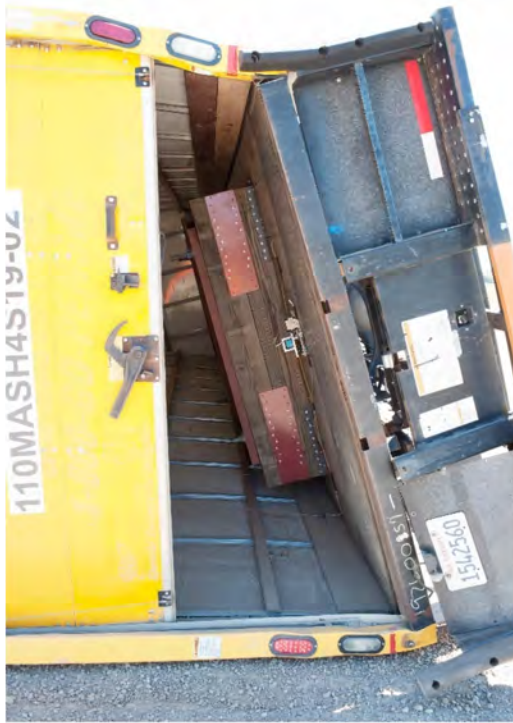
Figure 7-16 MASH 4-12 Test Vehicle Ballast After Impact
