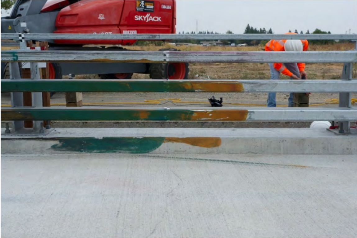
Figure 6-6 Test 4-11 Vehicle Marks on ST-75 at Impact Point Post-Test
