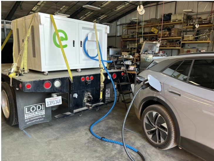
Figure 4.18: Volkswagen ID.4 being charged by the EVES-6060-NA
