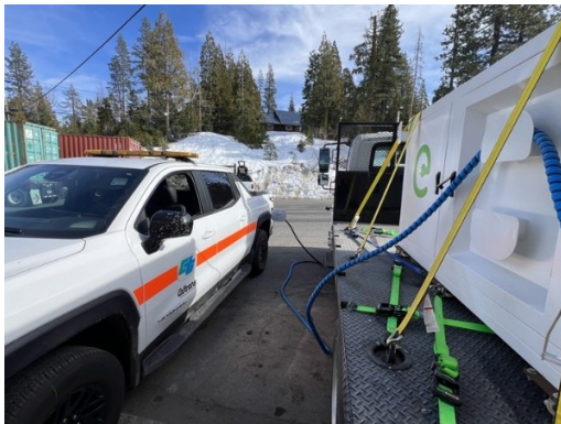
Figure 4.6: Chevrolet Silverado EV being charged by the EVES-6060-NA
