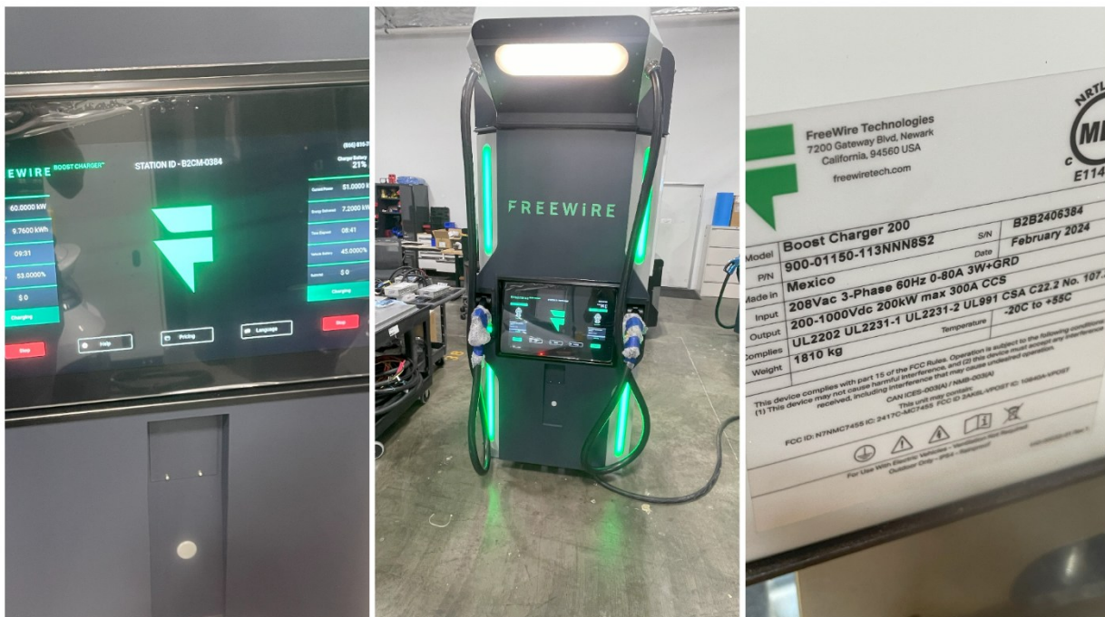
Figure 5.43: FreeWire Boost Charger 200 replacement unit commissioning process at SpeedCharge HQ: operational interface (left), unit in testing facility (middle), technical specifications (right)
