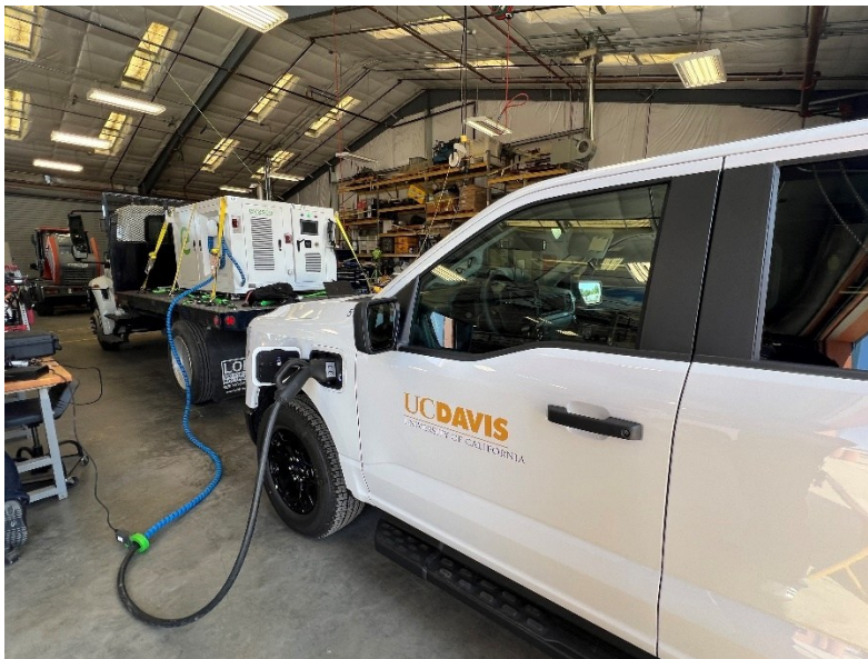
Figure 4.8: Ford F150 Lightning being charged by the EVES-6060-NA
