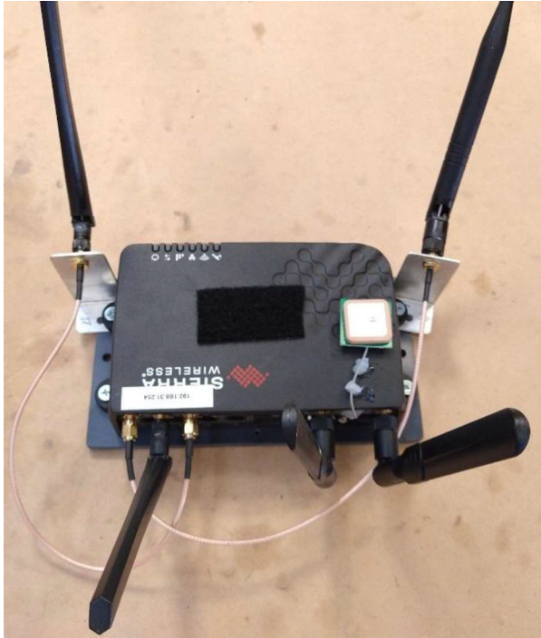
Figure 2.1: Sierra Wireless MP70 modem with Wi-Fi
