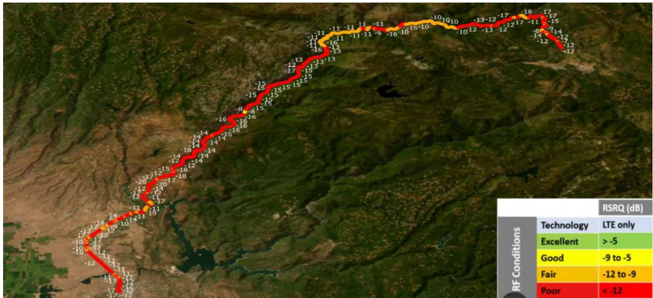
Figure 3.14: Trial 3 – Verizon RSRQ mapping result along Highway 70. Map generated using ArcGIS software by Esri.
