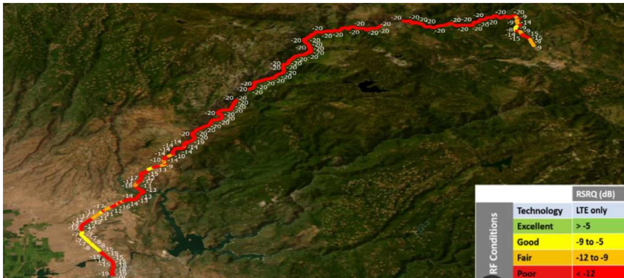
Figure 3.6: Trial 3 – AT&T RSRQ mapping result along Highway 70. Map generated using ArcGIS software by Esri.
