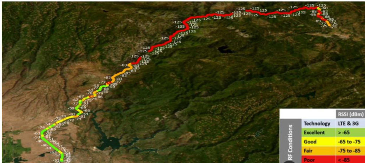
Figure 3.5: Trial 3 – AT&T RSSI mapping result along Highway 70. Map generated using ArcGIS software by Esri.
