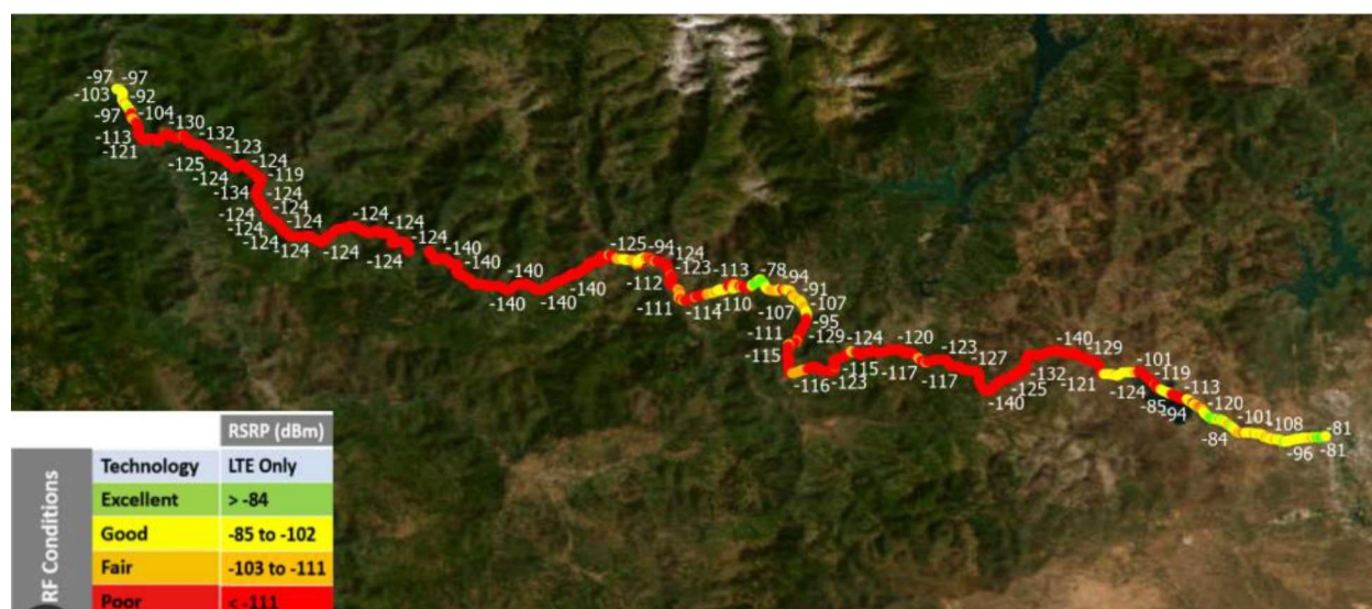
Figure 3.3: Trial 3 – AT&T RSRP mapping result along Highway 299. Map generated using ArcGIS software by Esri.
