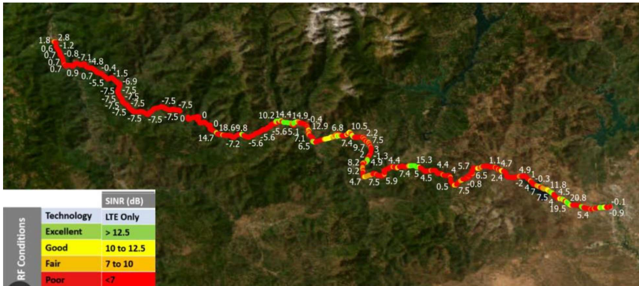
Figure 3.12: Trial 3 – Verizon SINR mapping result along Highway 299. Map generated using ArcGIS software by Esri.
