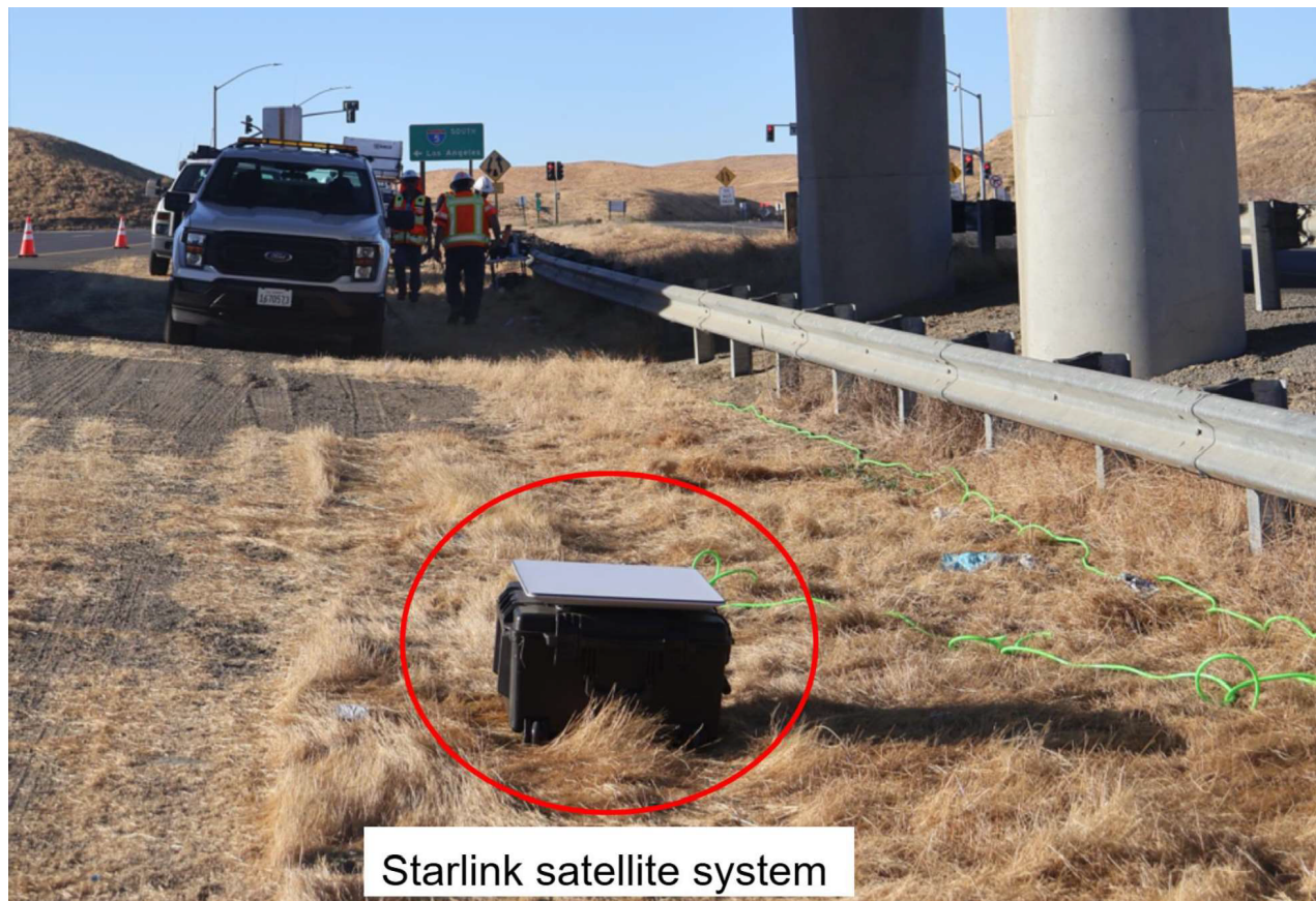
Figure 2.6: The Starlink satellite system set-up for AHMCT Task 4059 - Caltrans project. As long as the system is powered, it can serve as a hotspot for multiple devices.
