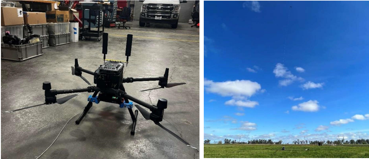
Figure 3.6: First-generation payload package mounted onto the DJI M300 and system testing conducted during the April 2024 testing session.
