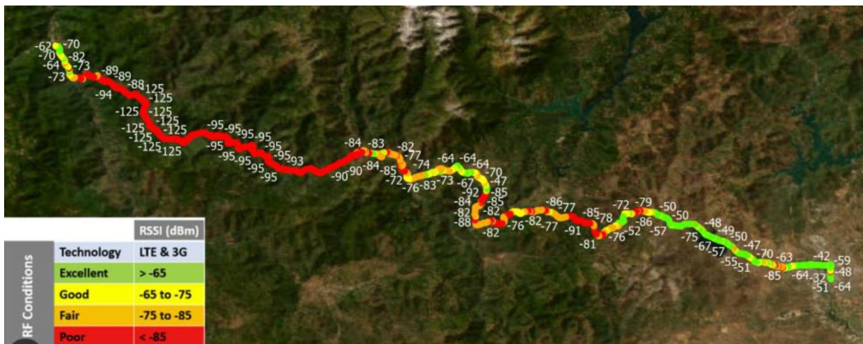
Figure A.9: Trial 1 – Verizon RSSI mapping result along Highway 299. Map generated using ArcGIS software by Esri.
