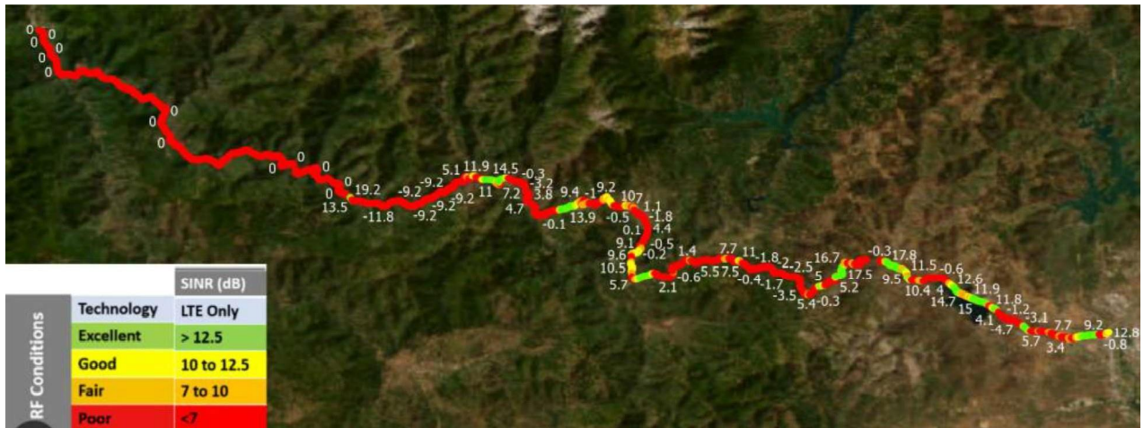
Figure A.16: Trial 2 – Verizon SINR mapping result along Highway 299. Map generated using ArcGIS software by Esri.
