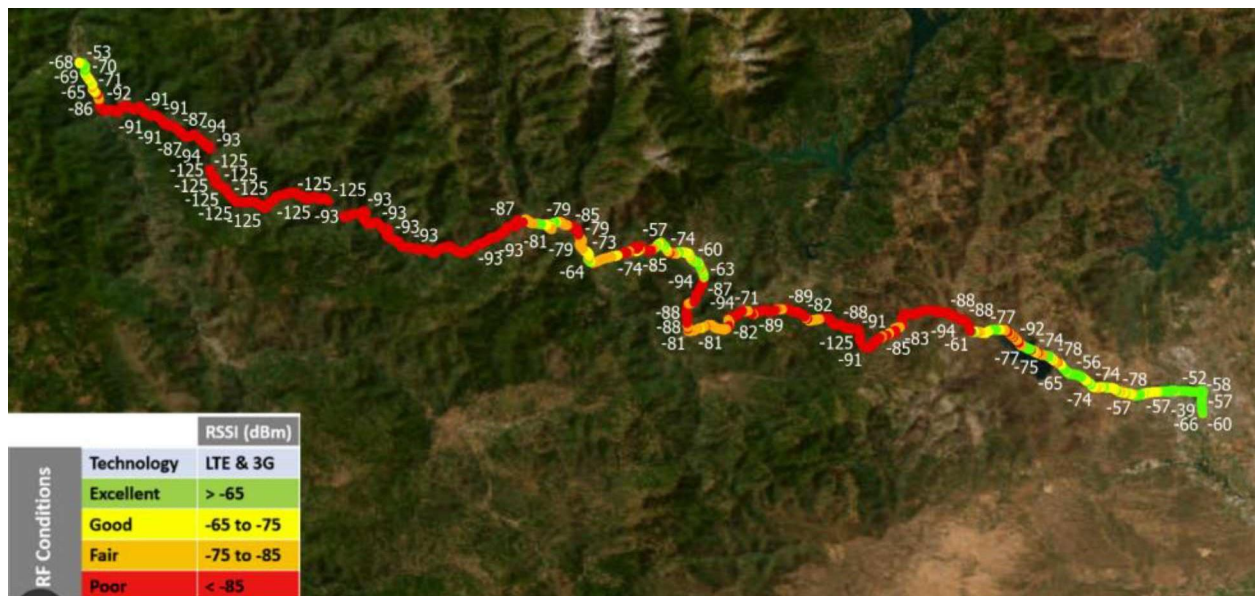
Figure A.1: Trial 1 – AT&T RSSI mapping result along Highway 299. Map generated using ArcGIS software by Esri.
