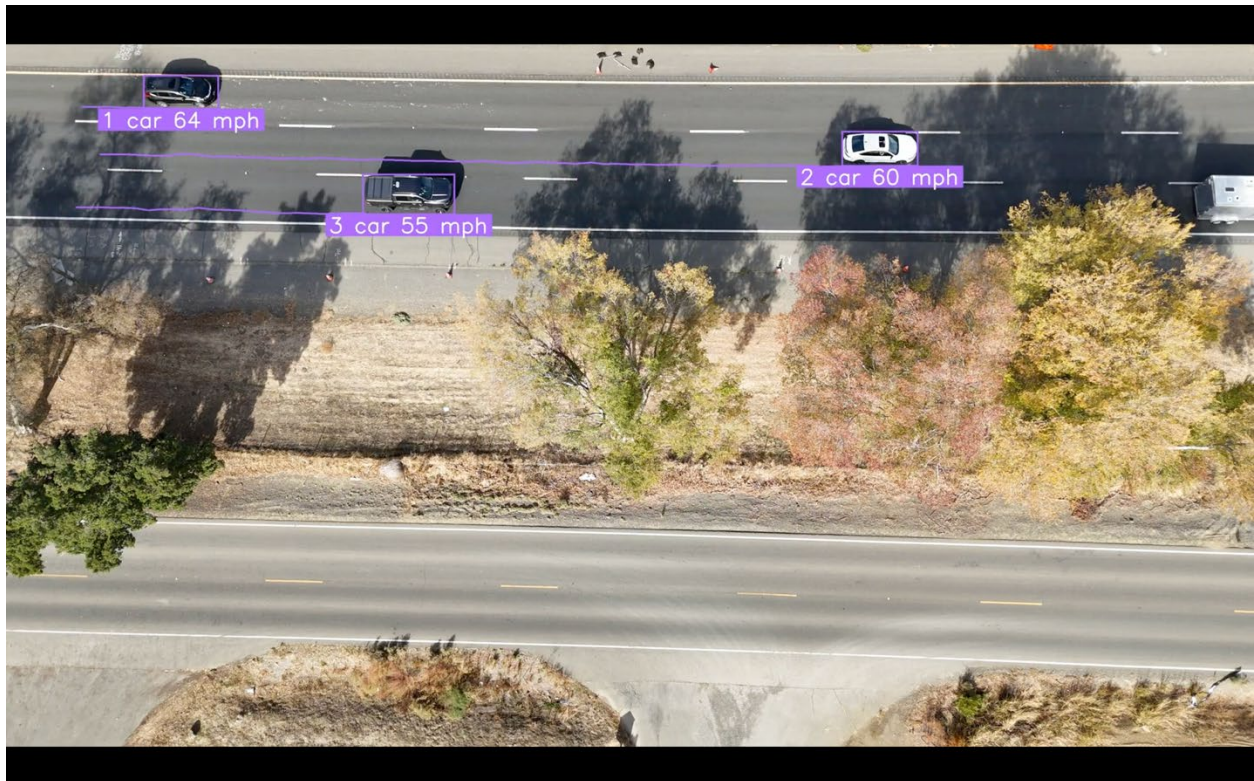
Fig.1. A floating car in the second lane with the speed of 64 mph is tracked along with its speed, lane, and classification as a passenger vehicle.
