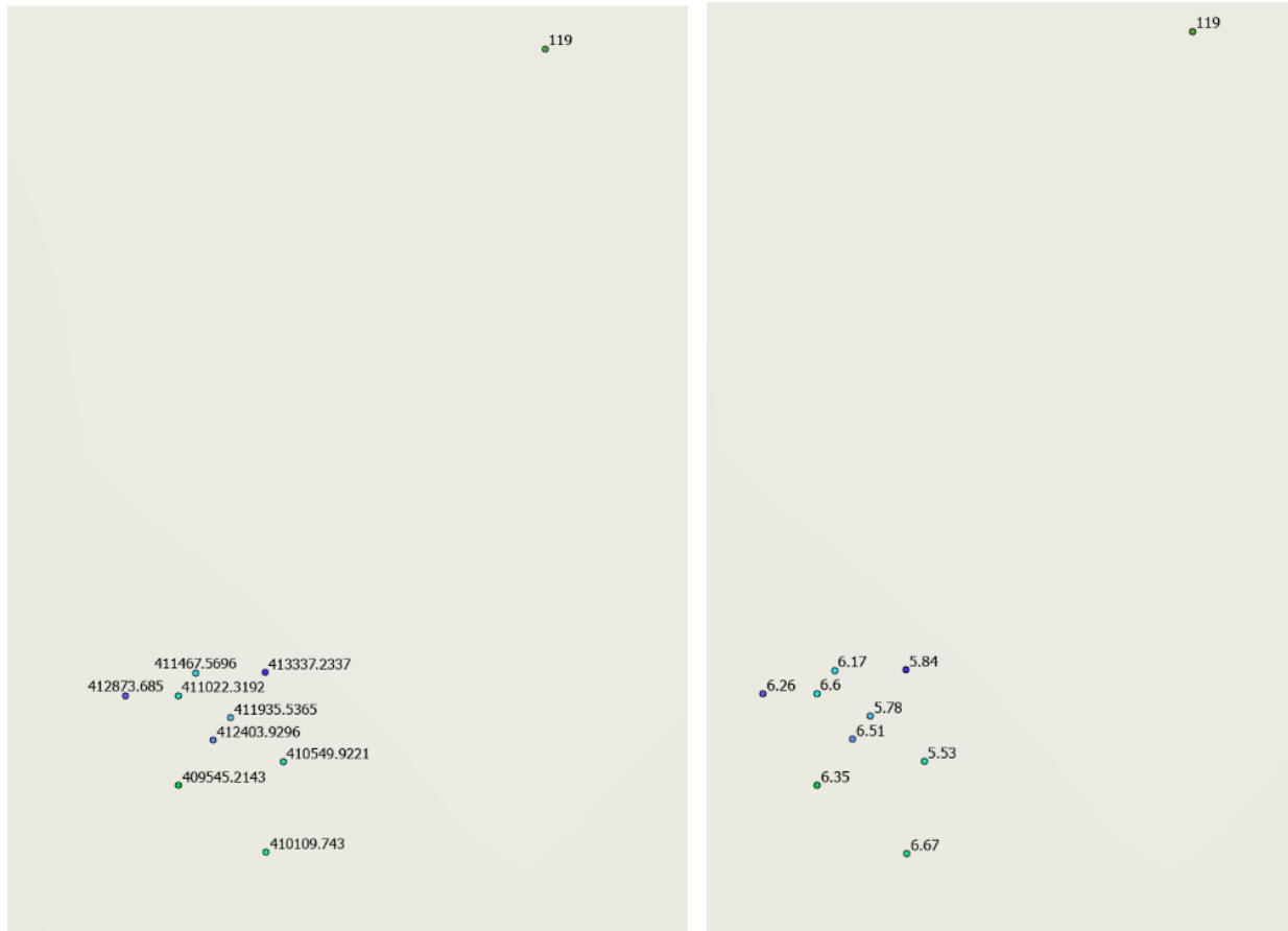
Figure 3.8: Vehicle trajectory points for each MTL record run closest to GCP number 119 plotted on ArcGIS Pro. The points were labeled with the point's GPS time (in seconds) in the left image. The points were labeled with time elapsed from previous GCP (in seconds) in the right image.
