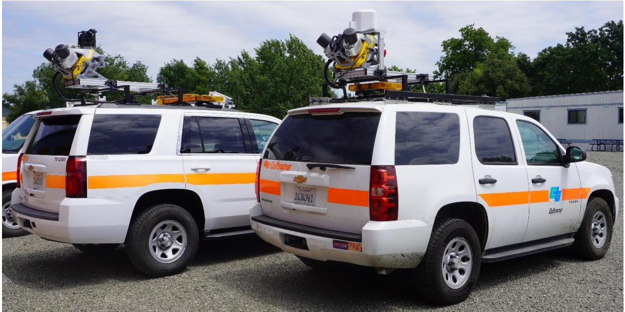
Figure 2.7: Examples of MX9 installation on Caltrans vehicles.
