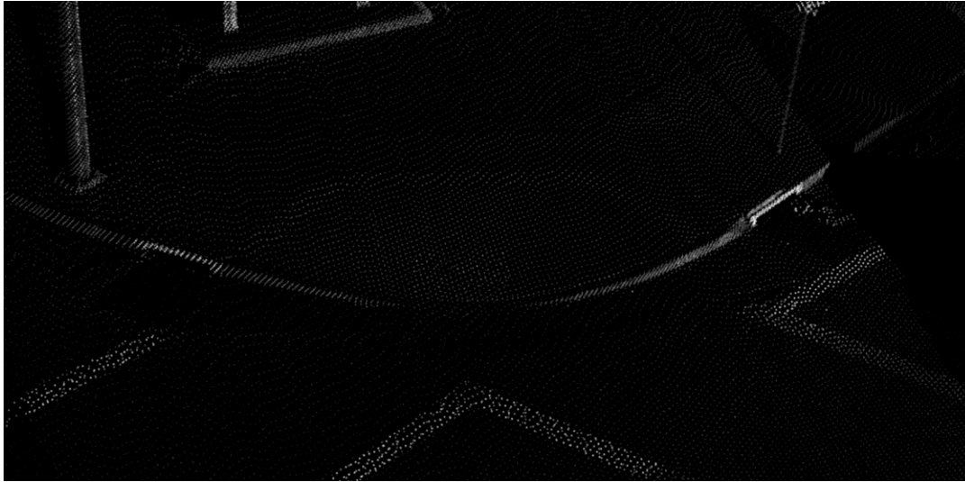
Figure 6.9: Point cloud of an ADA ramp located on the opposite travel direction side of the ADA ramp shown in Figure 6.8 collected in the same scan session by an MX50 system.
