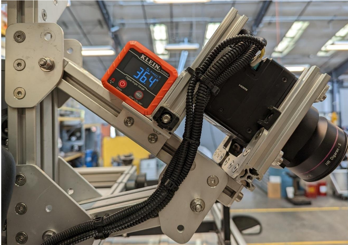
Figure 5.10: GS120 Camera with a 10 Gb Ethernet fiber optic cable installed.
