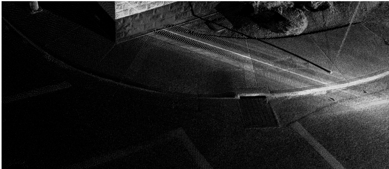
Figure 6.7: Intensity-based rendering of the same ADA ramp shown in Figure 6.5. The DWS reflectivity is very close to the surrounding concrete surface.
