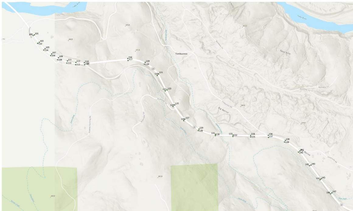
Figure 3.2: Test site topography map overlaid with GCP locations and GCP number using ArcGIS Pro software. Background topographic map image courtesy of ArcGIS Pro, ESRI.
