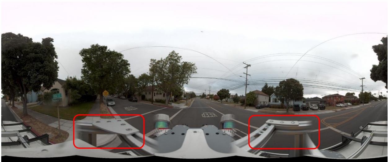
Figure 2.5: Example panorama image from the 360-degree camera from version 1 of the camera cap mount. The red rectangles highlight the areas of the frame supports blocking the 360-camera field-of-view (FOV).
