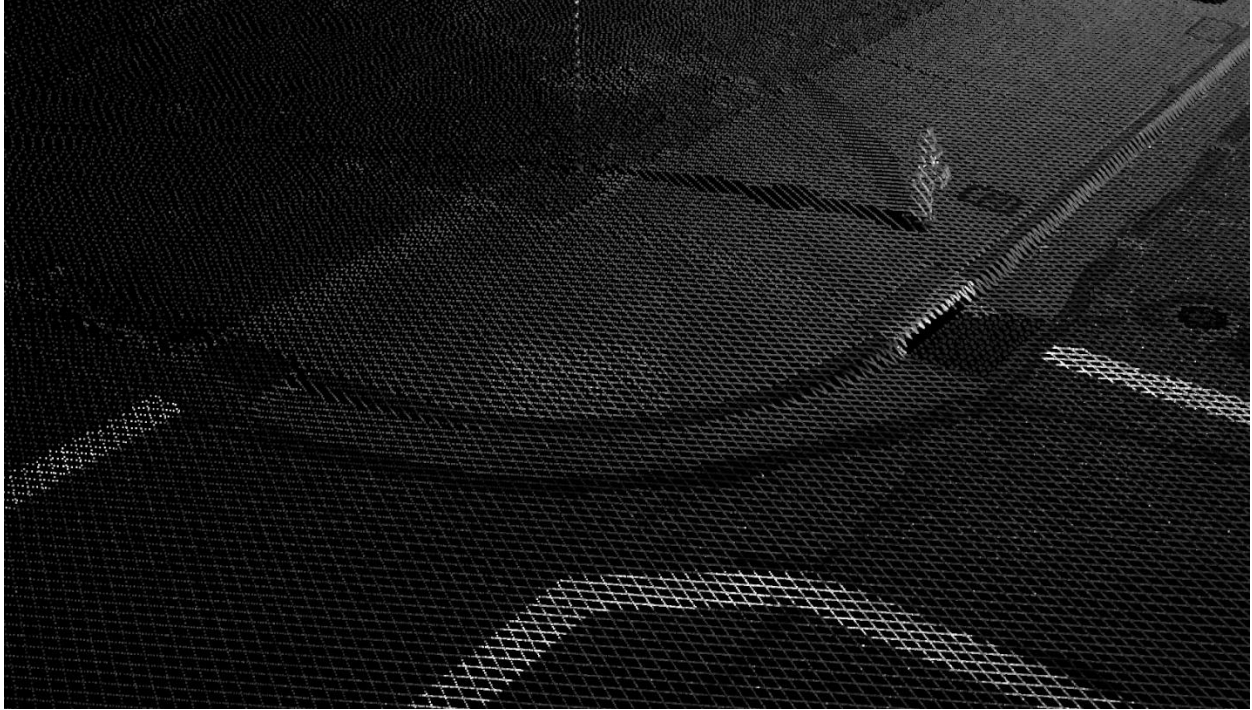
Figure 6.8: Example ADA ramp point cloud (intensity-based rendered, left and right lasers) collected from an MX50 system. The ADA ramp is located at Alturas California near the ADA ramp shown in Figures 6.6 and 6.7. In this case, the DWS and surrounding concrete surface reflectivity difference is larger.
