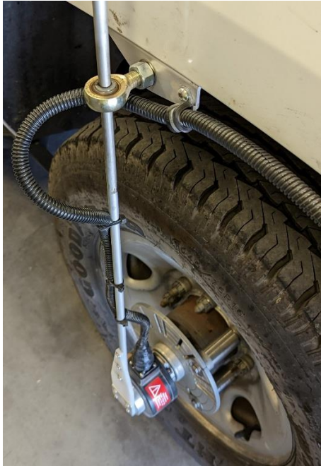
Figure 2.12: MX50 DMI rod support installation.
