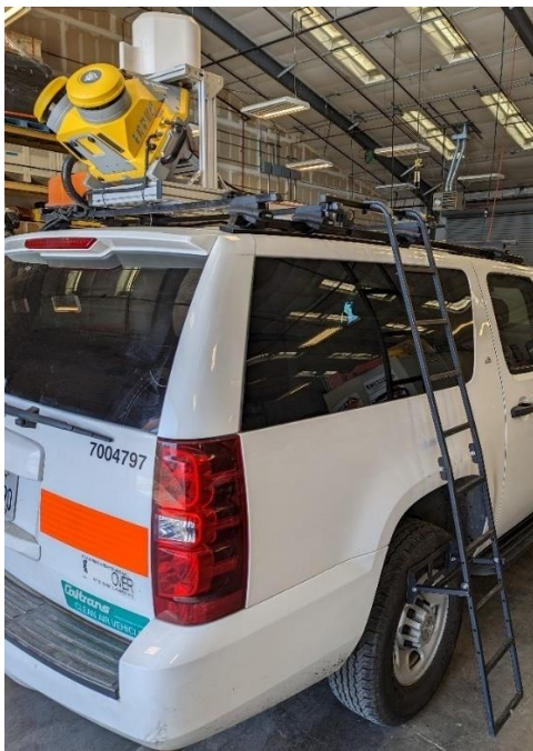
Figure 2.8: Caltrans MX50 installation with a custom side folding ladder.
