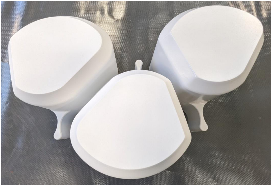
Figure 2.3: Completed 360-degree camera caps. White protective paint was applied.
