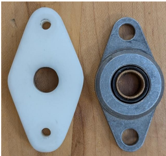
Figure 2.11: District 3's MX9 DMI rod brushings.
