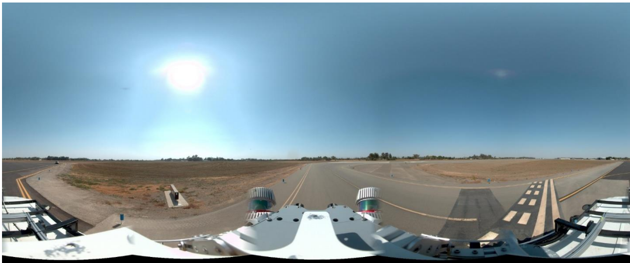
Figure 2.6: Example panorama image from the 360-degree camera from Version 2 camera cap mount. The Version 2 cap support reduces FOV blockage on both the sides of the vehicle.
