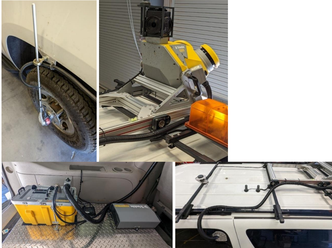
Figure 2.9: Caltrans MX50 installation on a Suburban. MX8 system was previously installed on the vehicle.
