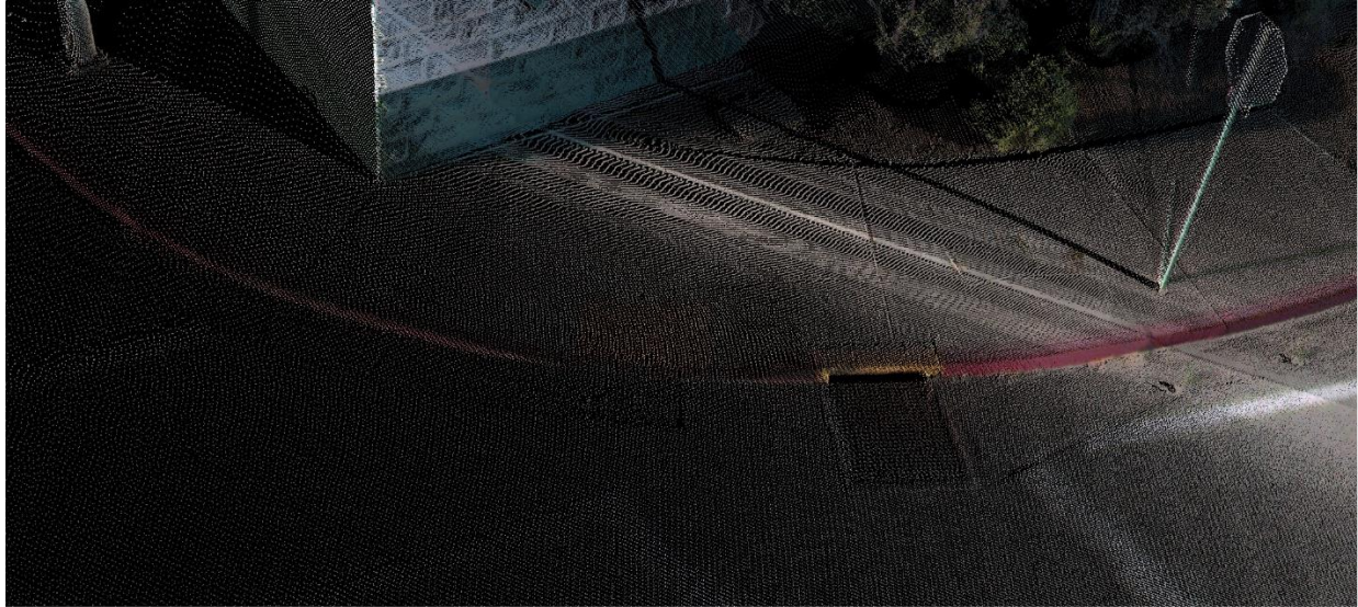
Figure 6.6: Example ADA ramp (Case A) colorized point cloud from the MX50's left and right lasers. The ADA ramp is located at Alturas, California. The yellow DWS can be seen in the colorized point cloud.
