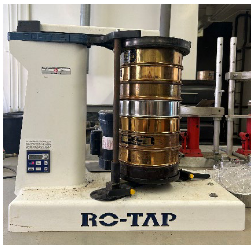
Figure 10. Sieve analysis of sweeping materials
