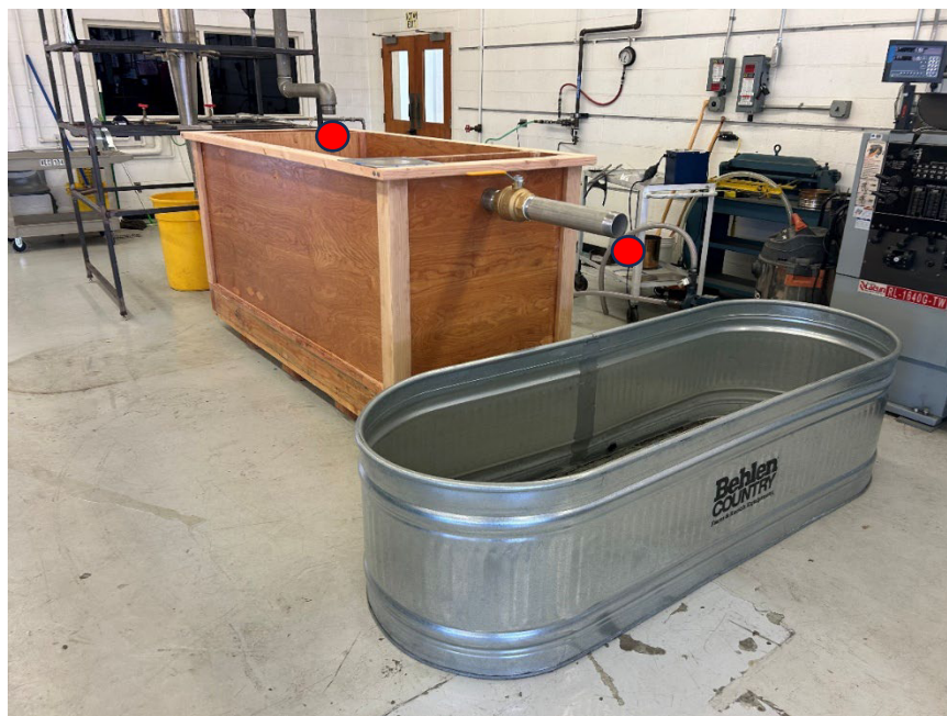
Figure 30. 12 gpm settling compartment testing system. Red indicating sampling locations
