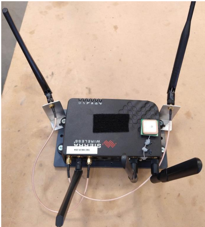
Figure 2.4: Sierra Wireless MP70 with LTE, GNSS, and 5 dB gain Wi-Fi antennas mounted on the UAS mounting plate
