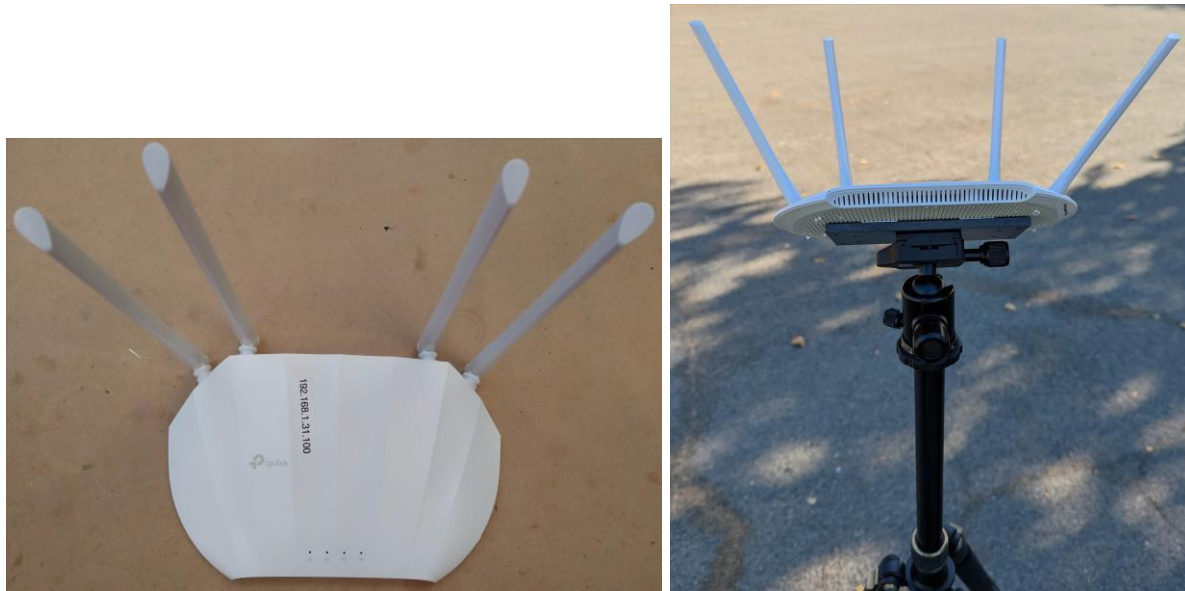
Figure 2.9: TP-Link AC1200 Wi-Fi repeater mounted on a tripod
