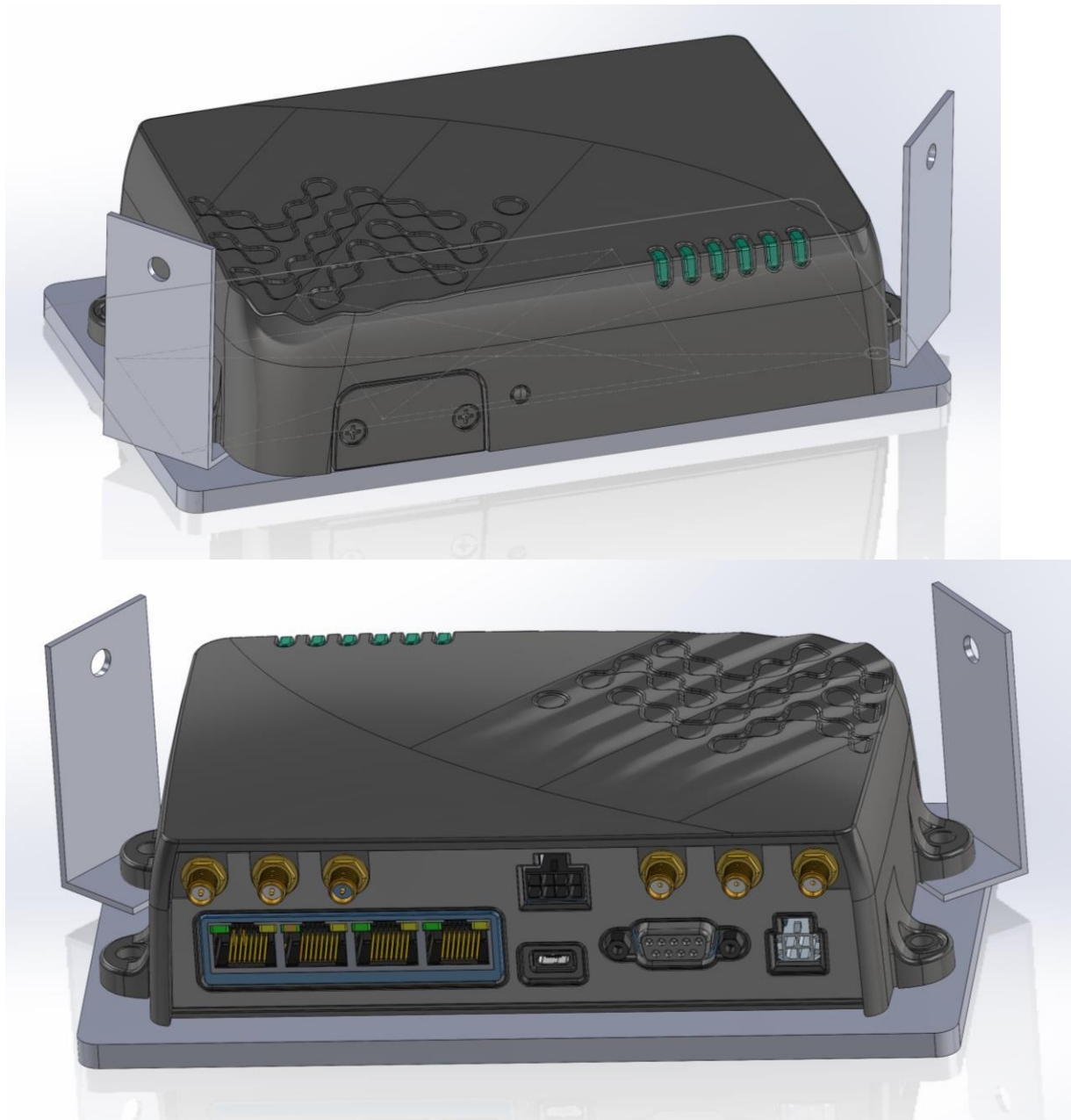
Figure A.2: UAS Repeater Computer-Aided Design 3D model rendering
