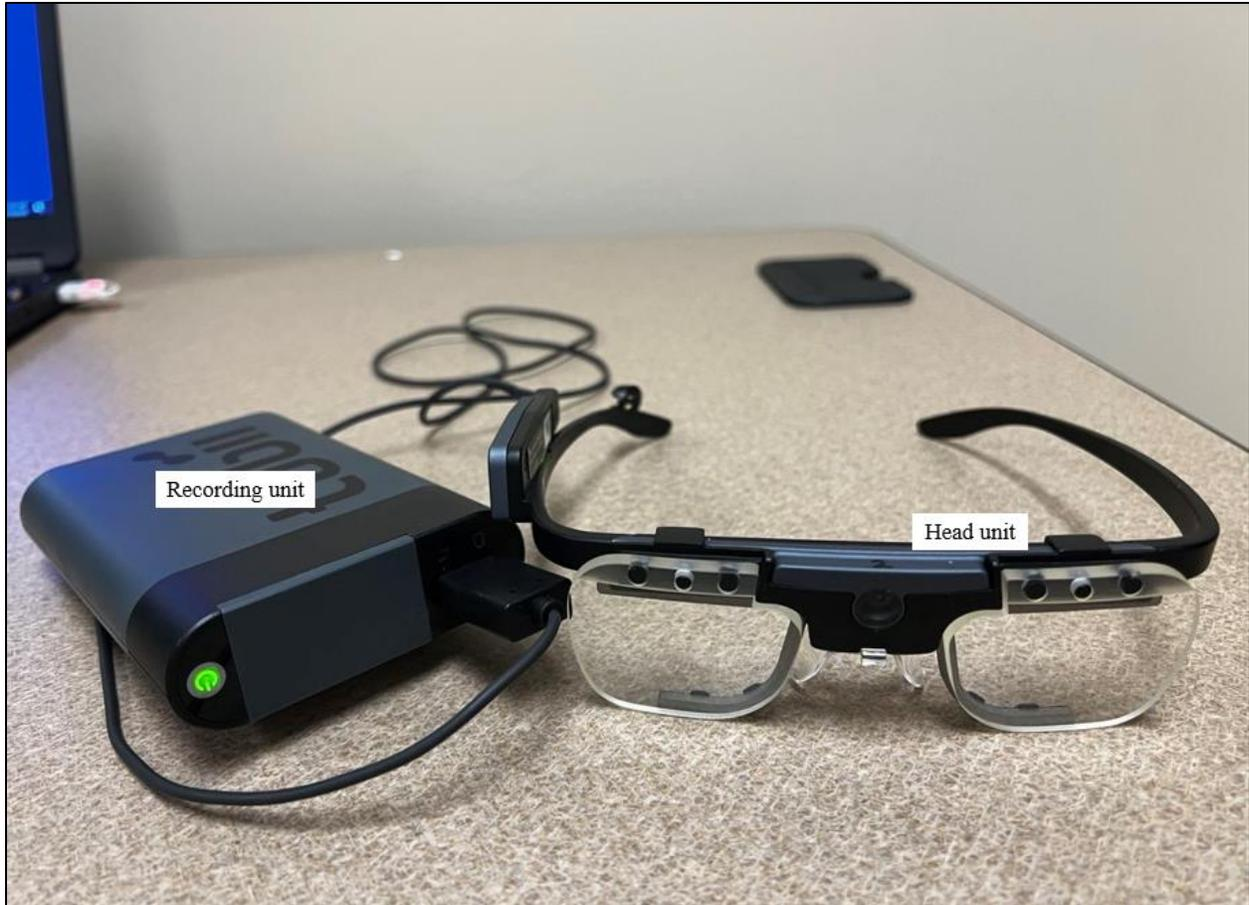
**Figure 3.2 Tobii Pro Glasses 2 Wearable Eye Tracker**
