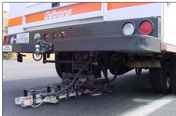
Figure 3.36: Falling weight deflectometer (FWD).
