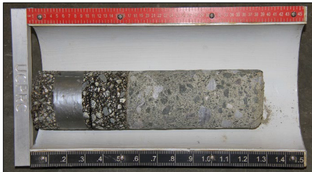
Figure 3.41: Core with asphalt concrete surface on cement-treated base.
