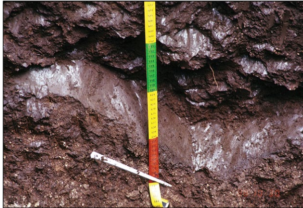
Figure 3.51: Slickenside in subgrade soil (USDA Natural Resources Conservation Service).
