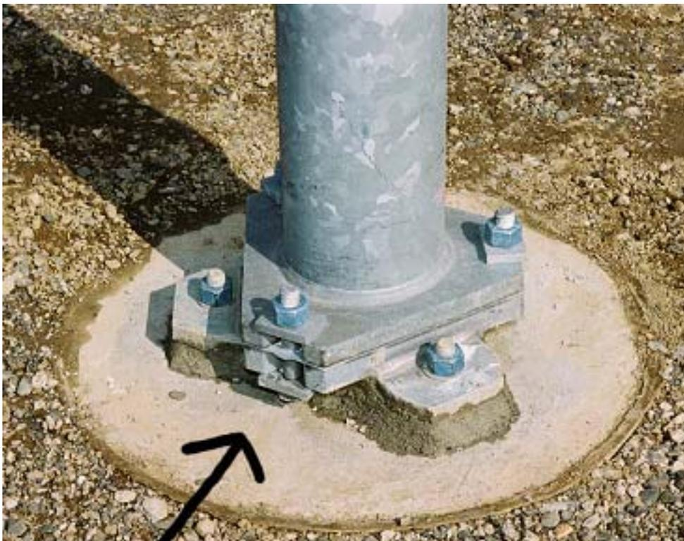
Figure 2-38. Close-Up View of Type 30/31 Slip-Base Used in Test 618
