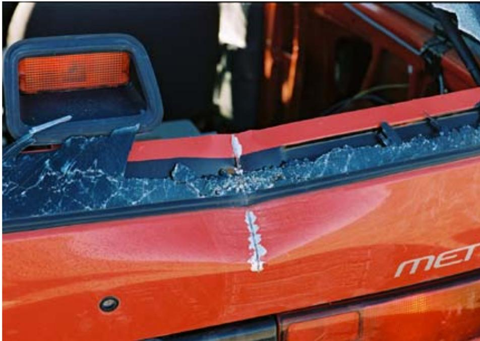
Figure 2-27. Lower Section of Hatchback of Test Vehicle After Test 614
