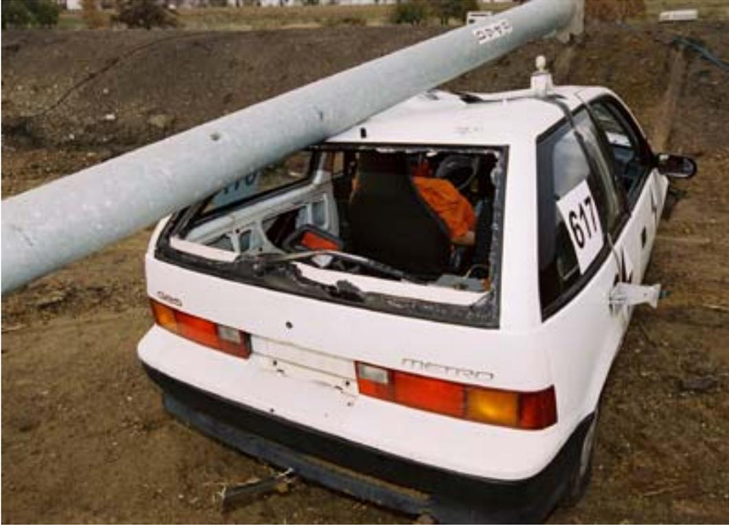
Figure 2-65. Damage to Rear Roof
