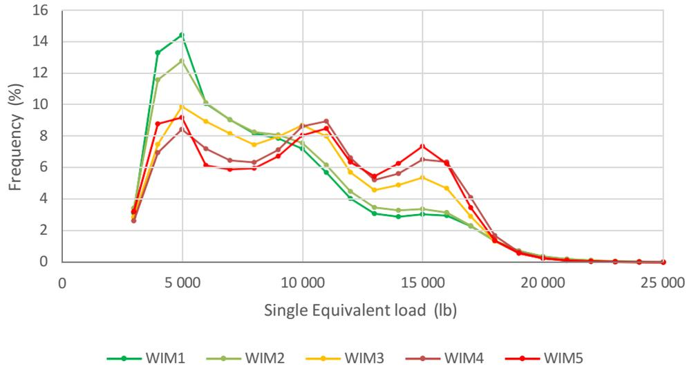
**Figure 2.1: Distribution of *Single Equivalent* loading of the different WIM spectra.**
