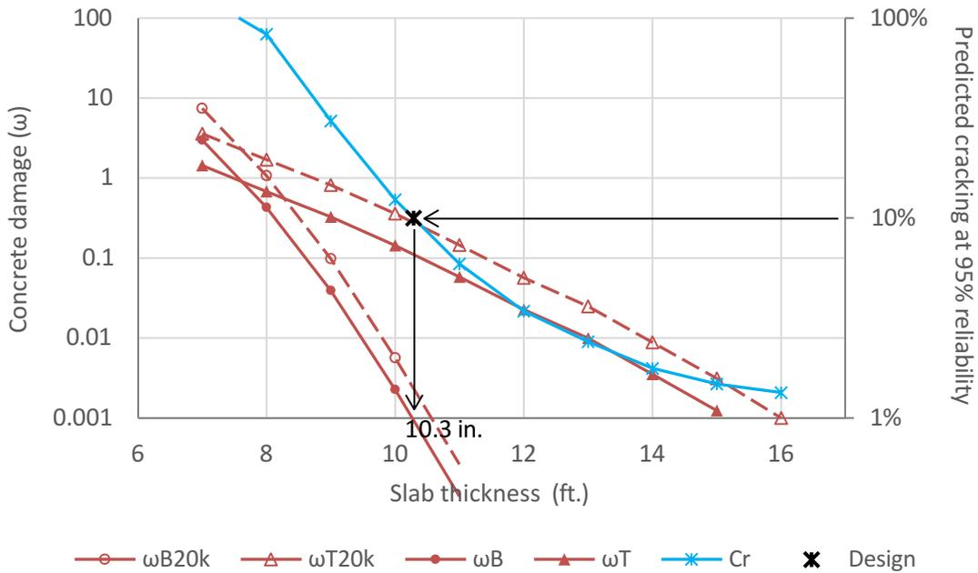
**Figure 3.1: Illustration of approach for determining slab thickness.**
