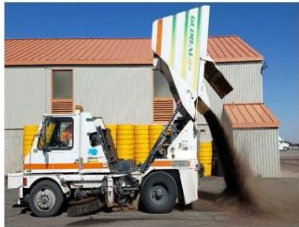
**Figure 5-3 a) Global M4HSD high-side dump sweeper and, b) Global M4 rear dump sweeper**
