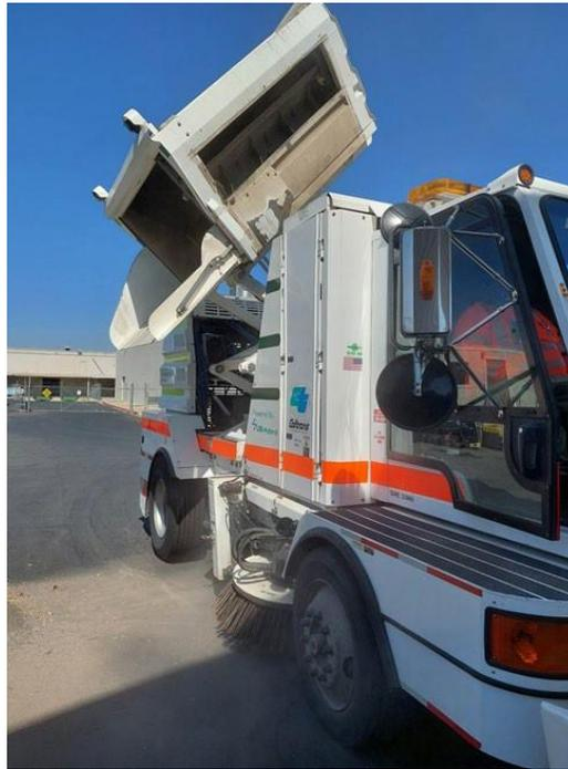
**Figure 3-4 Global M4 HSD high side dump street sweeper.**
