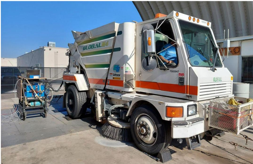
**Figure 6-1 Chassis dynamometer test set up**
