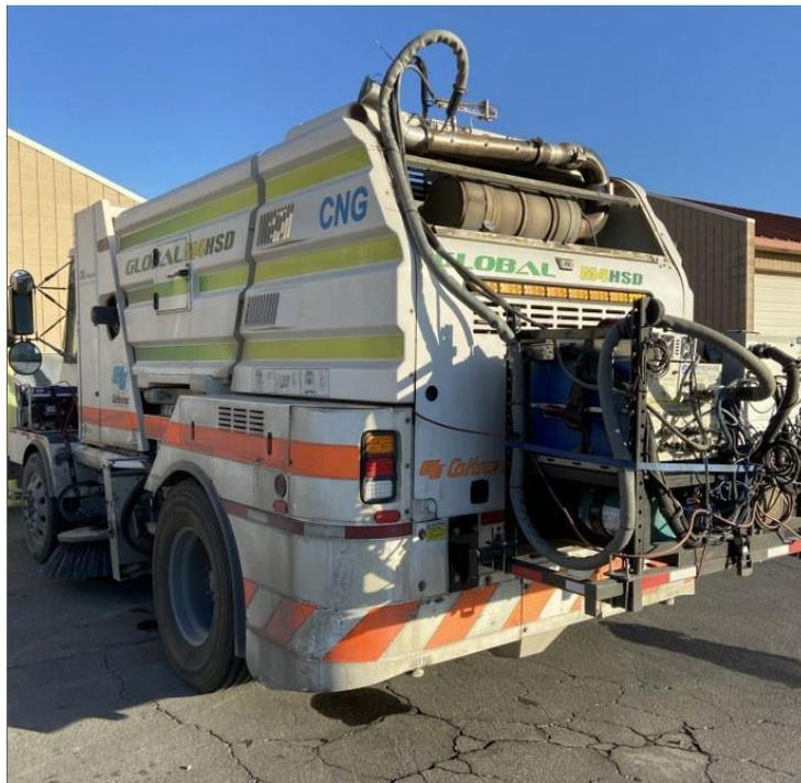
**Figure 5-1 PEMS unit mounted to rear of HSD street sweeper**
