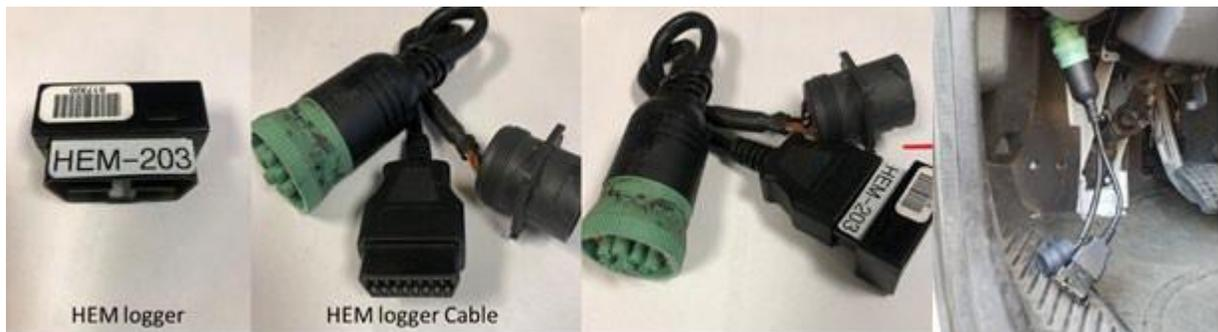
**Figure 4-1. HEM data logger and installation**
