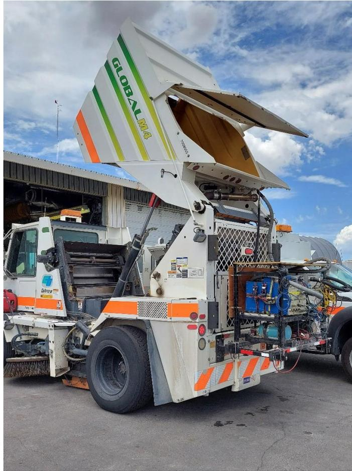
**Figure 5-2 PEMS unit mounted to rear of rear-dumping street sweeper**
