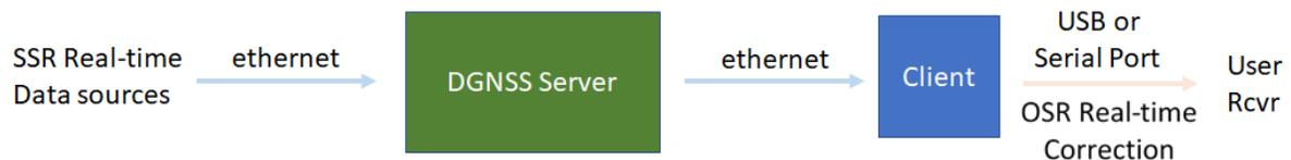
Figure 1. Client Server architecture
