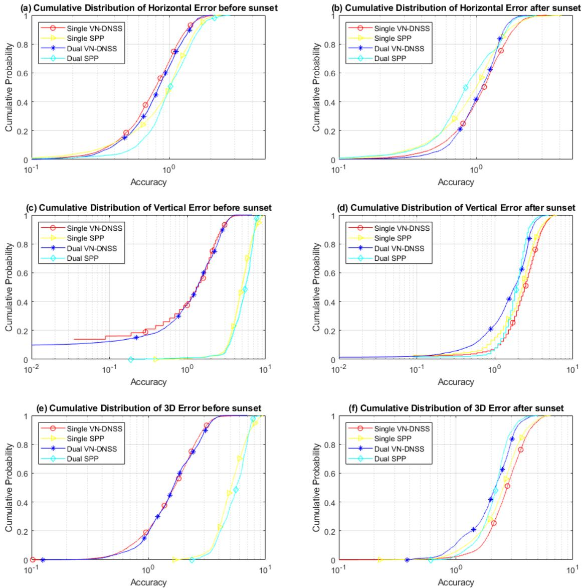
Figure 4: Figure (a), (c), and (e) show the cumulative distribution of the horizontal, vertical, and 3D position error in stationary test before sunset, respectively. Figure (b), (d), and (f) show the cumulative distribution of the horizontal, vertical, and 3D position error in stationary test after sunset, respectively.
