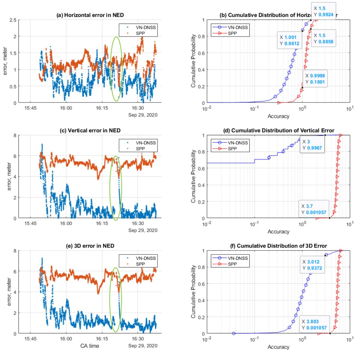
Figure 6: Figure (a), (c), and (e) are the horizontal, vertical, and 3D position error in NED frame plotted versus time respectively. The x-axis shows CA local time in 24-Hr format. Figure (b), (d), and (f) show the cumulative distribution of the horizontal, vertical, and 3D position error respectively. The red curve corresponding to the u-blox in DGNSS mode using the RTCM messages sent by the UCR VN-DGNSS server. The blue curve corresponding to the u-blox in SPP mode.
