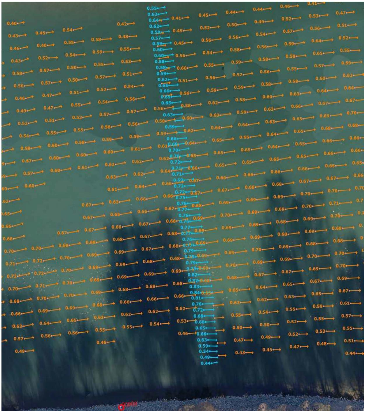
**Figure 4.15: RIVER LSPV and ADCP result overlaid on the orthophoto. The average ADCP data are represented by light blue arrows, and the orange arrows represent LSPV results from the 4K UAS color video. The blue text represent the surface flow estimate calculated from the average ADCP measurement values, and the orange text represents the LSPV estimates.**
