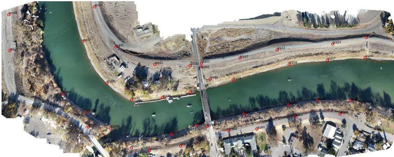
**Figure 4.2: SR13 pilot study site Ground Control Points (GCP) overlaid on top of orthophoto created by WebODM**
