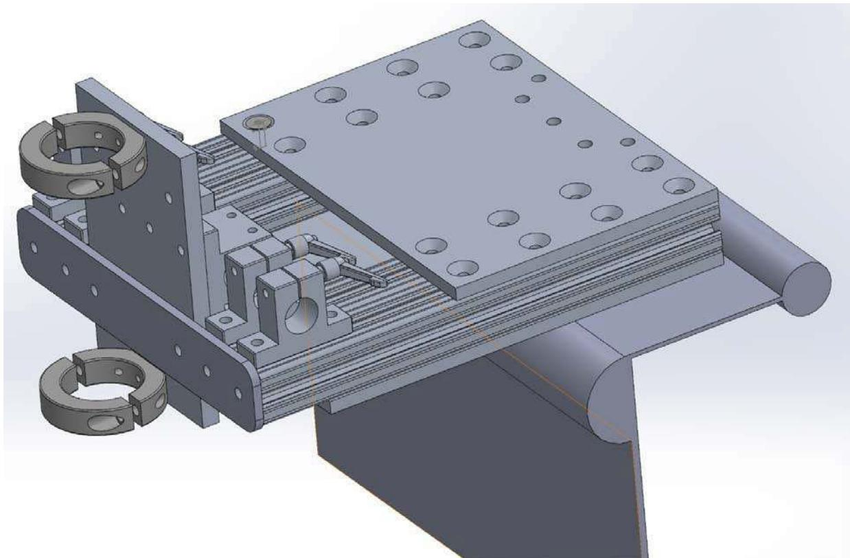
**Figure 3.13: Sensor mount CAD model**
