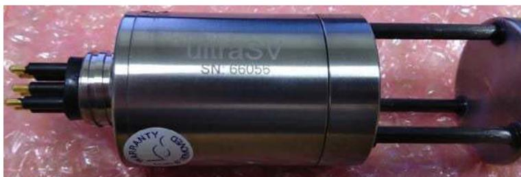
Figure 2.5: Valeport sound velocity sensor, model: UltraSV and S/N: 66056
