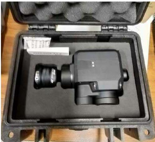
**Figure 2.3: FLIR XT2 IR and color camera**
