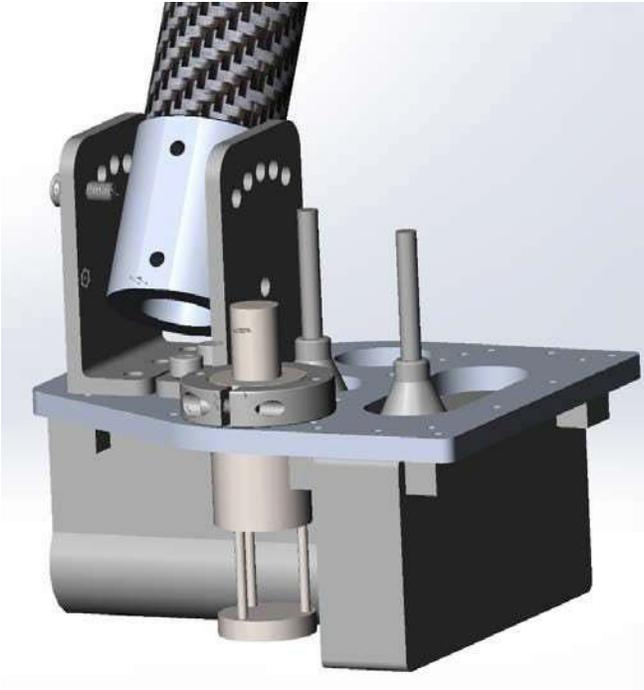
**Figure 3.4: PicoMBES 120 sensor assembly with cover CAD model**
