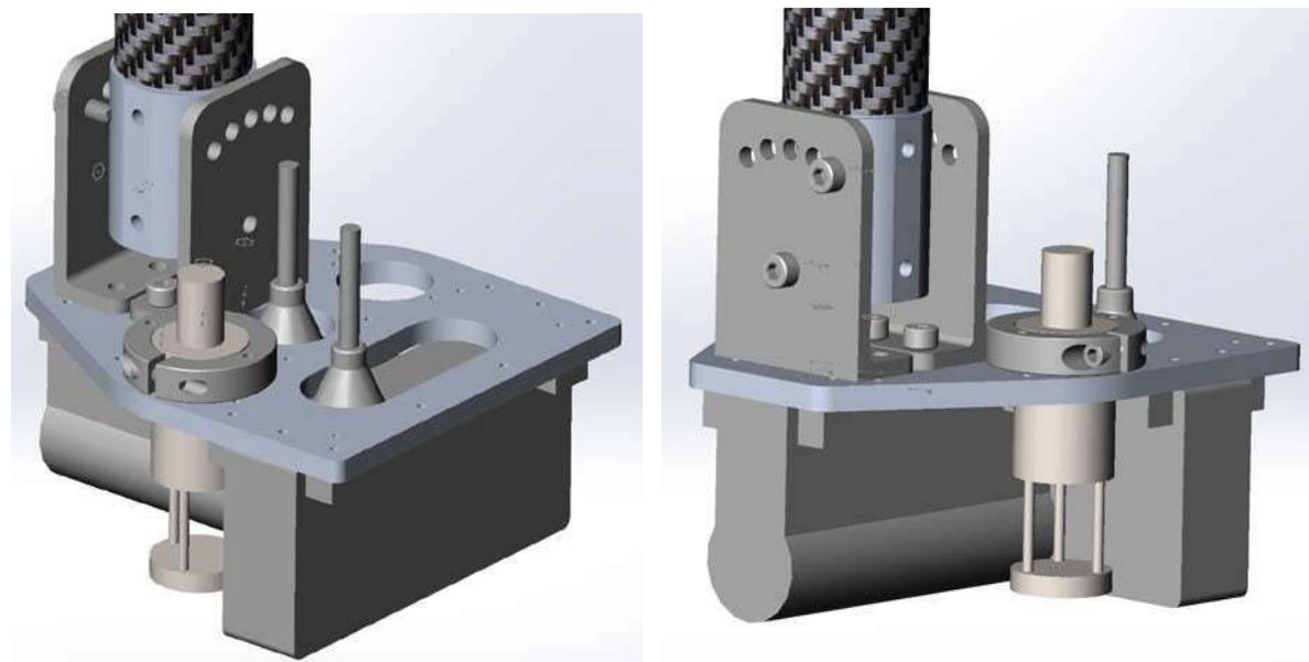
**Figure 3.3: PicoMBES 120 sensor assembly CAD model**
