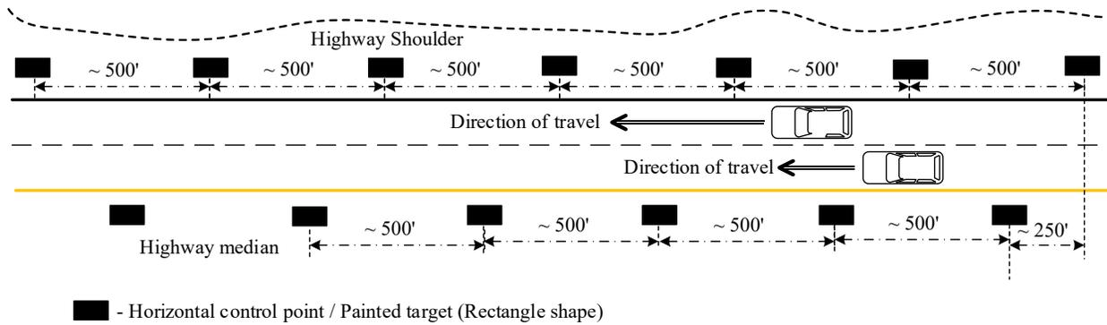
**Figure 6.1: GTPG MTLs control target layout design**
