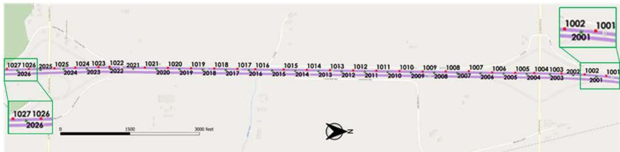
**Figure 6.3: Aerial view of GTPG site MTLs targets overlaid on Microsoft Bing Maps. The red squares with numbers 10xx mark the location of MTLs targets on the shoulder. The green squares with numbers 20xx mark the location of MTLs targets on the median.**
