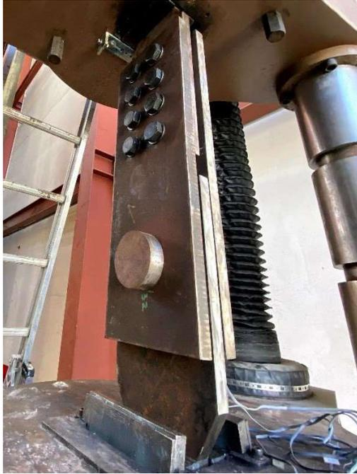
Figure 3.3 Pin Plate Test Setup
