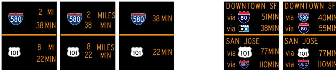
Figure 16. Proposed Design for Up to Six Lines Messages
