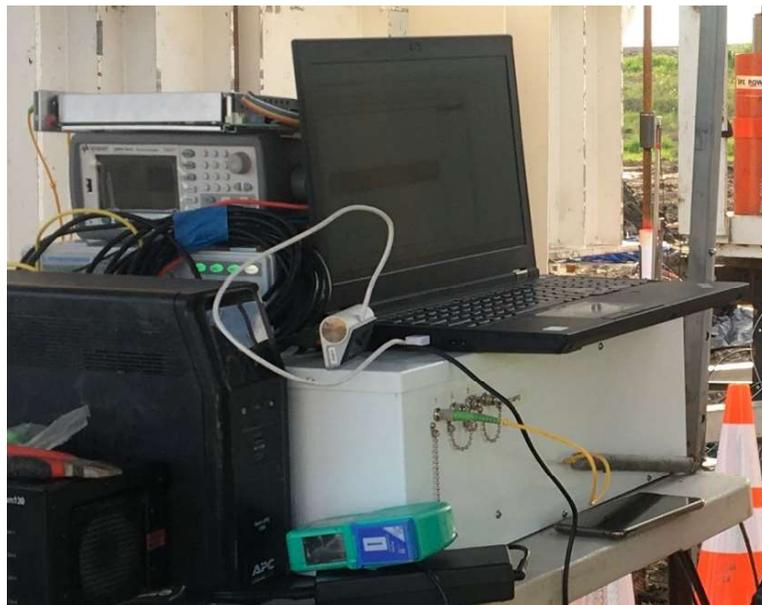
*Figure 4-8: ALICIA fiber optic analyzer during load test*
