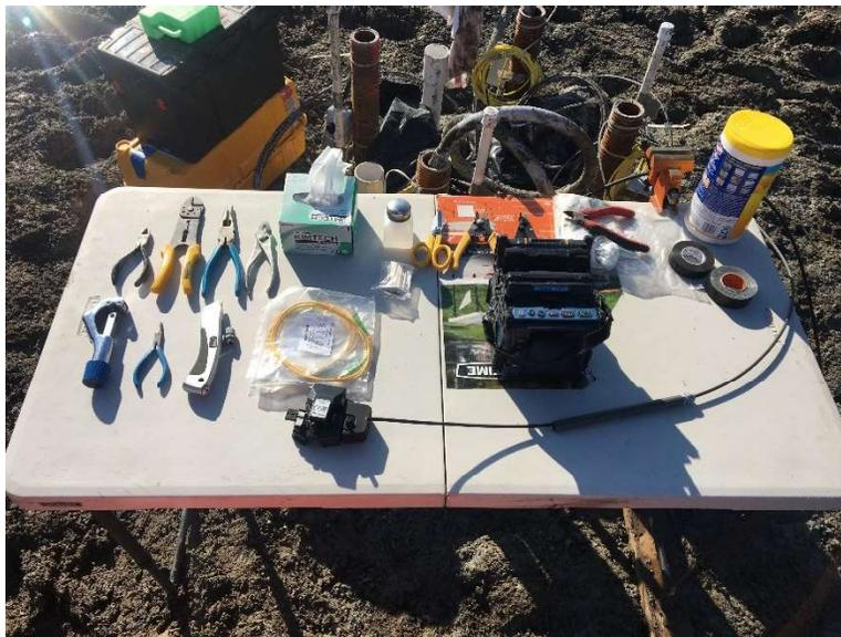
*Figure 4-17: Photo of the field setup and tools used for splicing fiber optic cables from the piles*
