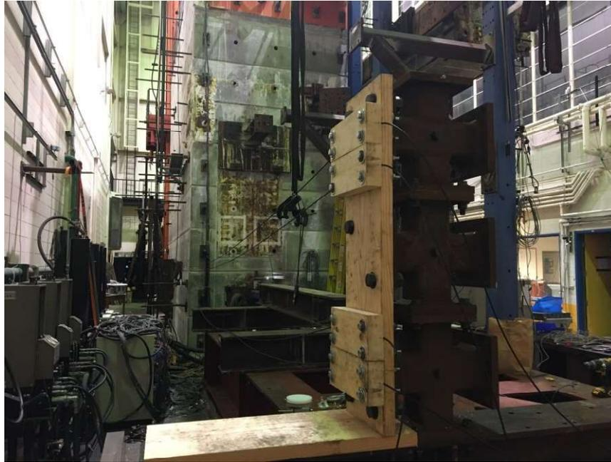
*Figure 3-3: Photo of wood clamp setup at far corner of 1D shake table*
