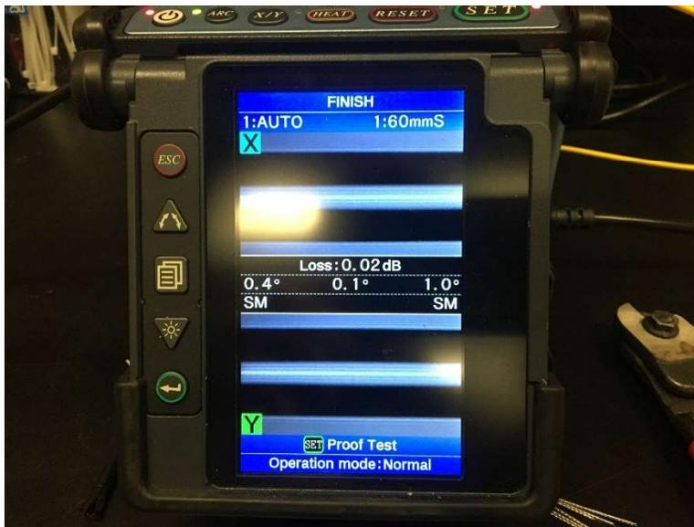
Figure 4-20: Photo of completed splice between strain cable (left) and FC patch cable (right)
