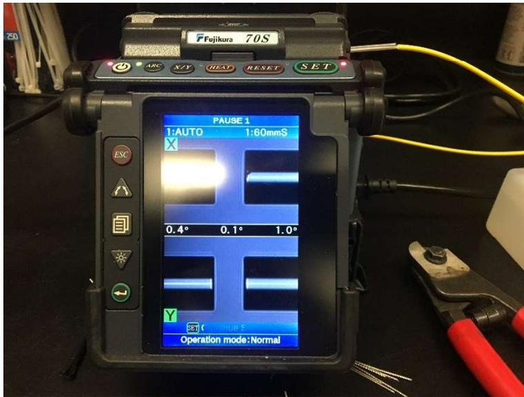
Figure 4-19: Fujikura fusion splicer, joining strain cable (left) and FC patch cable (right)
