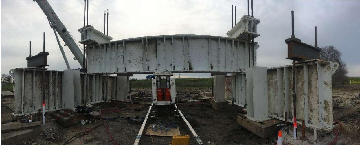
*Figure 1-3: Load test frame*
