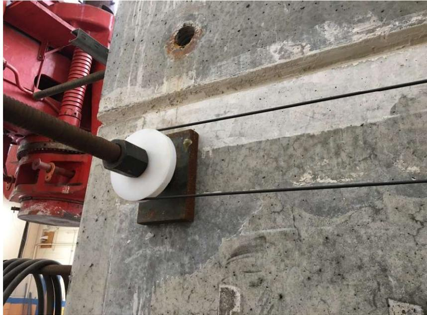
*Figure 3-2: Photo of Loop 2 (long loop) pulley mounted on strong wall*
