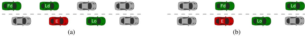
Figure 20: In (a), the left lane is moving faster than the right lane. The ego vehicle decided between which vehicles to merge and they can start creating the gap. Afterwards, in (b),  $F_d$  created the gap between itself and  $L_d$ , but, due to the relative speed between lanes, the gap is not at a suitable location for  $E$ .
