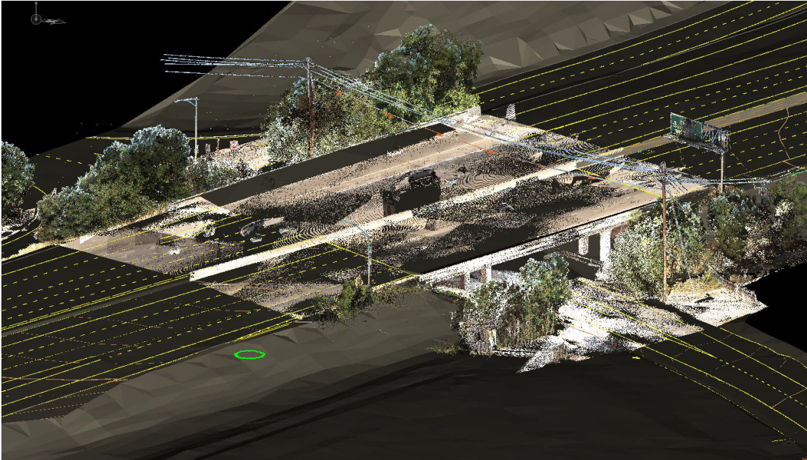
Figure F.3 Route Alameda 680 Express Lane Project Digital Terrain Model and Lidar Data Set
