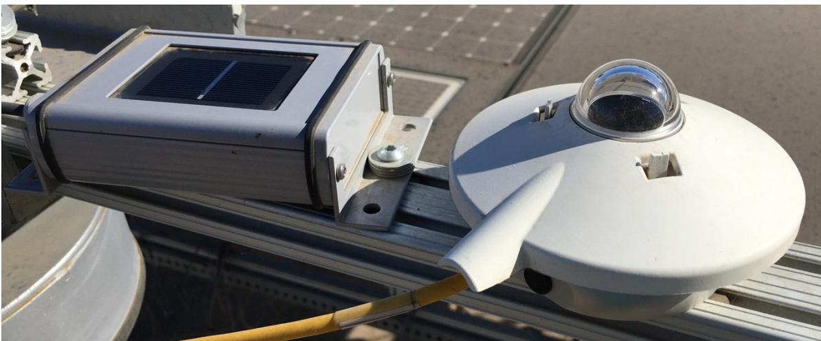
Figure 2.15. Example of reference cell and pyranometer mounted in same plane.
