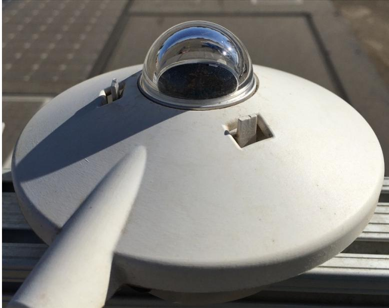
**Figure 2.1. Example of pyranometer.** The glass dome allows light to strike the black thermopile from any angle.
