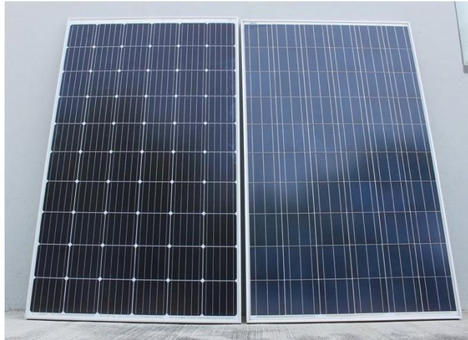
**Figure 6.7. Typical commercial solar modules: a monocrystalline silicon solar (left); a multicrystalline silicon solar (right).** The monocrystalline silicon solar module's distinctive pattern is a result of trimming the round ingot shape into an almost square (pseudosquare) shape with missing corners. Photo credit: Jorge Luis Carnalla Ortiz.
