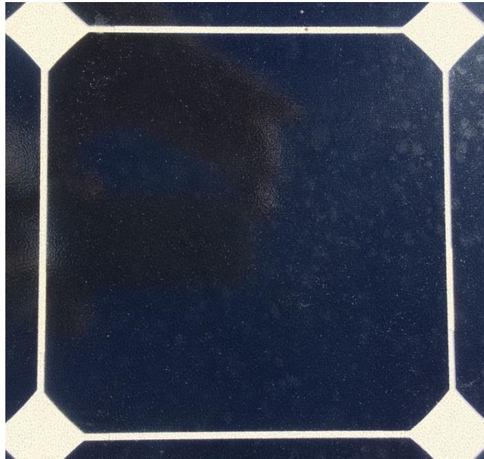
Figure 6.9. Image of cell in SunPower Module with no front grid pattern.
