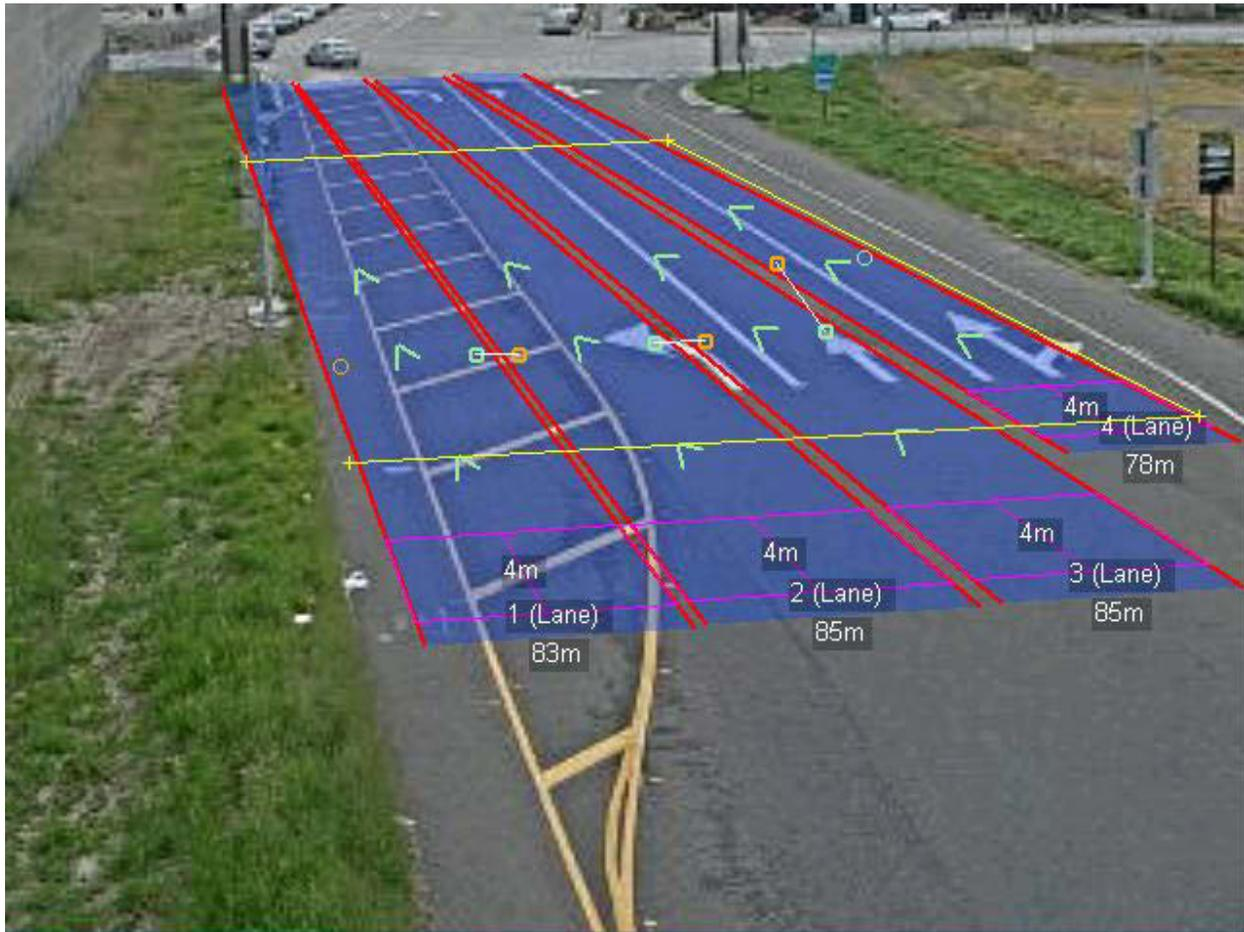
**Figure 3.6: Effect of pole twist on one WWD monitoring installations' lane masks. US 50 WB South River Road exit ramp. Note the significant discrepancy between mask lines and actual lane lines. These were aligned at the time of camera installation.**
