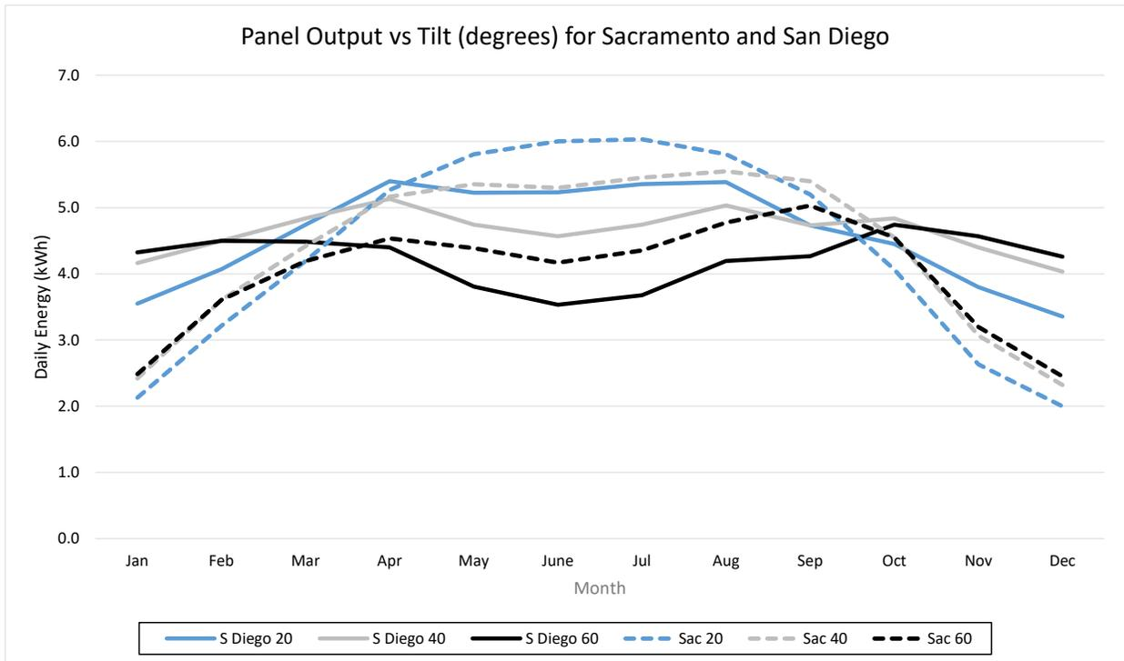
**Figure 3.4: Solar panel output per day over the full year for various panel tilt angles from horizontal for Sacramento and San Diego, California<sup>1</sup>**
