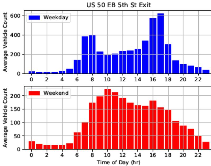
**Figure 4.4: Traffic count as determined from camera analytics for eastbound (EB) US 50 to 5<sup>th</sup> Street exit ramp in Sacramento**
