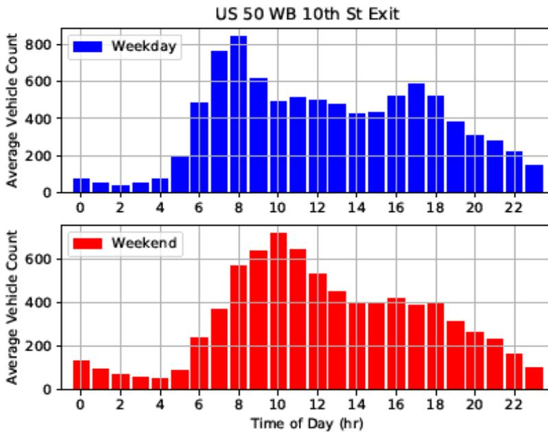
Figure 4.7: Traffic count as determined from camera analytics for WB US 50 to 10<sup>th</sup> Street exit ramp in Sacramento
