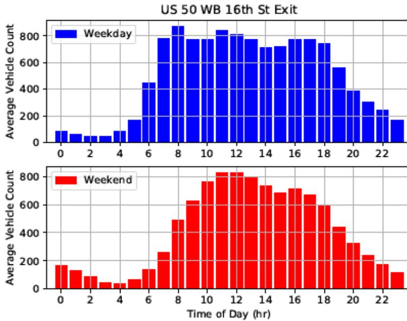
**Figure 4.8: Traffic count as determined from camera analytics for WB US 50 to 16<sup>th</sup> Street exit ramp in Sacramento**
