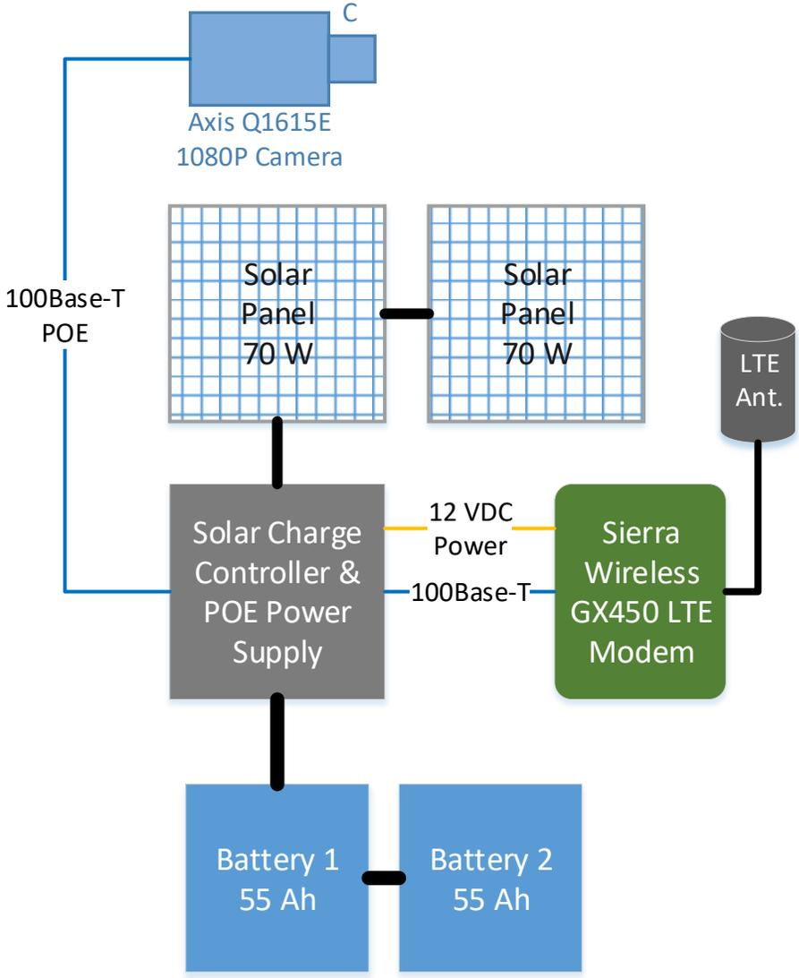
**Figure 2.1: The WWD VBSM system block diagram**
