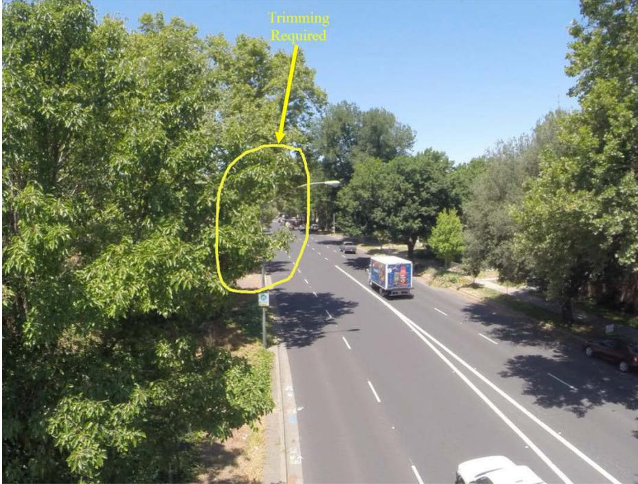
**Figure 3.2: Example of tree trimming required to provide better camera FOV (US 50 WB 10<sup>th</sup> St exit)**
