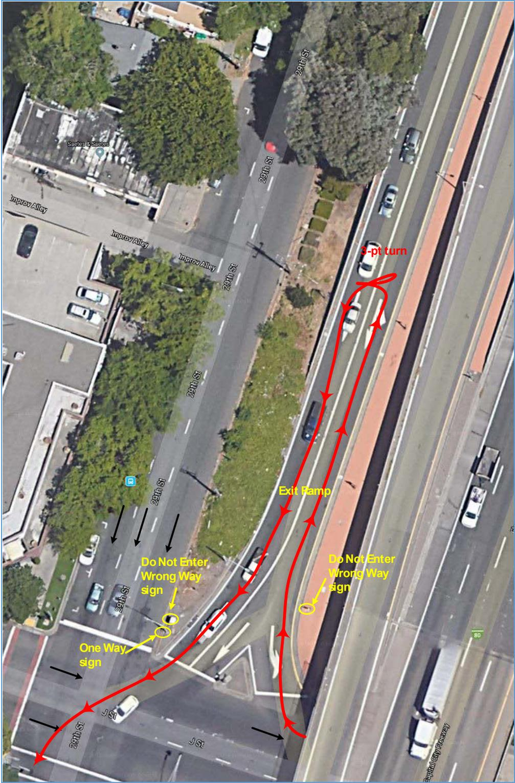
Figure A.6: Aerial view of the 3/8/2018 1:30 am WWD event on the J Street exit ramp. Approximate vehicle trajectory is shown in red. Aerial image courtesy of Google Maps.
