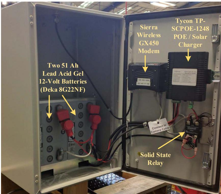
Figure 2.2: The WWD VBSM system component details
