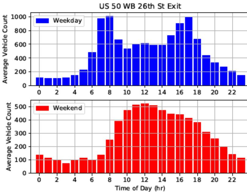
**Figure 4.9: Traffic count as determined from camera analytics for WB US 50 to 26<sup>th</sup> Street exit ramp in Sacramento**
