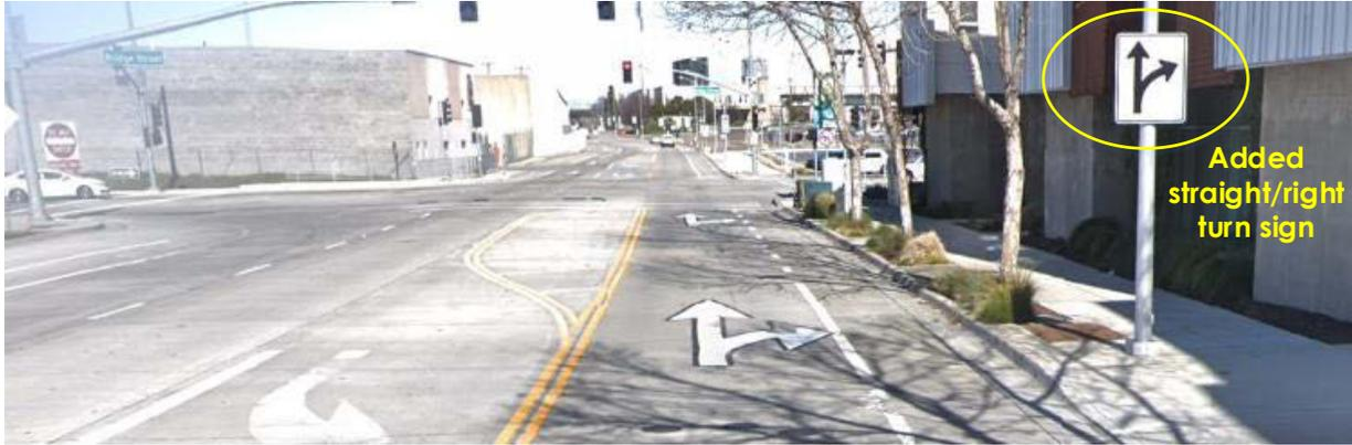
Figure 4.35: Caltrans' sign addition for northbound 5<sup>th</sup> Street on the south side of the intersection at the South River Road exit ramp. Image courtesy of Google Street View.
