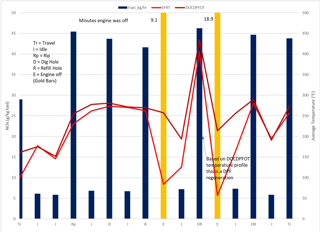
**Figure 4-9: Fuel consumption rate by mode of operation for 2014 tier 4F John Deere 1050K Crawler Tractor**
