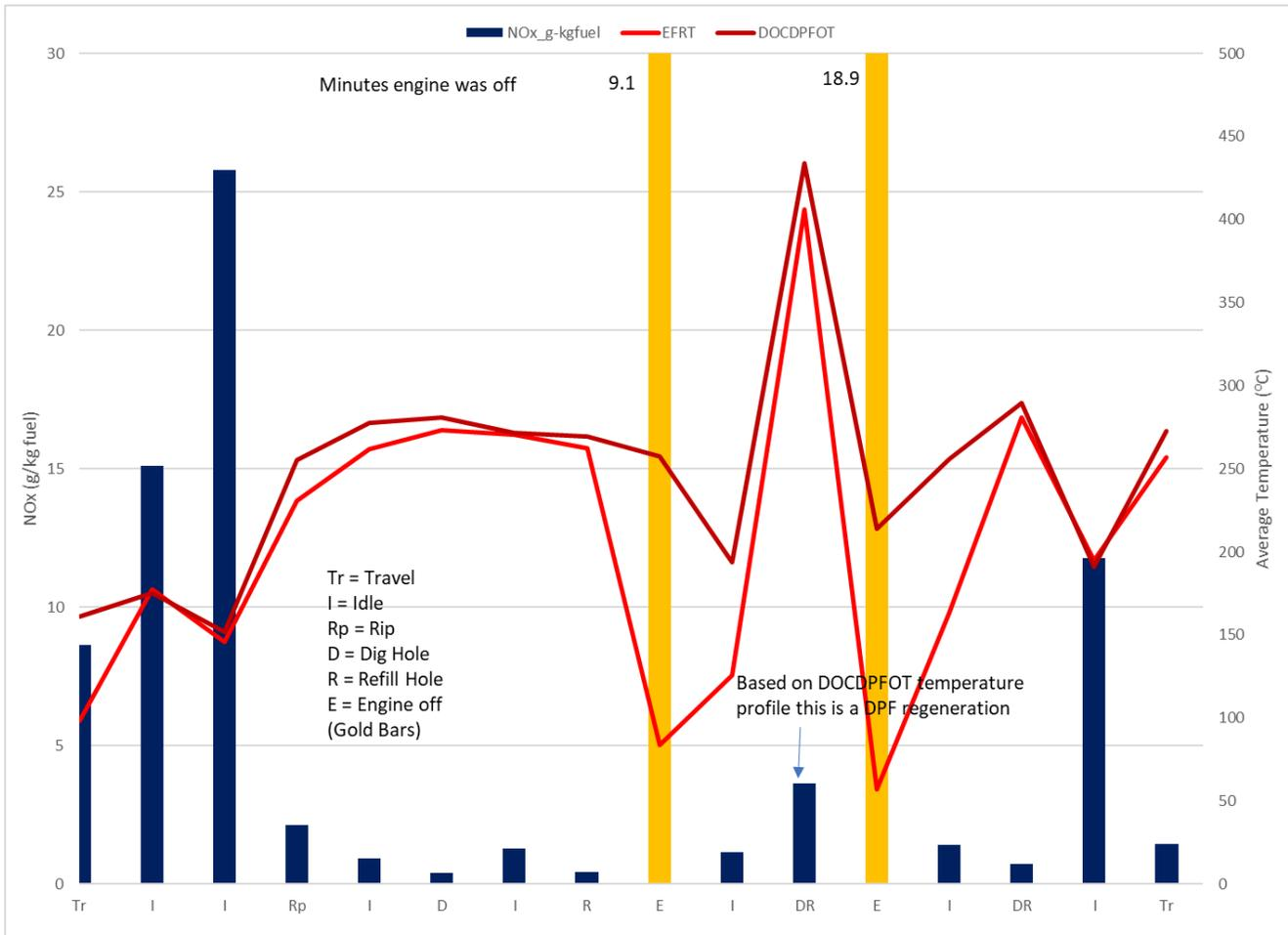
**Figure 4-7: Fuel based NOx emissions by mode of operation for 2014 tier 4F John Deere 1050K Crawler Tractor**
