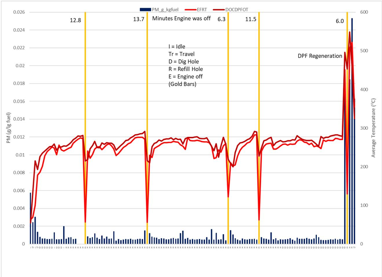
**Figure 4-11: Fuel based PM emissions by mode of operation for 2014 tier 4F John Deere 824KII Wheel Loader**
