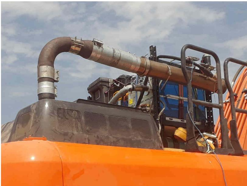
**Figure 2-14: Emission Equipment on Hitachi 210GLC Excavator**
