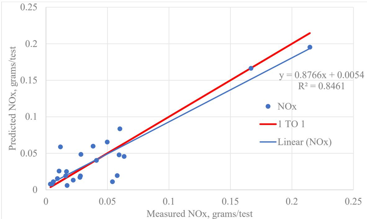
**Figure 5-2 NO<sub>x</sub> calibration results for 10 units (23 tests) in development dataset.**
