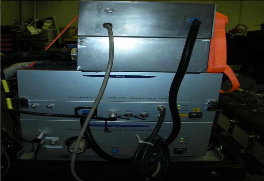
**Figure 2-2: AVL Micro Soot Sensor with Gravimetric Filter Box on Top**
