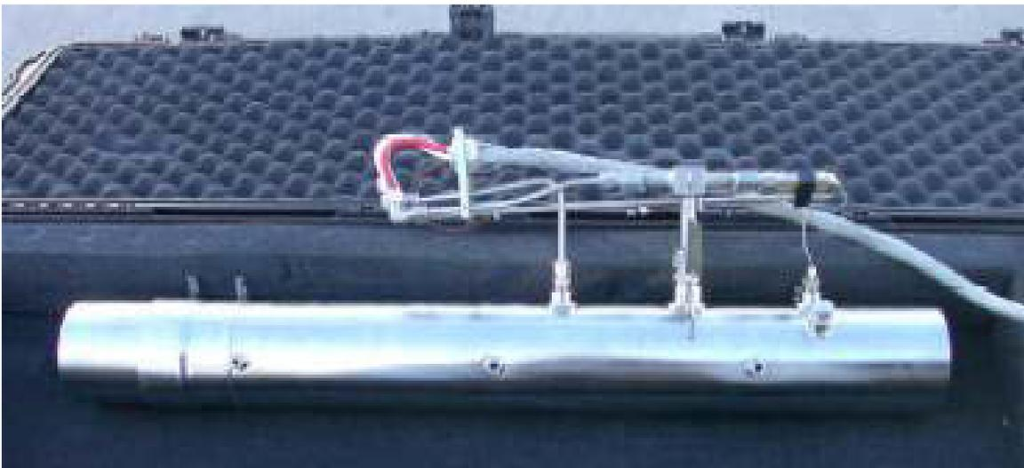
**Figure 2-3: Semtech DS Exhaust Flow Meter**
