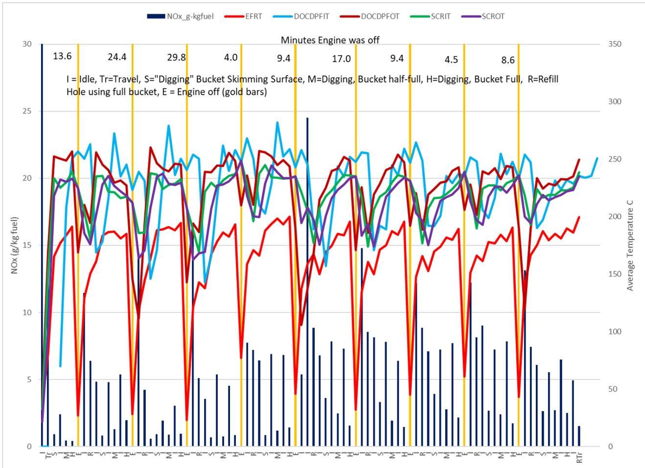
**Figure 4-4: Fuel based NOx emissions by mode of operation for 2015 tier 4F CAT930M Wheel Loader**
