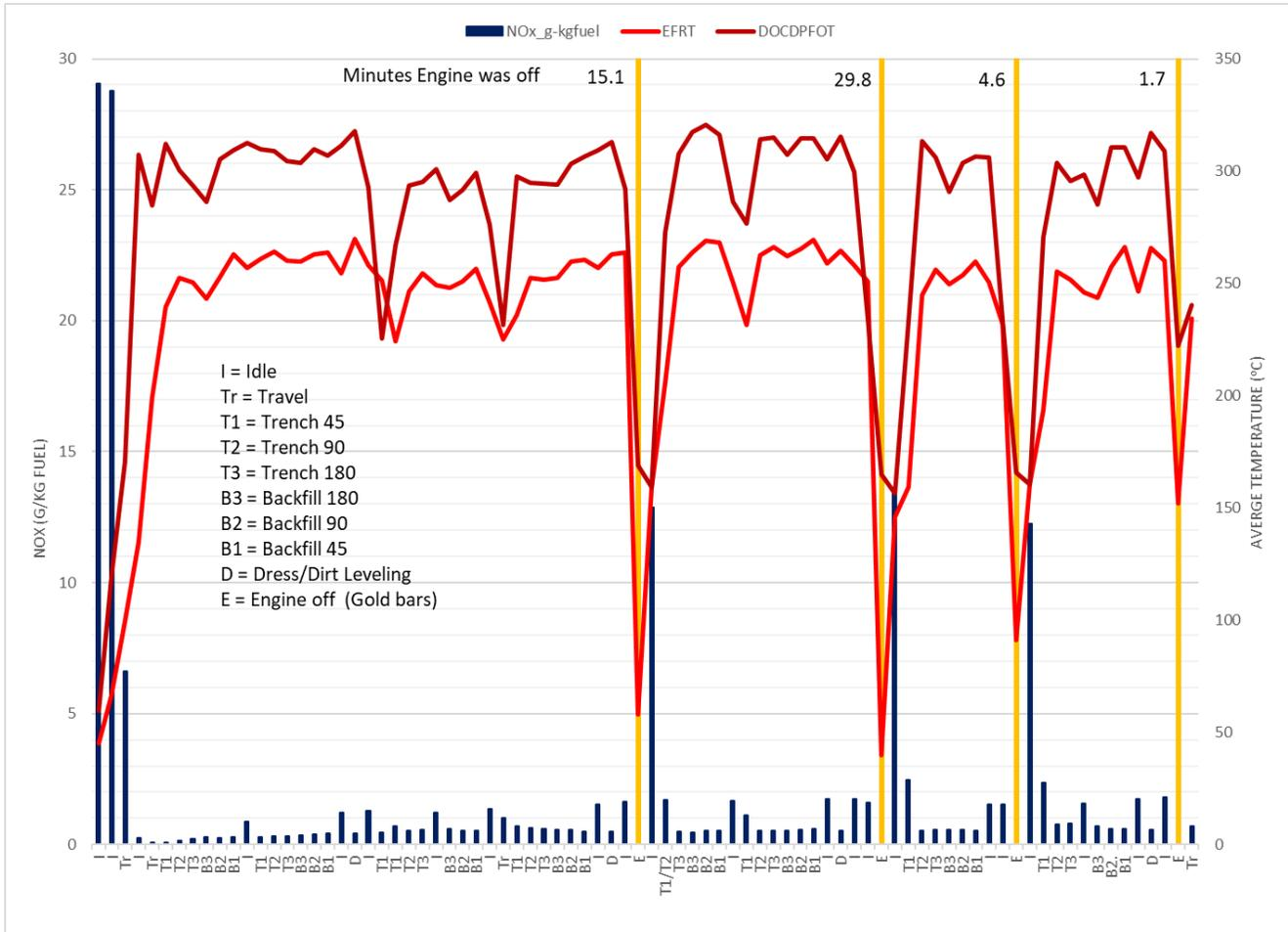
**Figure 4-1: Fuel based NOx emissions by mode of operation for 2015 tier 4F CAT335F Excavator**
