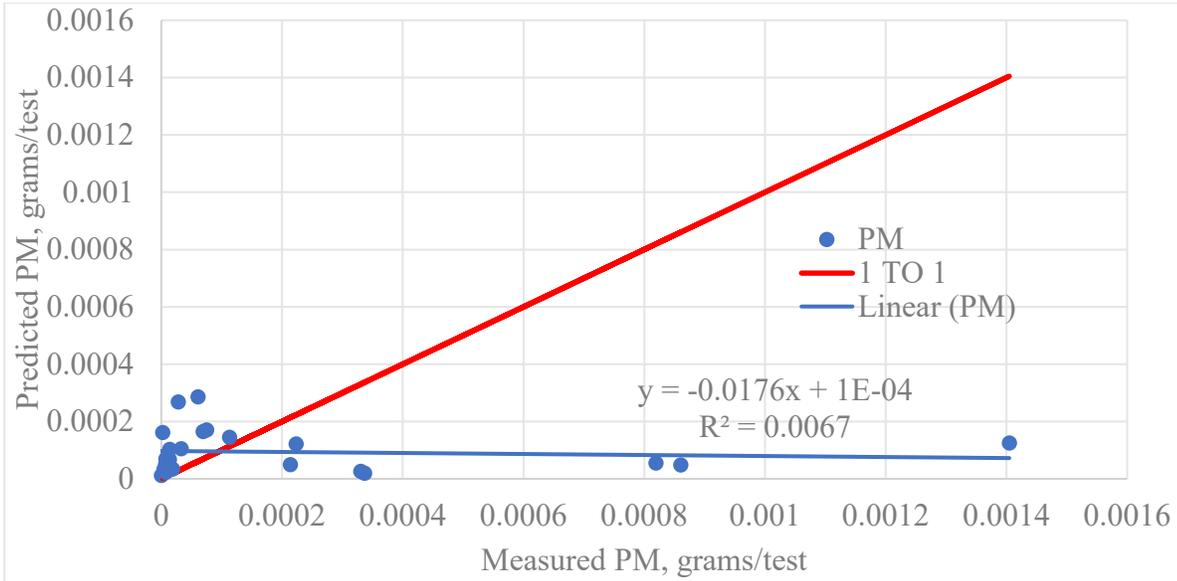
**Figure 5-1: PM calibration results for 10 units (23 tests) in development dataset.**
