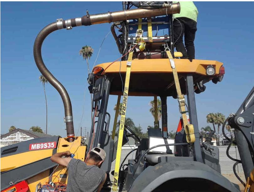
**Figure 2-12: Emission Equipment on JD 310SL Backhoe/Loader**
