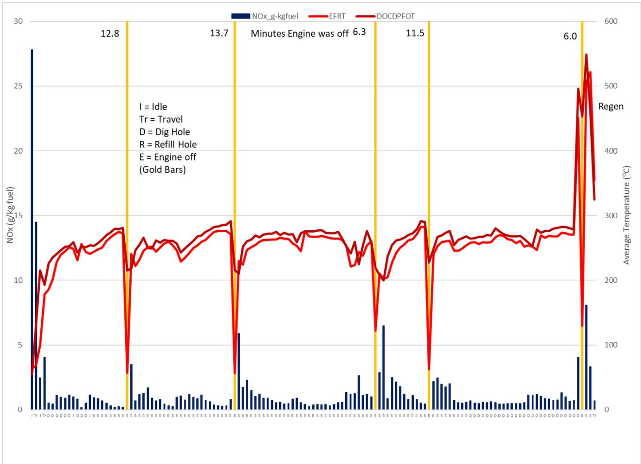
**Figure 4-10: Fuel based NOx emissions by mode of operation for 2014 tier 4F John Deere 824KII Wheel Loader**
