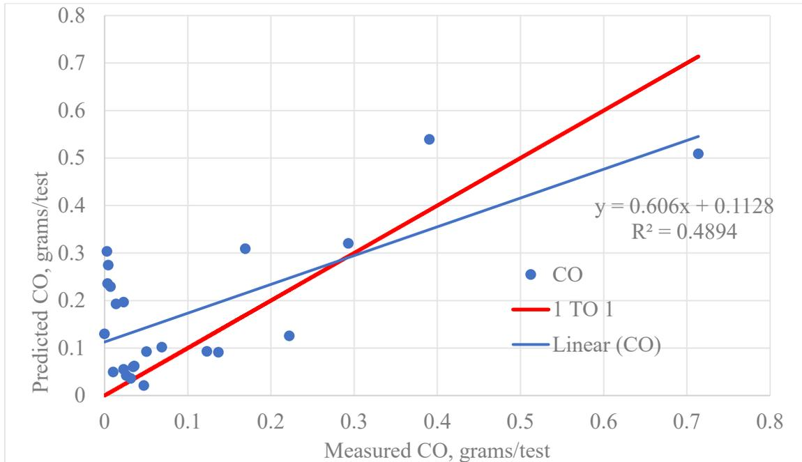
**Figure 5-3: CO calibration results for 10 units (23 tests) in development dataset**
