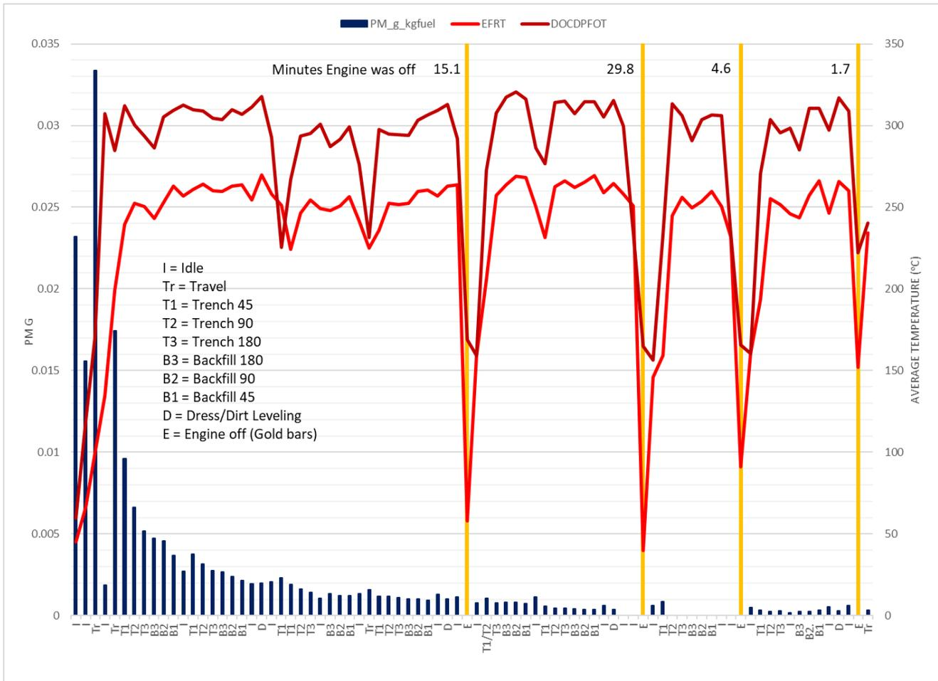
Figure 4-2: Fuel based PM emissions by mode of operation for 2015 tier 4F CAT335F Excavator
