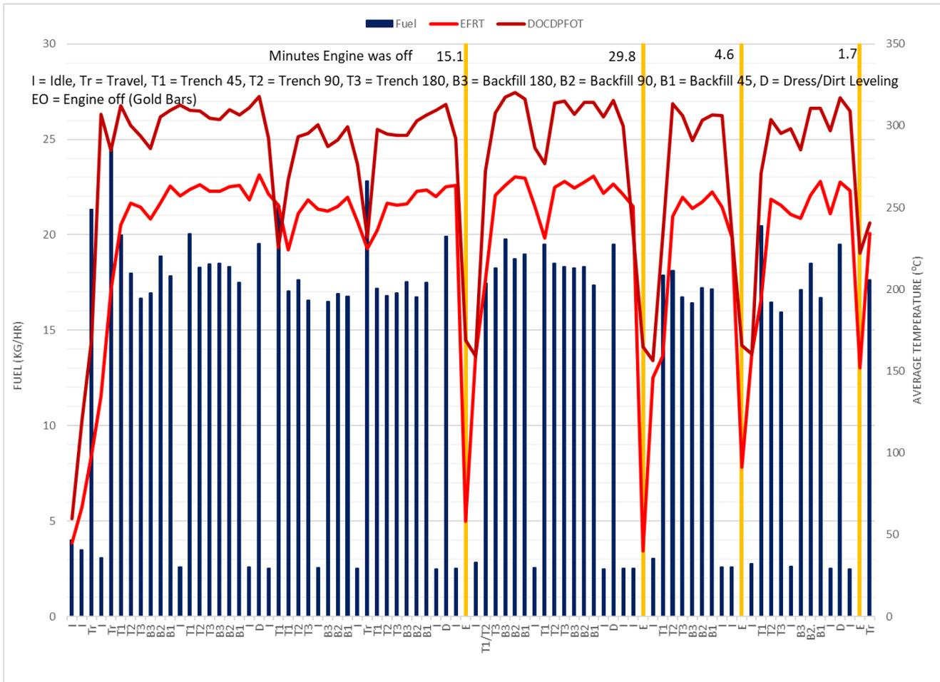
Figure 4-3: Fuel consumption rates by mode of operation for 2015 tier 4F CAT 335F Excavator
