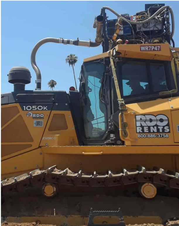
**Figure 2-13: Emission Equipment on JD 1050K Crawler Tractor**
