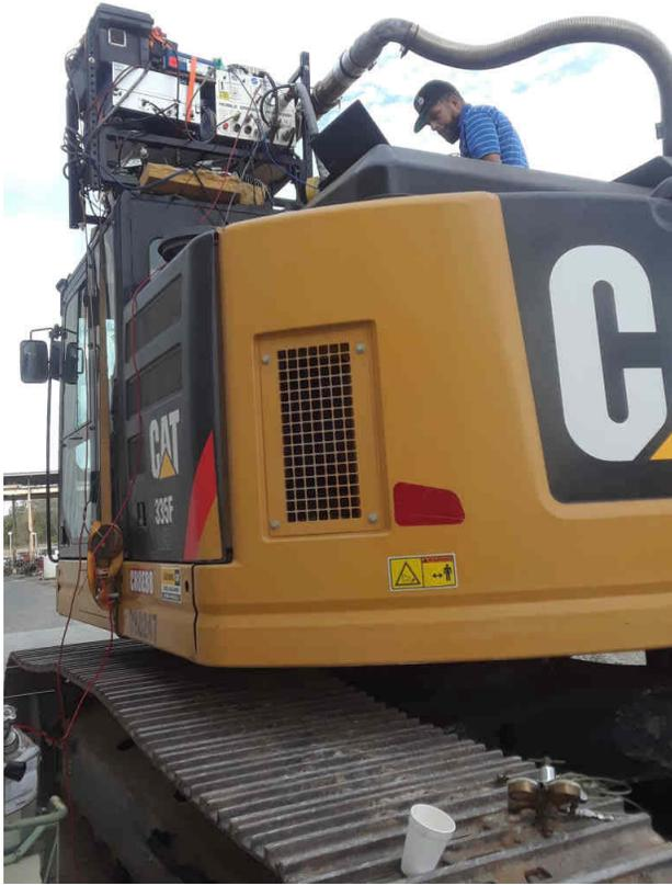
**Figure 2-7: Emission Equipment on CAT 335F Excavator**
