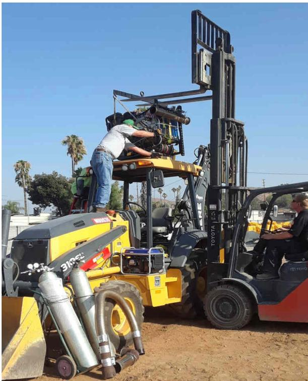
**Figure 2-6: Emission Measurement Equipment being lifted by forklift**
