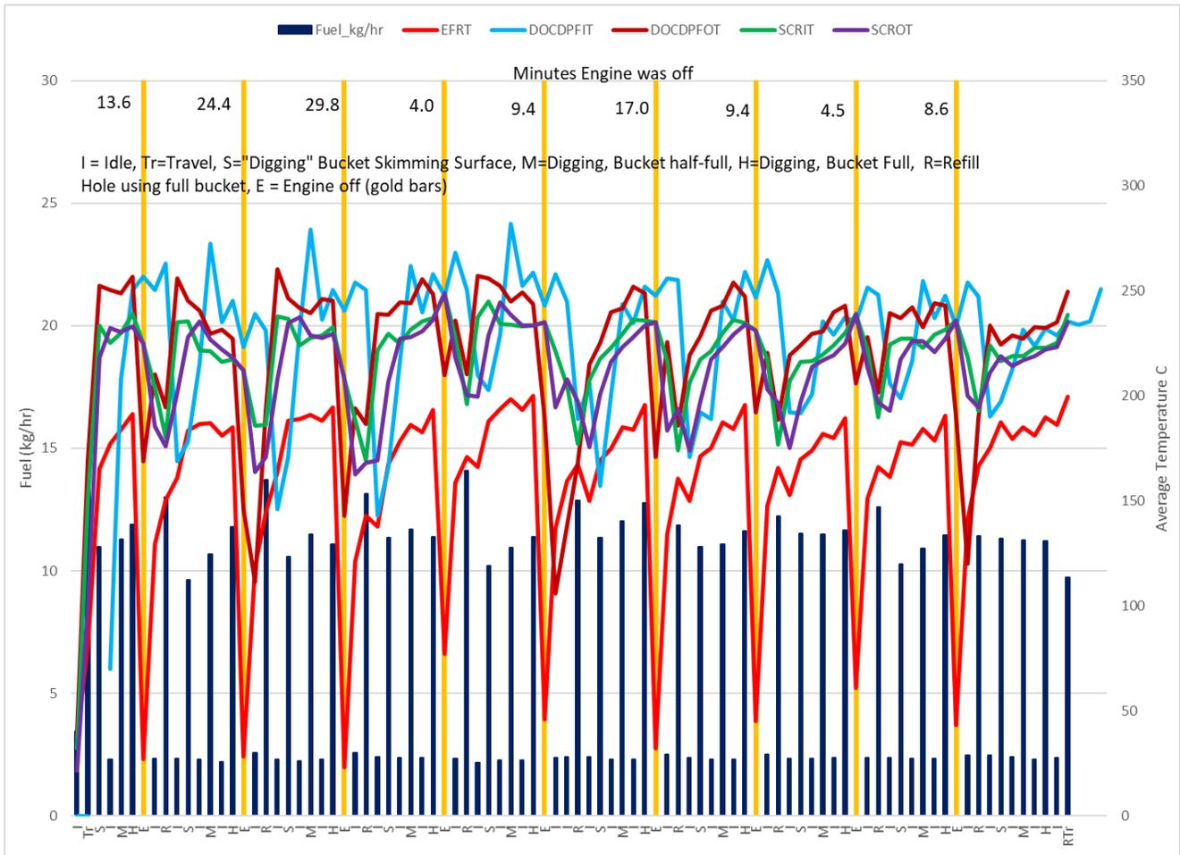
**Figure 4-6: Fuel consumption rate by mode of operation for 2015 tier 4F CAT930M Wheel Loader**
