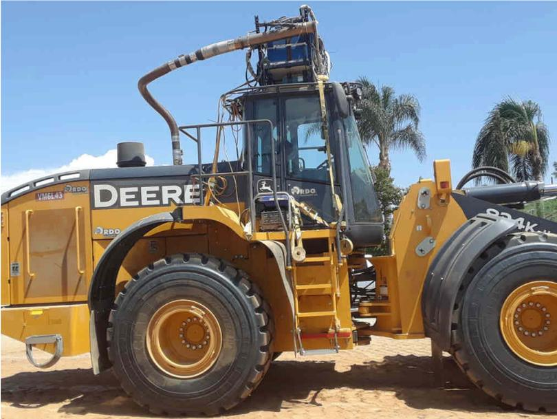
**Figure 2-15: Emission Equipment on JD 824KII Wheel Loader**
