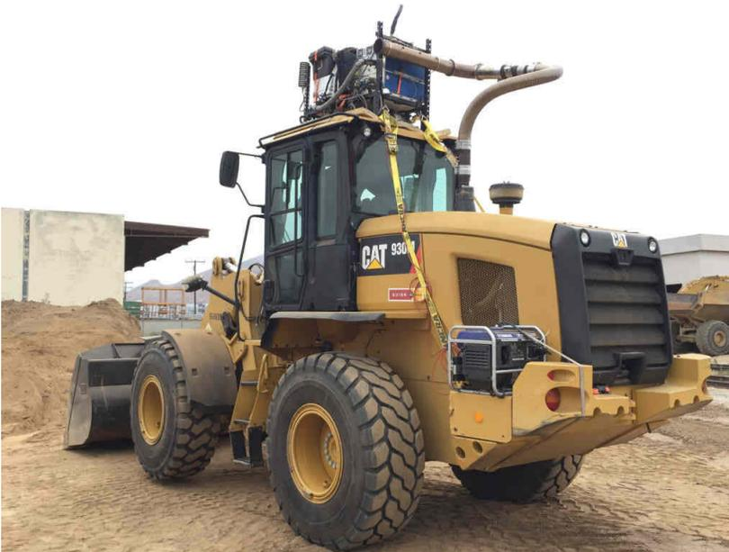
**Figure 2-8: Emission Equipment on CAT 950M Wheel Loader**
