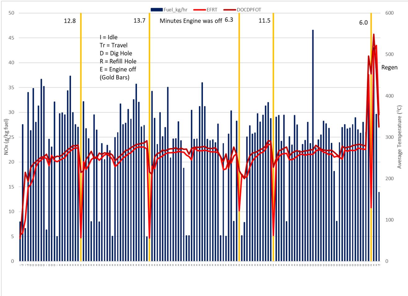
**Figure 4-12: Fuel consumption rate by mode of operation for 2014 tier 4F John Deere 824KII Wheel Loader**
