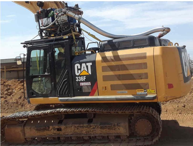
**Figure 2-10: Emission Equipment on CAT 336FL Excavator**
