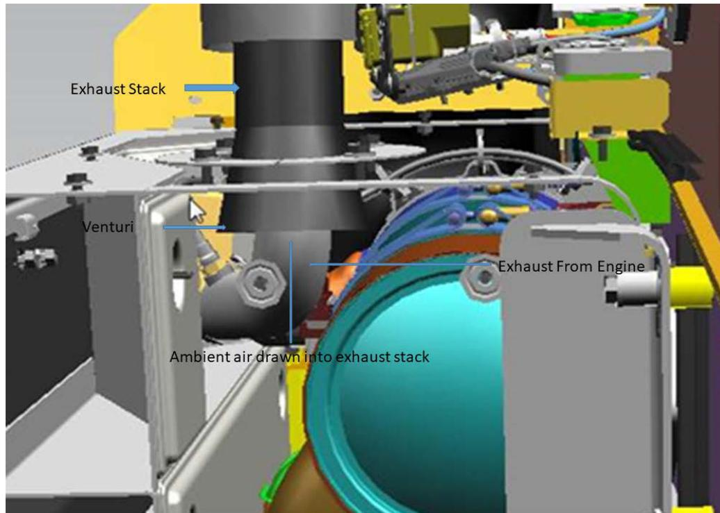
**Figure 3-1: Exhaust Stack Venturi on CAT 430F2**
