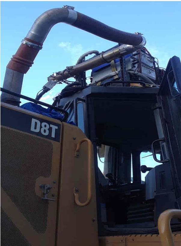
**Figure 2-16: Emission Equipment on CAT D8T Crawler Tractor**
