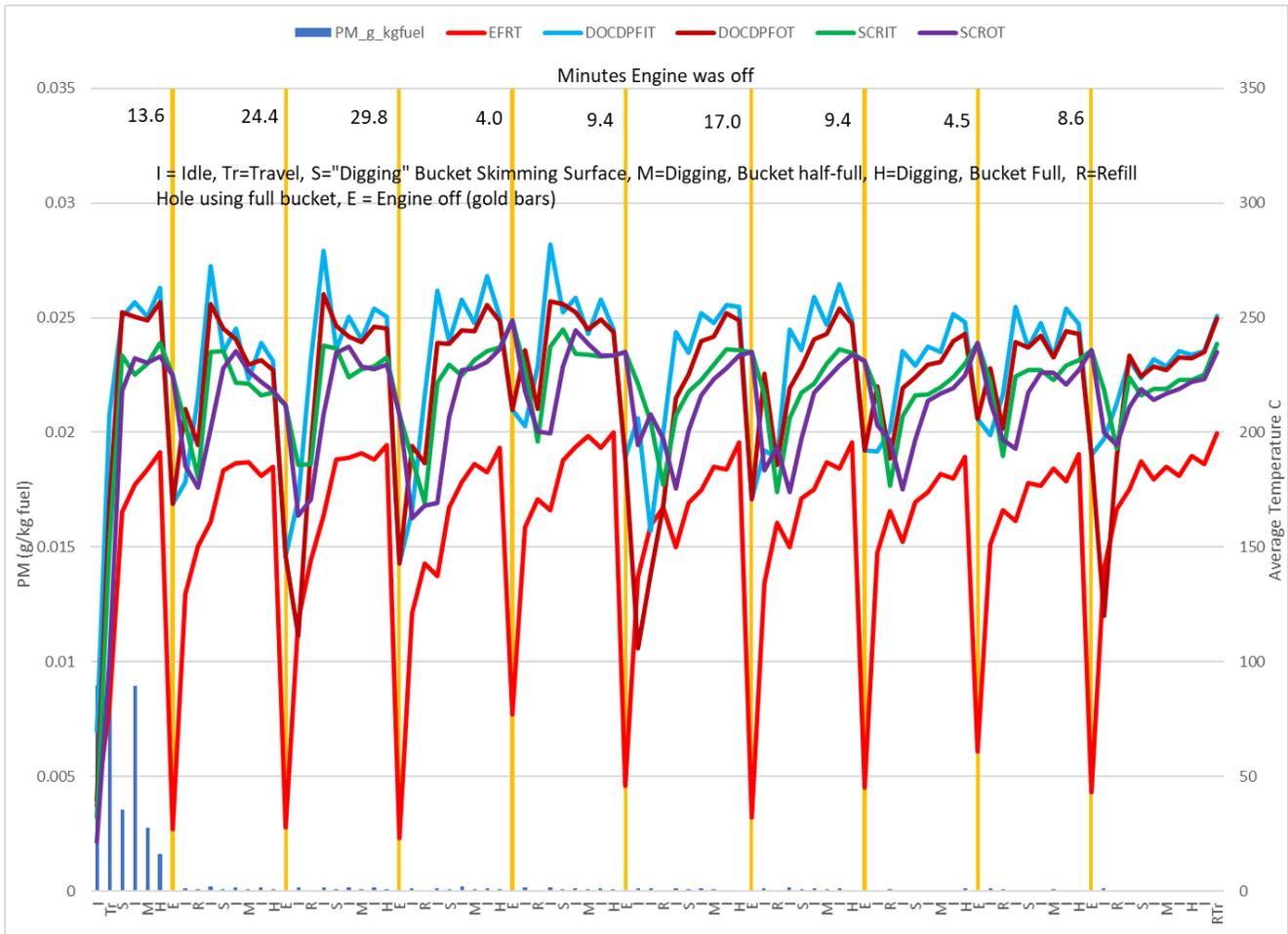
**Figure 4-5: Fuel based PM emissions by mode of operation for 2015 tier 4F CAT930M Wheel Loader**
