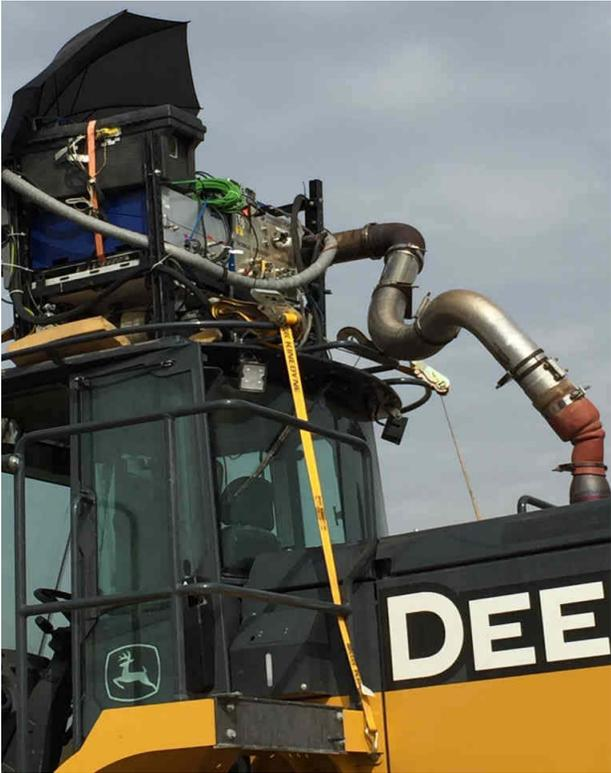
**Figure 2-11: Emission Equipment on JD 744KII Wheel Loader**
