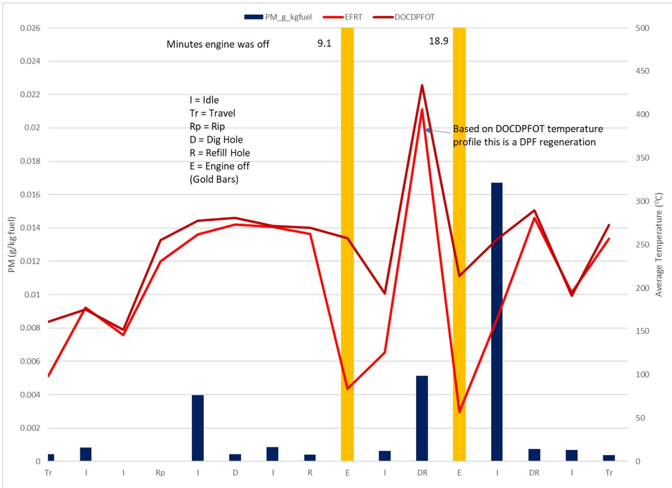
**Figure 4-8: Fuel based PM emissions by mode of operation for 2014 tier 4F John Deere 1050K Crawler Tractor**
