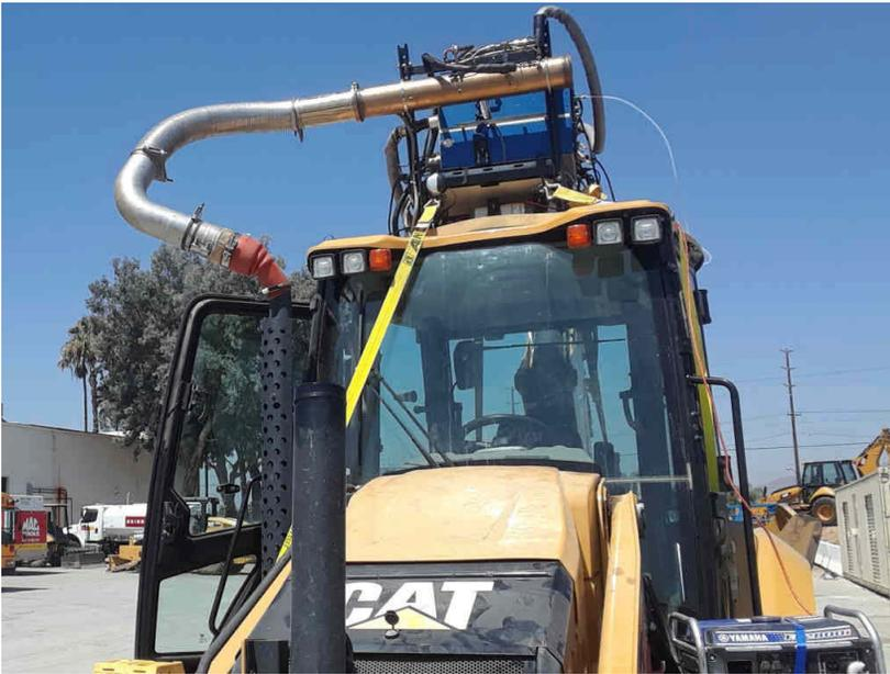
**Figure 2-9: Emission Equipment on CAT 430F2 Backhoe/Loader**
