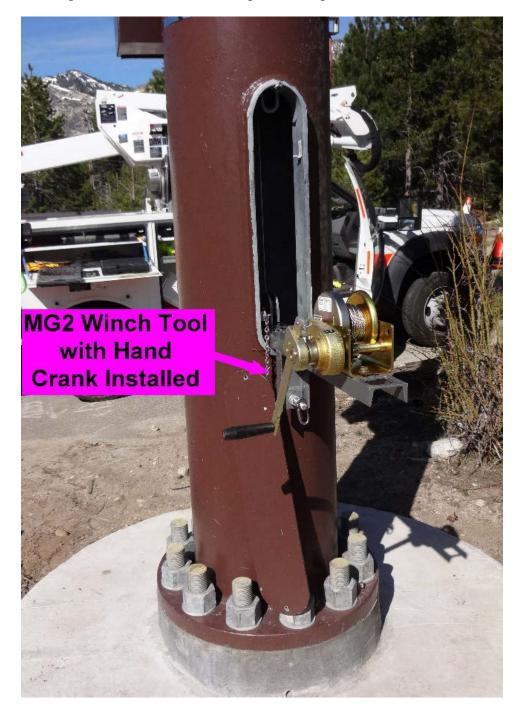
Figure 49. Meyers MG<sup>2</sup> Lowering Winch Tool
