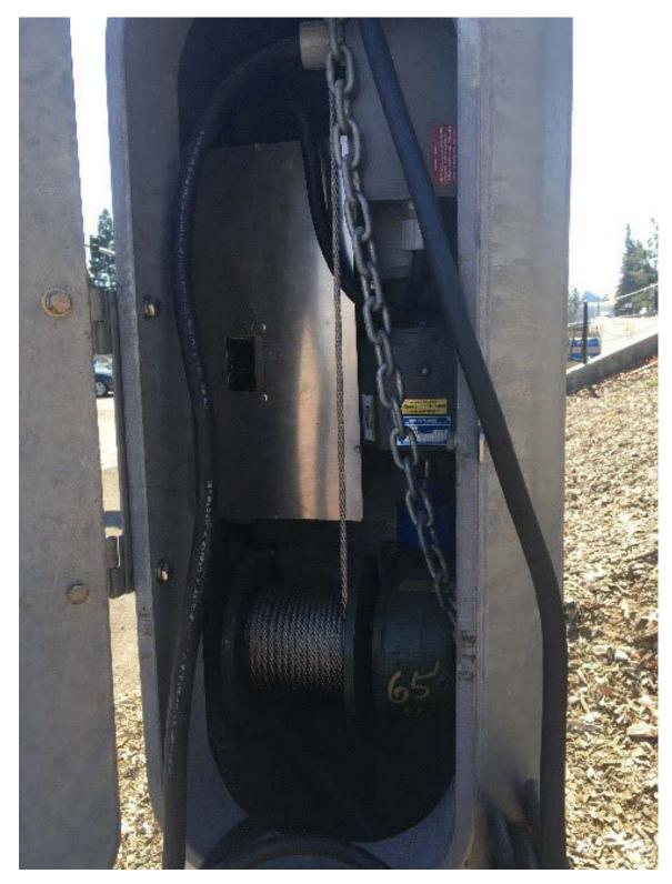
Figure 4. Stratus Internal Winch Tool with Integrated Electric Motor
