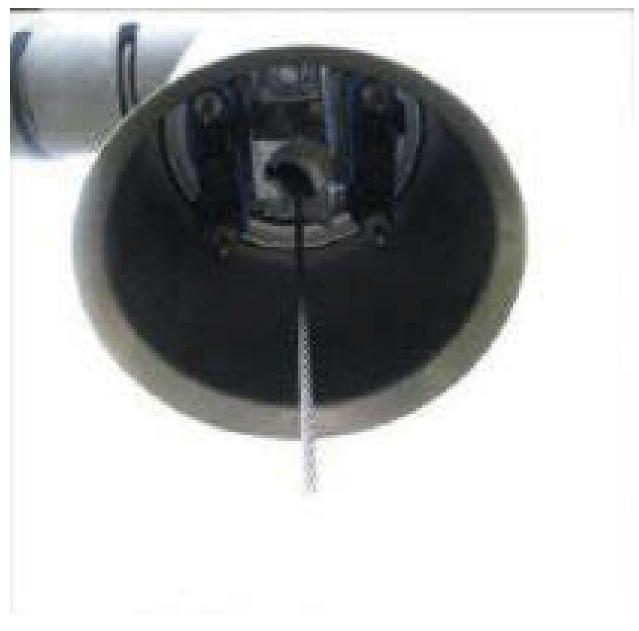
Figure 15. Camera Lowering Systems, Inc. Disconnect Top Half (Image courtesy of Camera Lowering Systems, Inc.)
