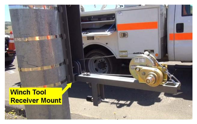
Figure 55. Winch Tool Receiver
