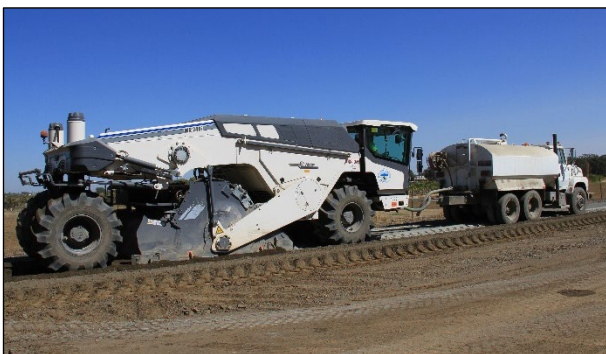
Figure 5.6: Water tanker and reclaimer.
