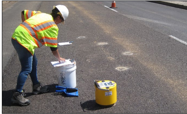
Figure 3.13: Soil stiffness gauge.
