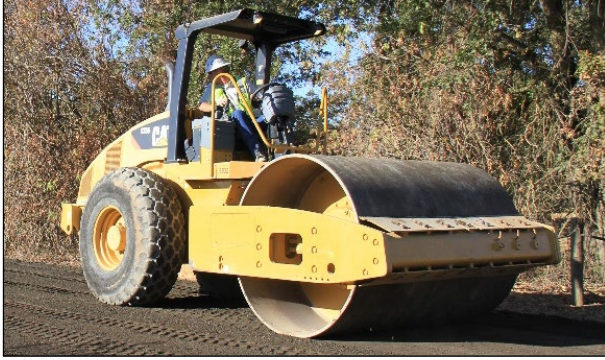
Figure 4.4: 12-ton SSR used for microcracking on FDR-C Test Road.
