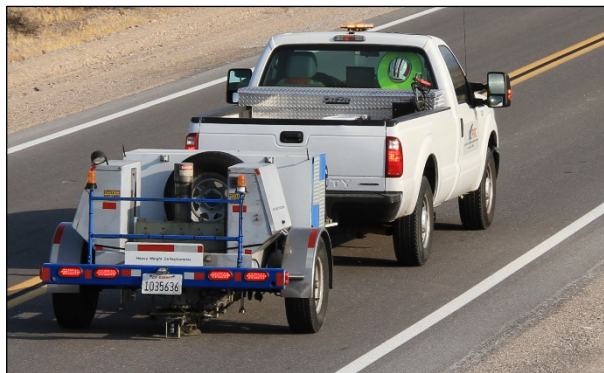
Figure 3.11: Falling weight deflectometer.
