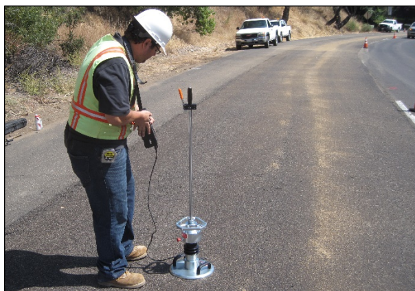
Figure 3.12: Light weight deflectometer.
