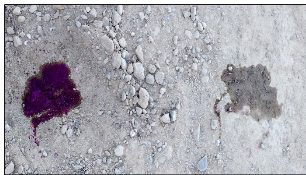
Figure 2.17: Carbonated area (no color in sprayed area) attributed to inappropriate curing.
