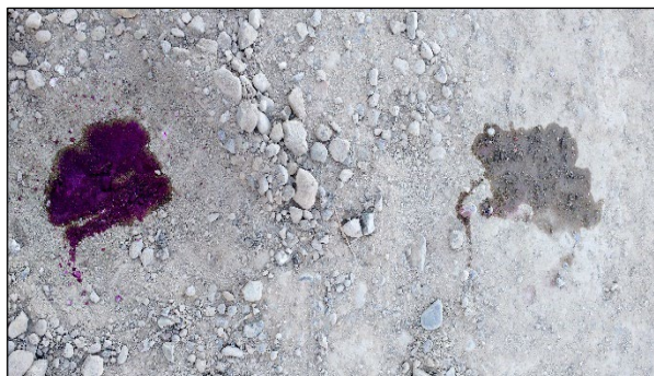
Figure 3.5: Surface carbonation on an FDR-C layer.
