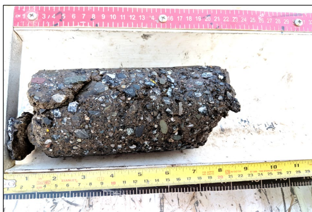
Figure 6.22: Core taken across shrinkage crack.
