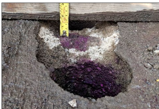
Figure 6.24: Carbonation extent beneath microsurfacing.
