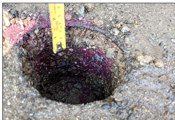
Figure 6.23: Carbonation with depth in core hole.
