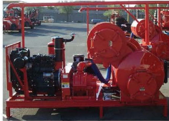
Figure 25. Crafcro™ Crack-Vac (Image Courtesy of Crafcro Inc.)
