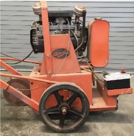
Figure 37. Conventional Router Engine Drivetrain and Encasement
