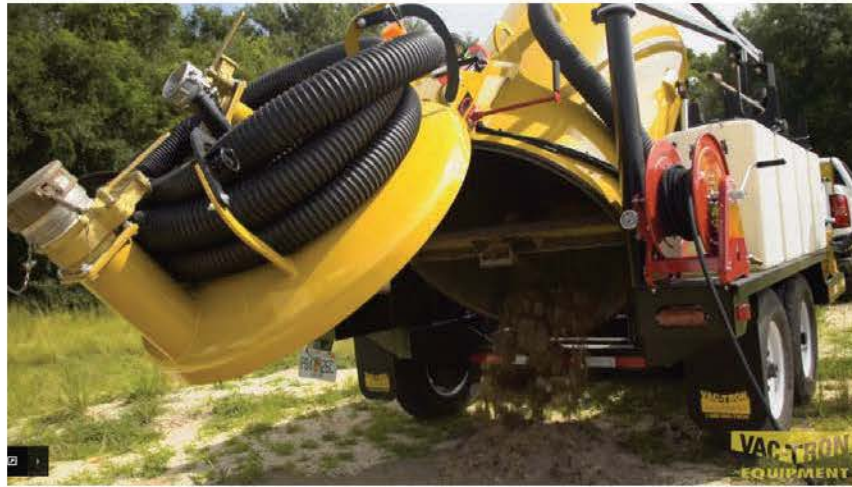
Figure 26. Vacuum Debris Off-Loading (Image courtesy of Vac-Tron)
