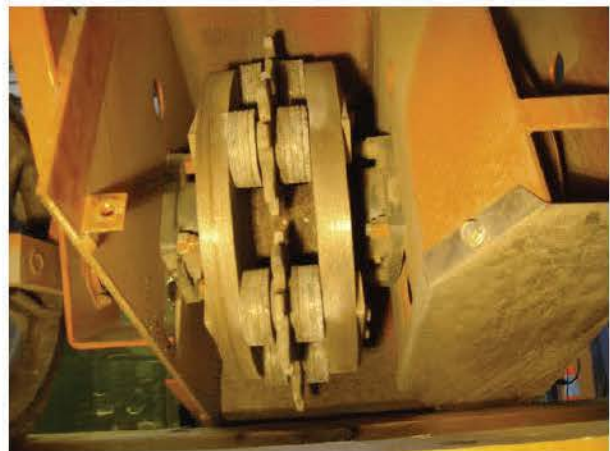
Figure 8. Standard Manual Impact Router for Joint Crack Cleaning
