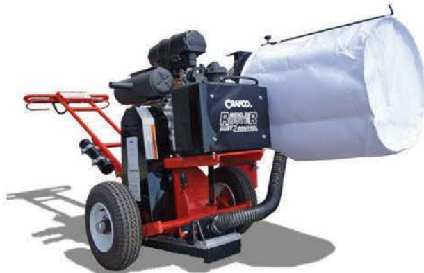
Figure 24. Crafcro™ Manual Router with Dust Control Option (Image Courtesy of Crafcro Inc.)
