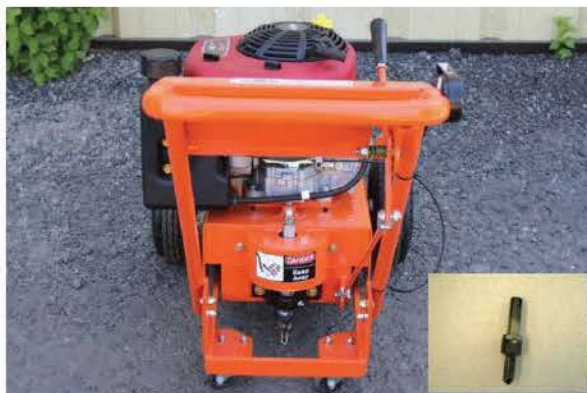
Figure 4. Pin Router (Courtesy of Salsco Inc.)
