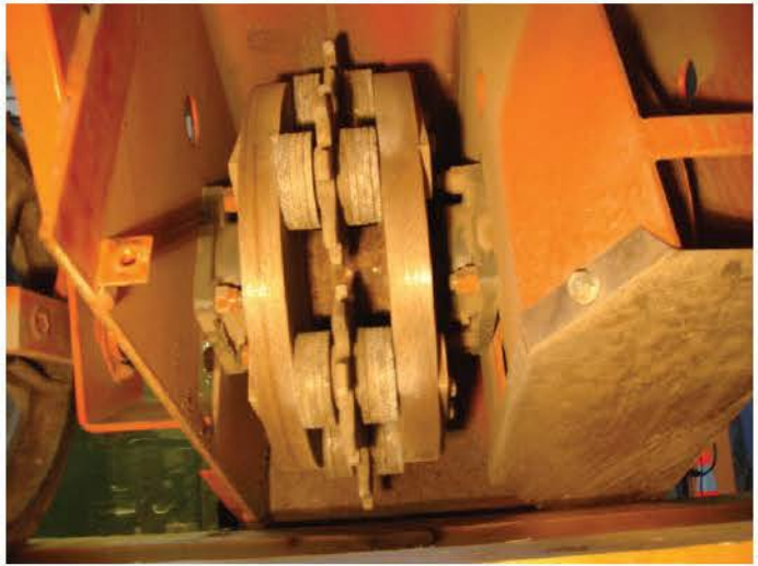
Figure 38. Conventional Router Wheel Linkage and Cutter Flywheel
