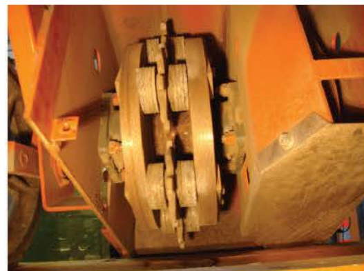
Figure 5. Impact Router Freewheeling Cutters
