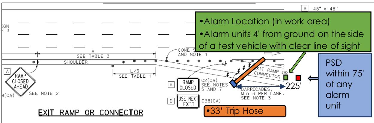
**Figure 6.4 Recommended Deployment Plan for Worker Alert System on a Standard Ramp Closure**
