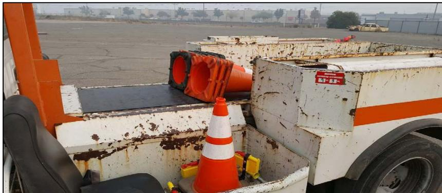
**Figure 4.9 Deploying a SonoBlaster Mounted Cone from a Standard Caltrans Cone Body Truck**
