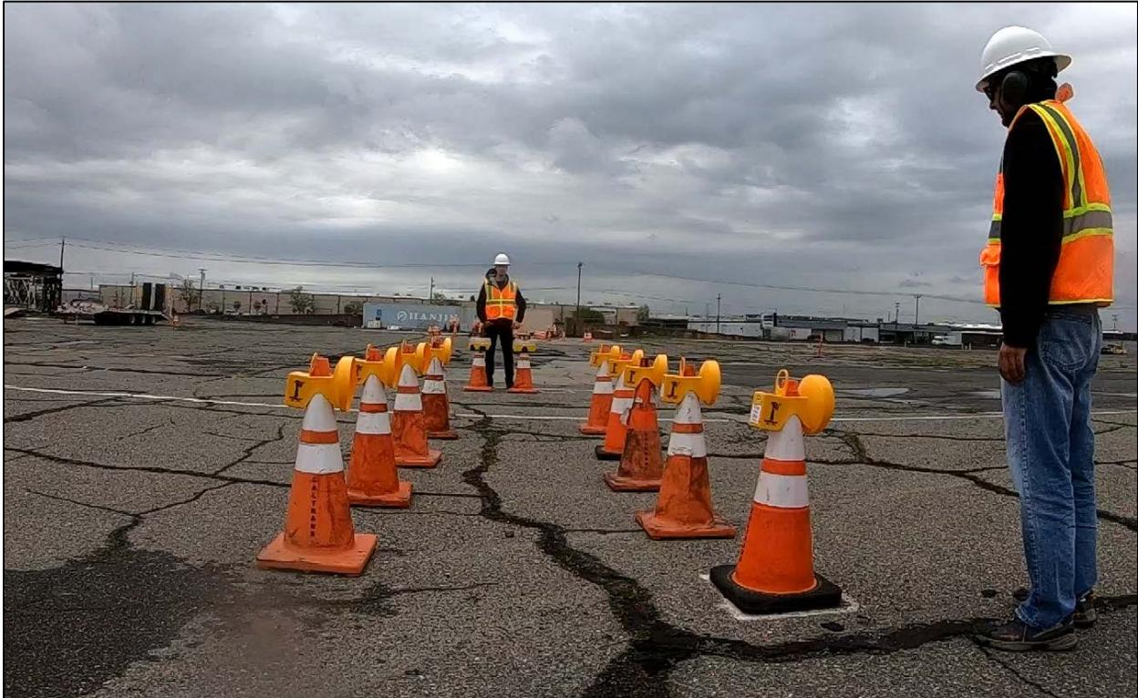
**Figure 5.3 Photo of Intellicone Lamp Sensitivity Tests Using High Speed Video**
