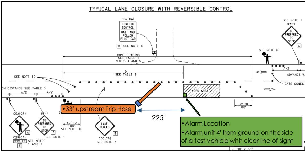
**Figure 6.1 Worker Alert System Layout for Reaction Time Calculations**
