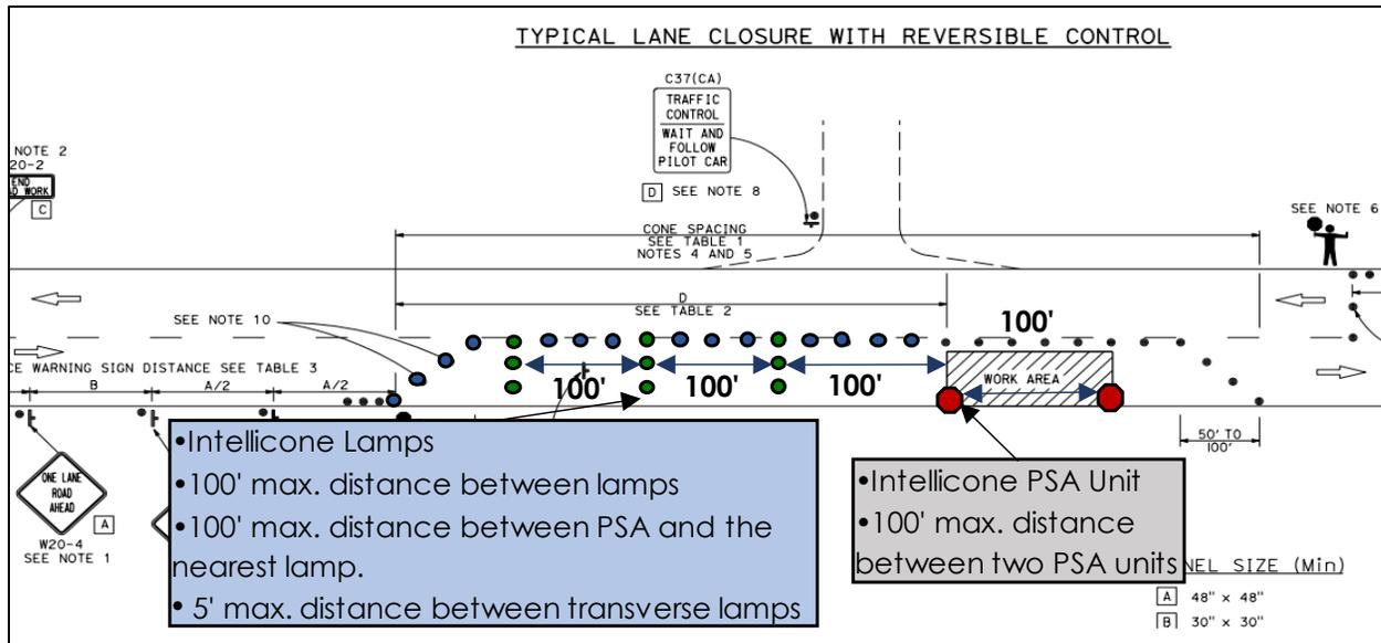
**Figure 6.5 Recommended Deployment Plan for Intellicone on a Standard T-13 Closure**
