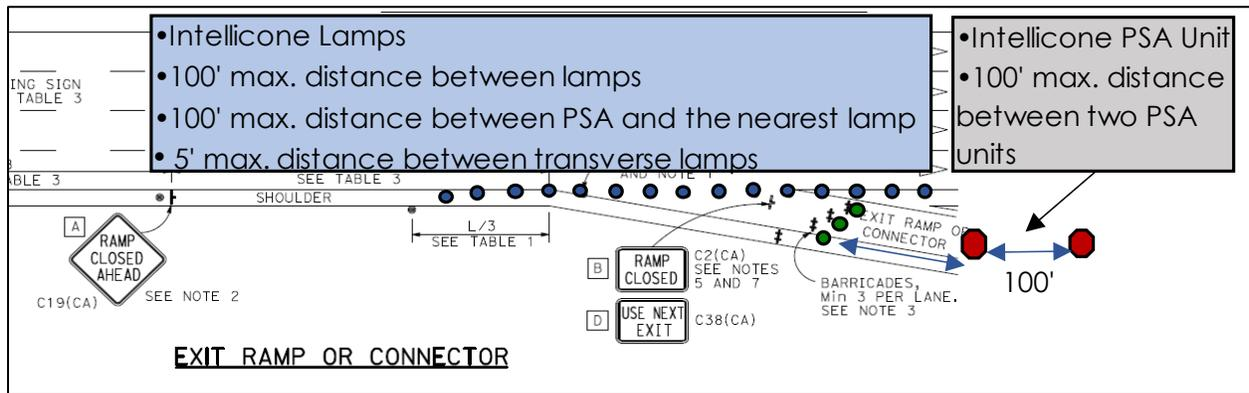
**Figure 6.6 Recommended Deployment Plan for Intellicone on a Standard Ramp Closure**
