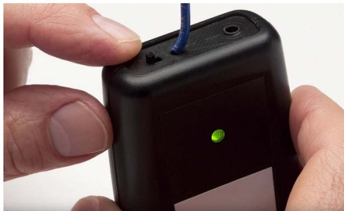
**Figure F.3 Turning on Personal Safety Device**
