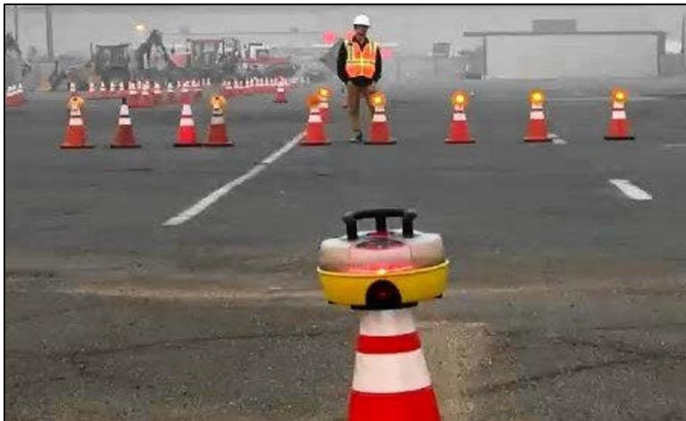
**Figure 4.15 Photo of Intellicone Operational and Lamp Sensitivity Test**
