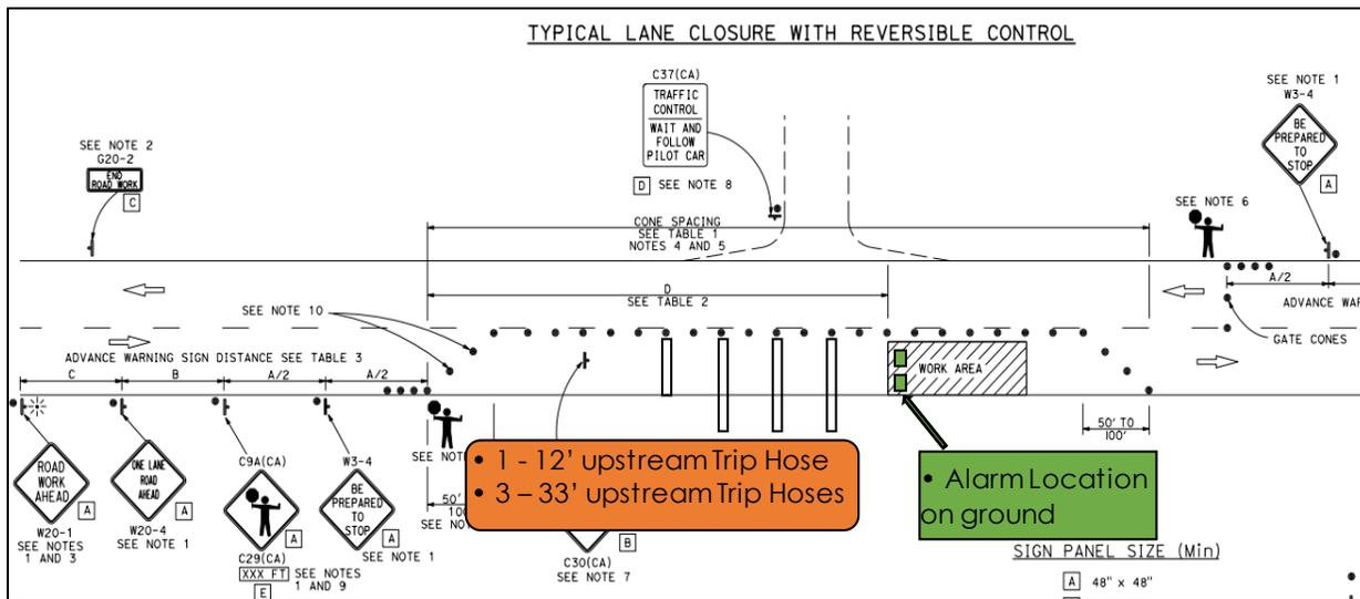
Figure 4.1 WAS Deployment Layout During Pilot Testing
