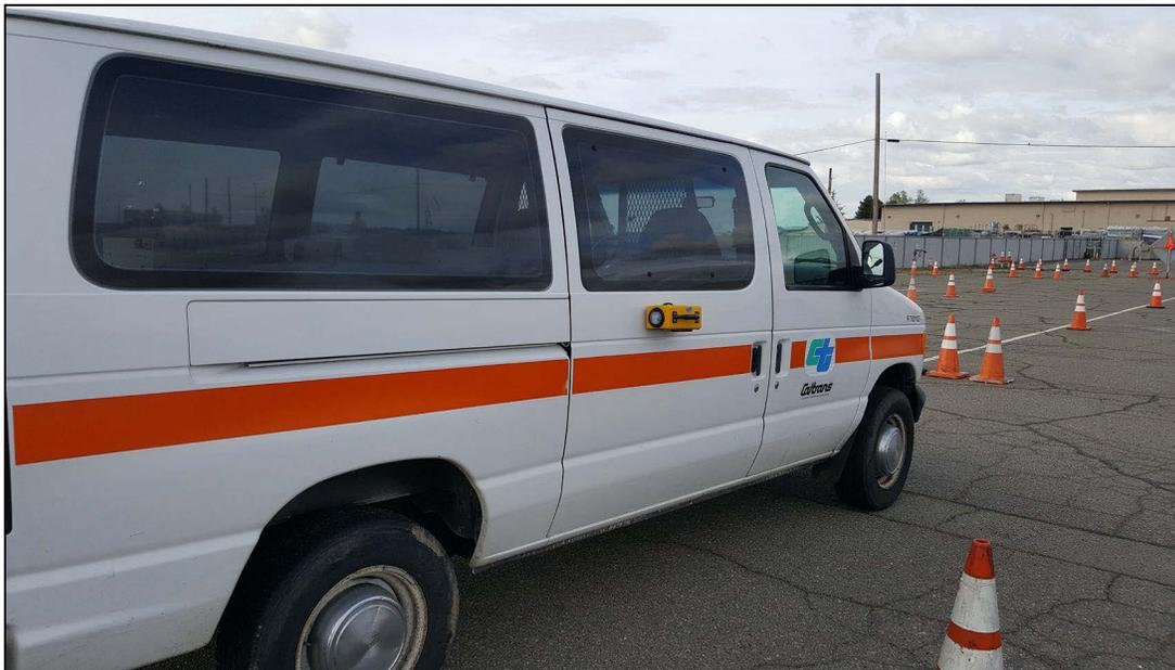
**Figure 5.1 WAS Alarm Unit Attached to a Vehicle in the Work Zone (4 Feet Above the Ground)**
