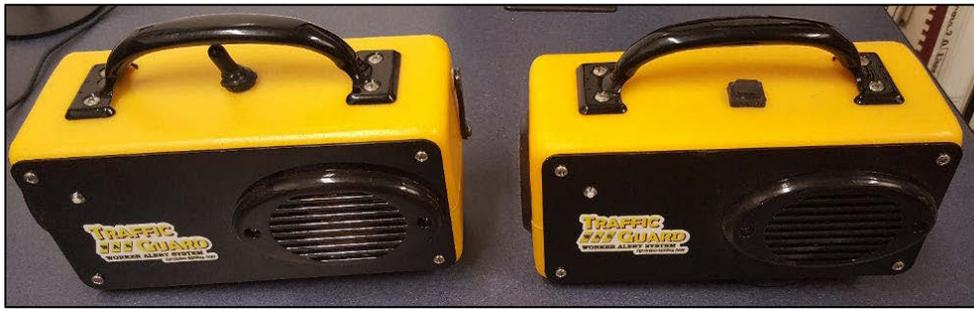
**Figure 3.1 Traffic Guard WAS RT Alarm Unit on the Left and CAL Unit on the Right**
