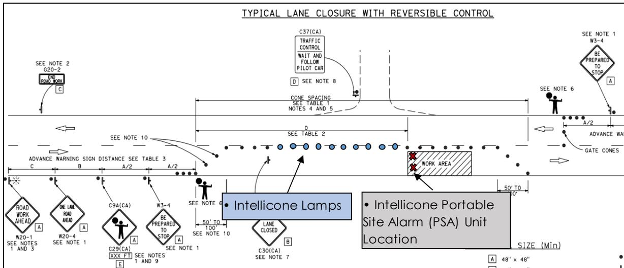
**Figure 4.13 Deployment Layout of Intellicone System Deployment during Pilot Testing**
