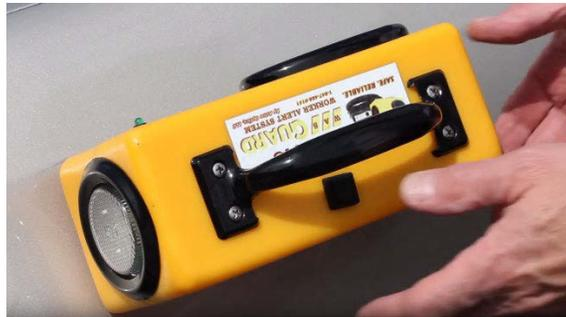
**Figure F.1 Turning on Horn/Light Alarm**
