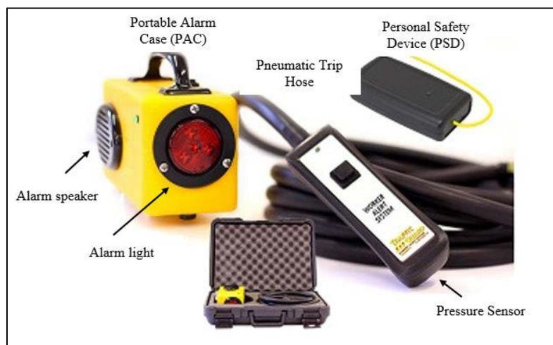
**Figure 2.1 Traffic Guard Worker Alert System Components**
