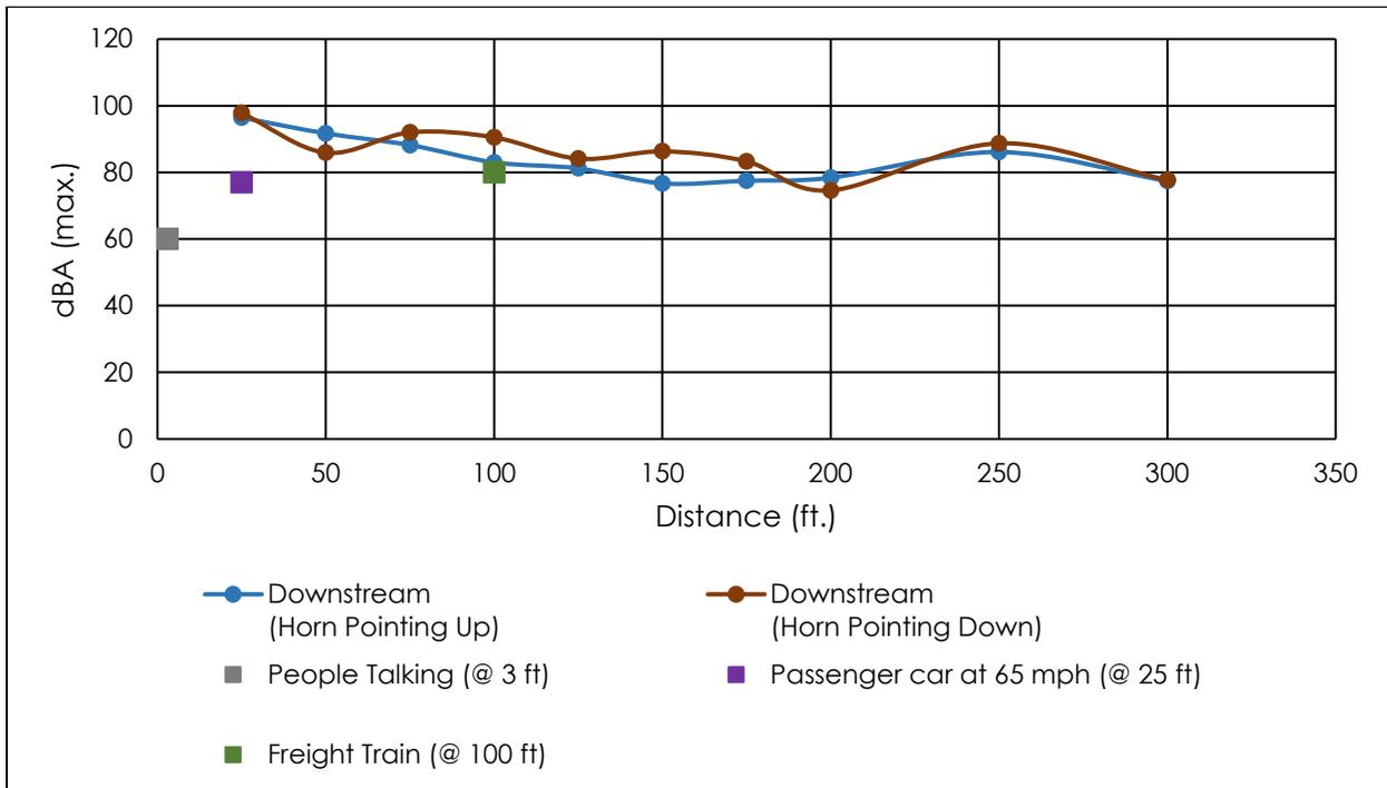
**Figure 4.11 SonoBlaster Sound Level Measurements Downstream of Work Area**
