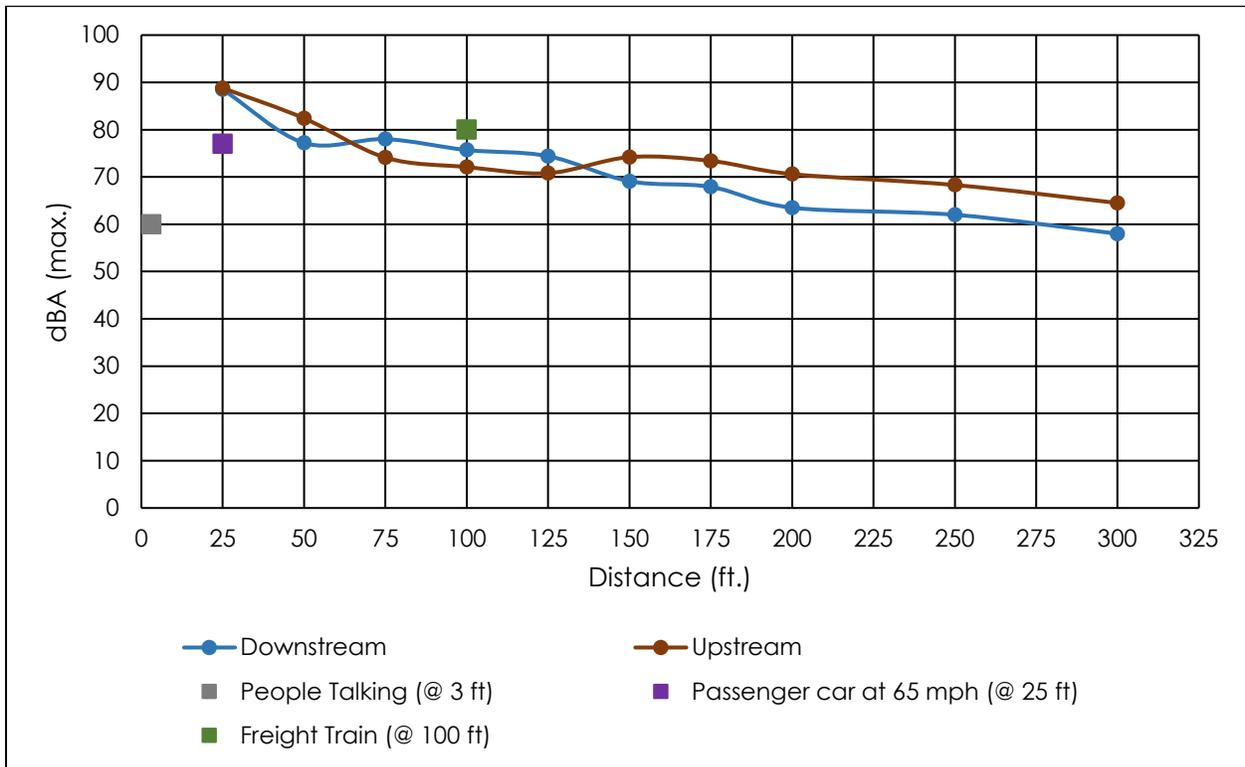
**Figure 4.14 Sound Level Measurements Upstream and Downstream of Work Area for Intellicone**
