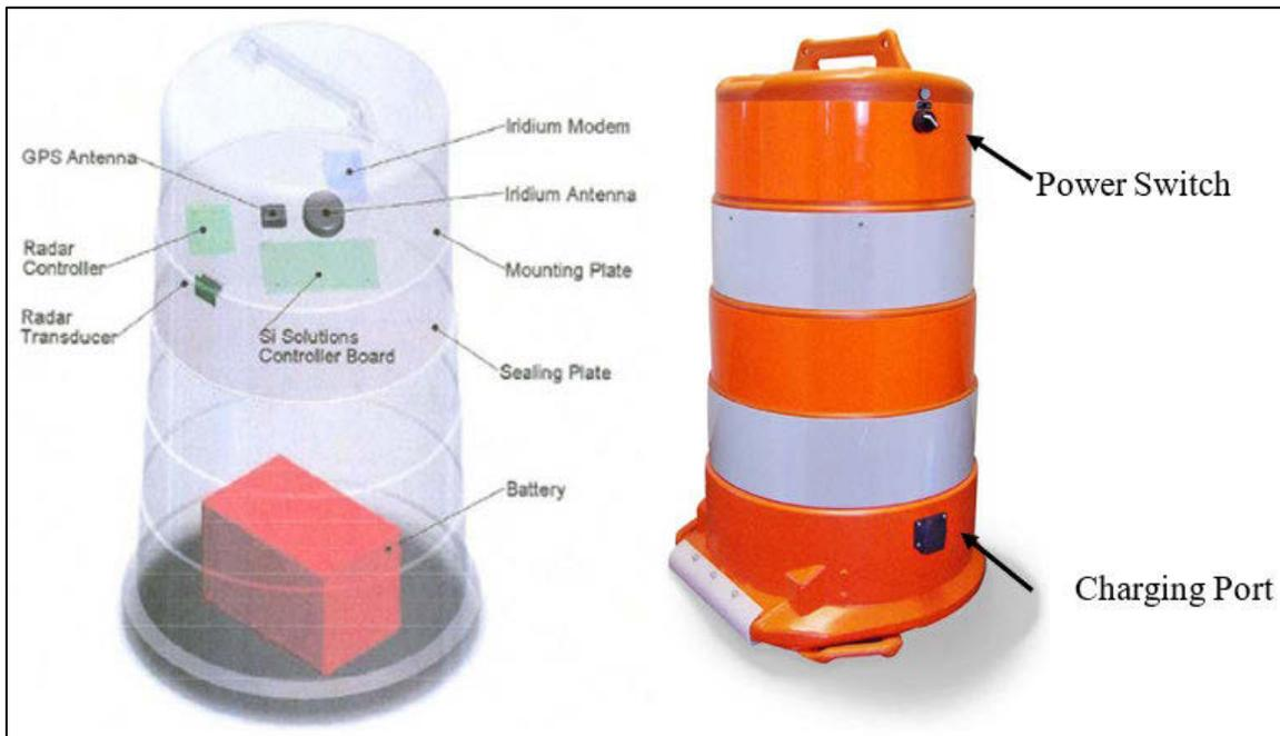
**Figure A.3 iCone System - Interior and Exterior**
