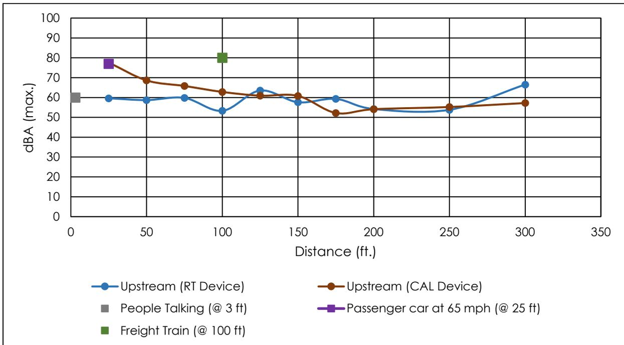
**Figure 4.5 WAS Sound Level Measurements Upstream of Work Area**
