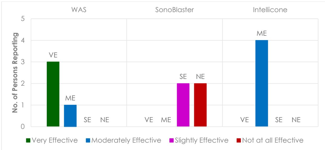
**Figure 5.6 Effectiveness of WZIA Devices in Mitigating Work Zone Collisions**
