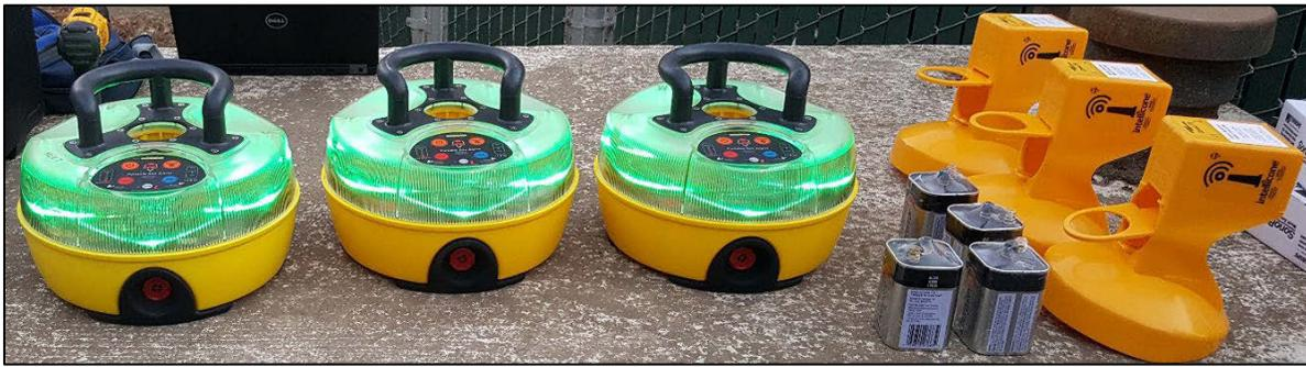
**Figure 3.2 Intellicone System PSA and Lamps**
