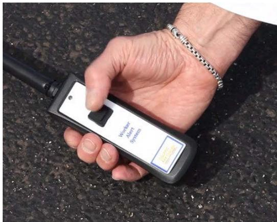
**Figure F.2 Turning on the Pressure Sensor**
