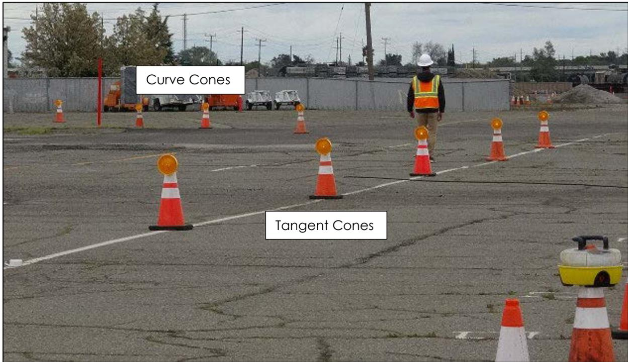
**Figure 5.4 Photo of Intellicone Operation Tests with Lamps Deployed on a Tangent-Curve Combination**
