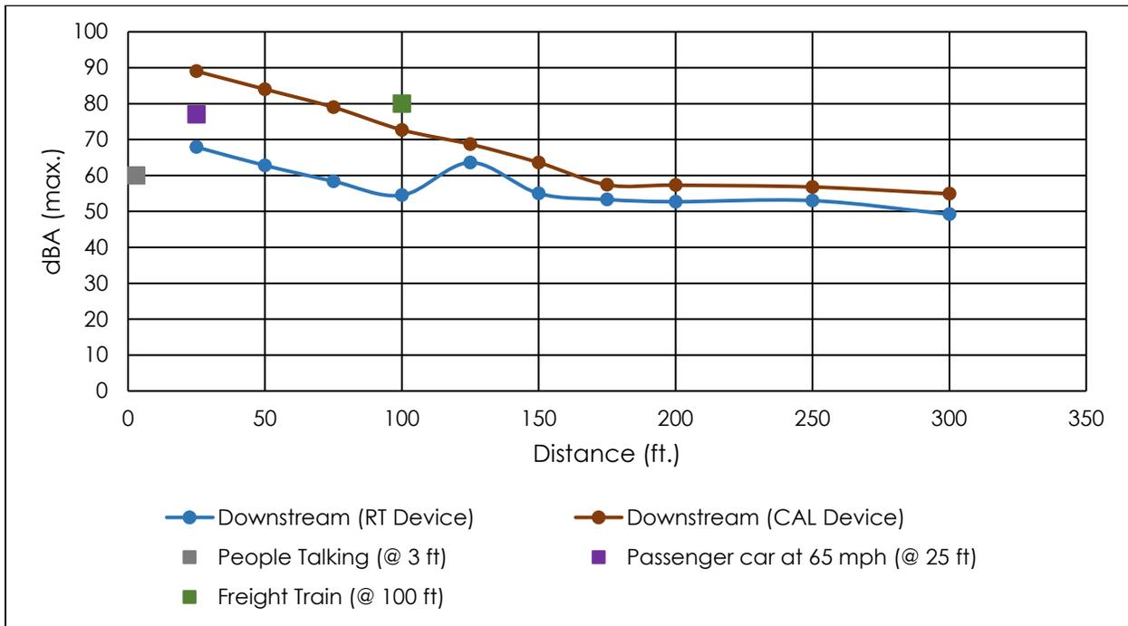
**Figure 4.4 WAS Sound Level Measurements Downstream of Work Area**
