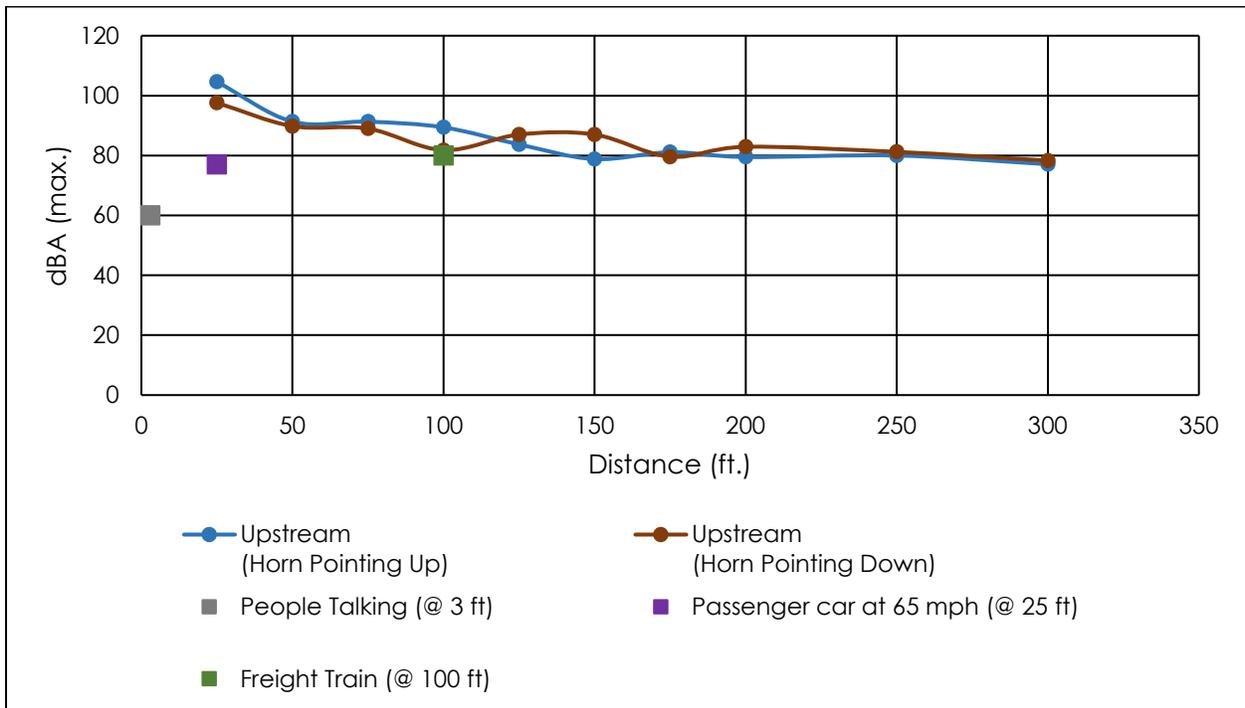
**Figure 4.12 SonoBlaster Sound Level Measurements Upstream of Work Area**
