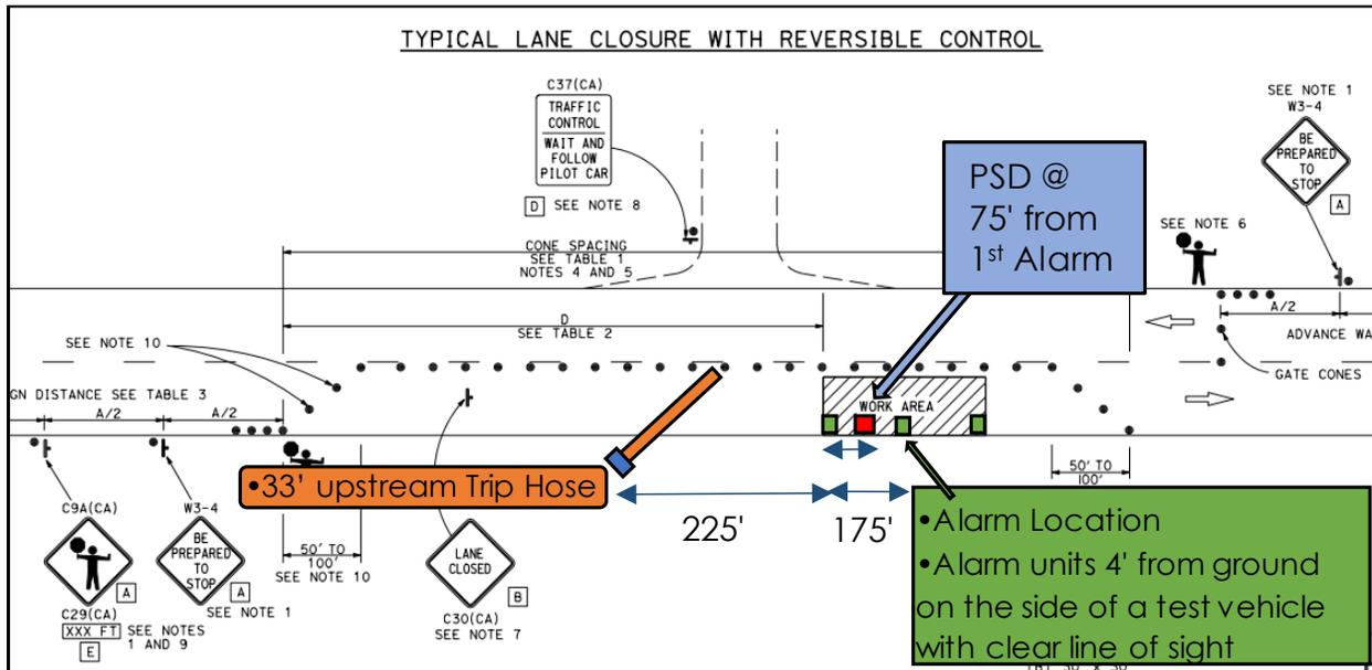
**Figure 5.2 Deployment Layout of WAS Range Tests during Supplemental Testing**
