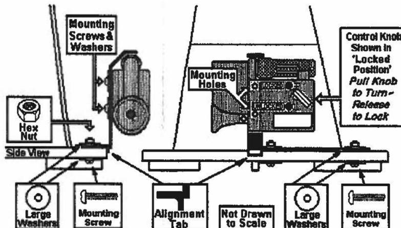
Figure F.5 SonoBlaster Bracket Assembly
