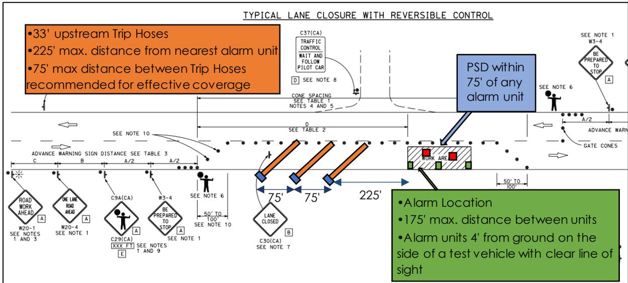
**Figure 6.3 Recommended Deployment Plan for Worker Alert System on a Standard T-13 Closure**
