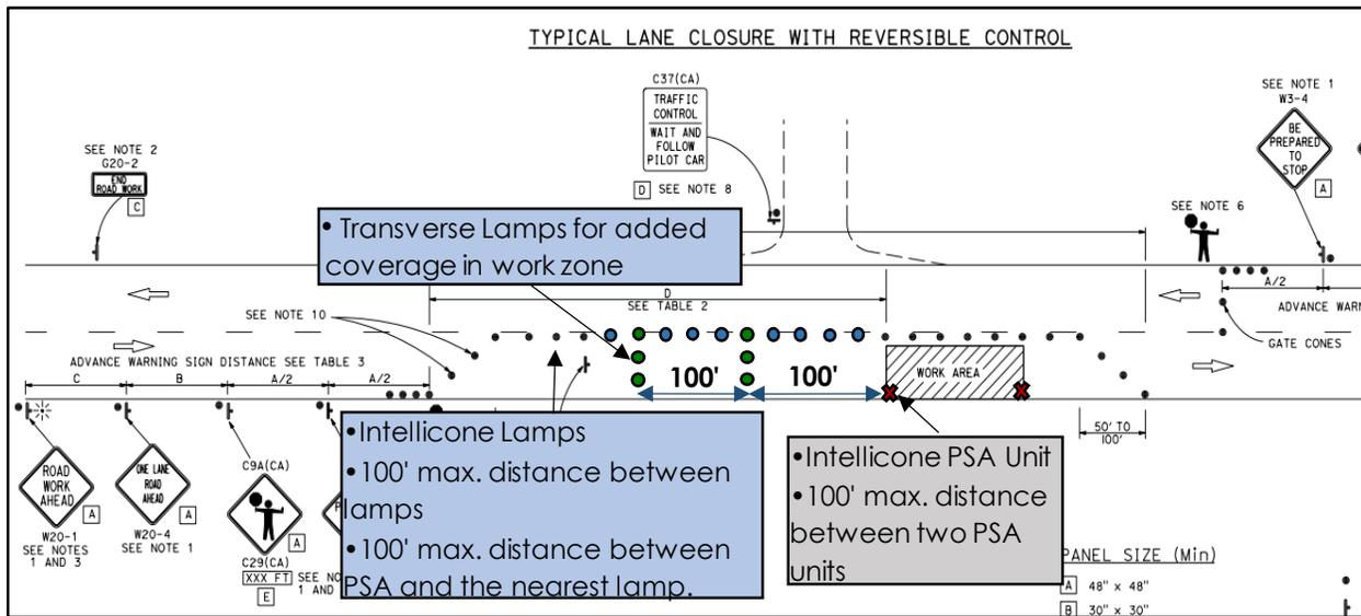
**Figure 6.2 Intellicone System Layout for Reaction Time Calculations**
