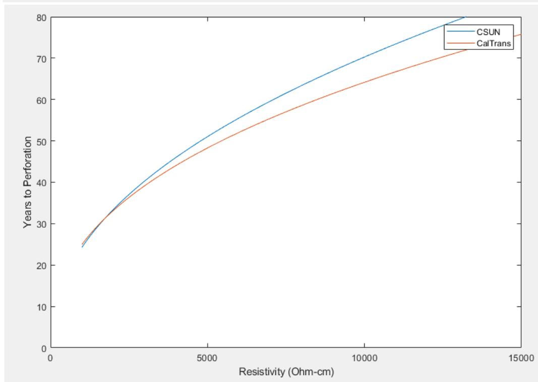
**Fig. 6.8** Years vs. Resistivity with a constant pH of 7.5 at 15% failure criteria (top) and 25% failure criteria (bottom) \*
