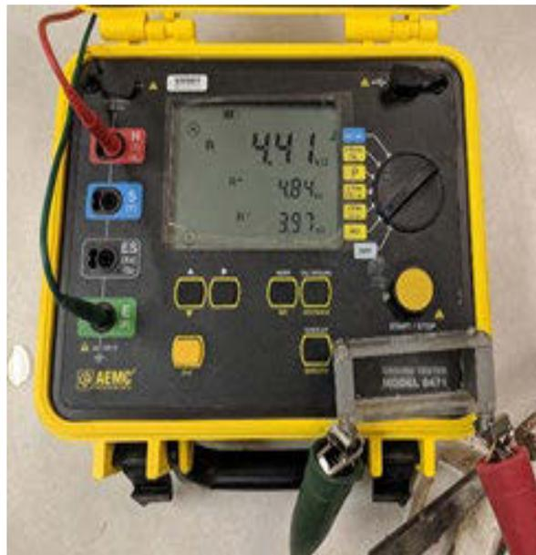
**Fig. 4.1** Small soil resistivity box and meter
