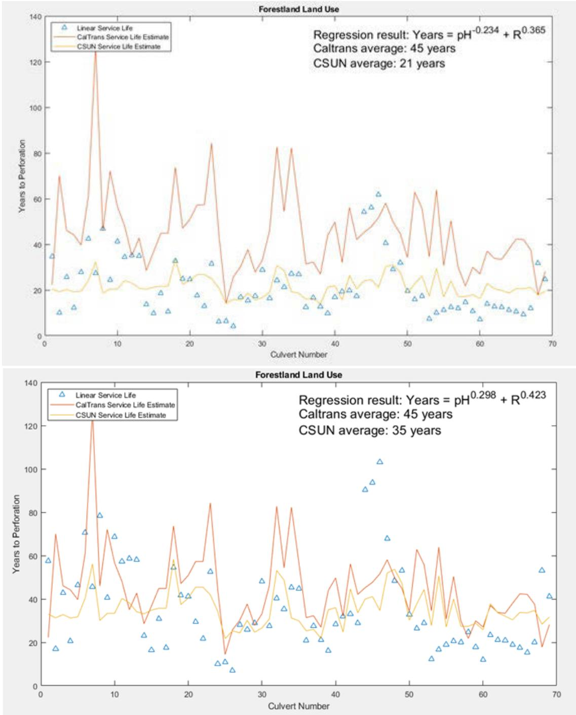
**Fig. 6.5** Comparison of Caltrans and CSUN service life equations for Forestland regions at 15% failure criteria (top) and 25% failure criteria (bottom) \*
