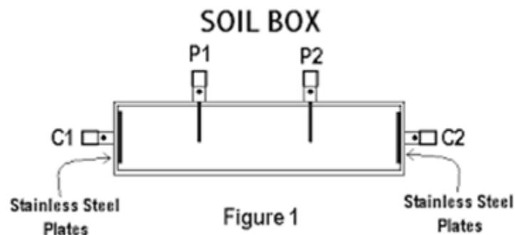
**Fig. 1.3** Design of the 4-connection soil box (Florida Department of Transportation)
