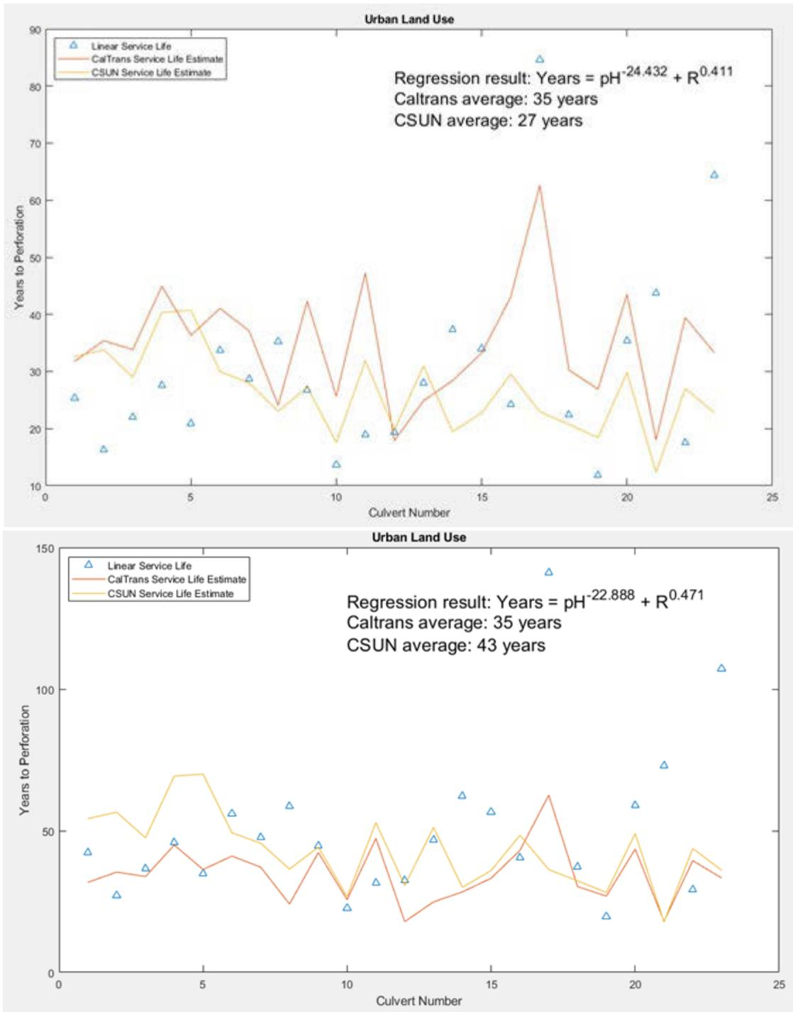
**Fig. 6.7** Comparison of Caltrans and CSUN service life equations for Urban regions at 15% failure criteria (top) and 25% failure criteria (bottom) \*
