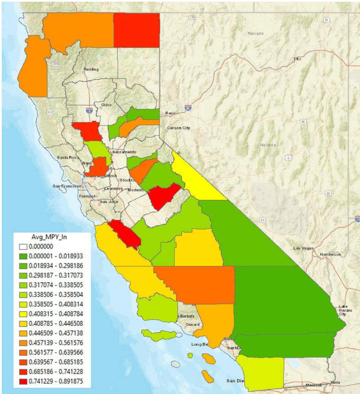
Fig. 5.7 Corrosion map of California measured in milli-inches per year
