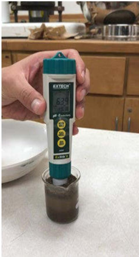
**Fig. 4.2** ExStik II reading soil data
