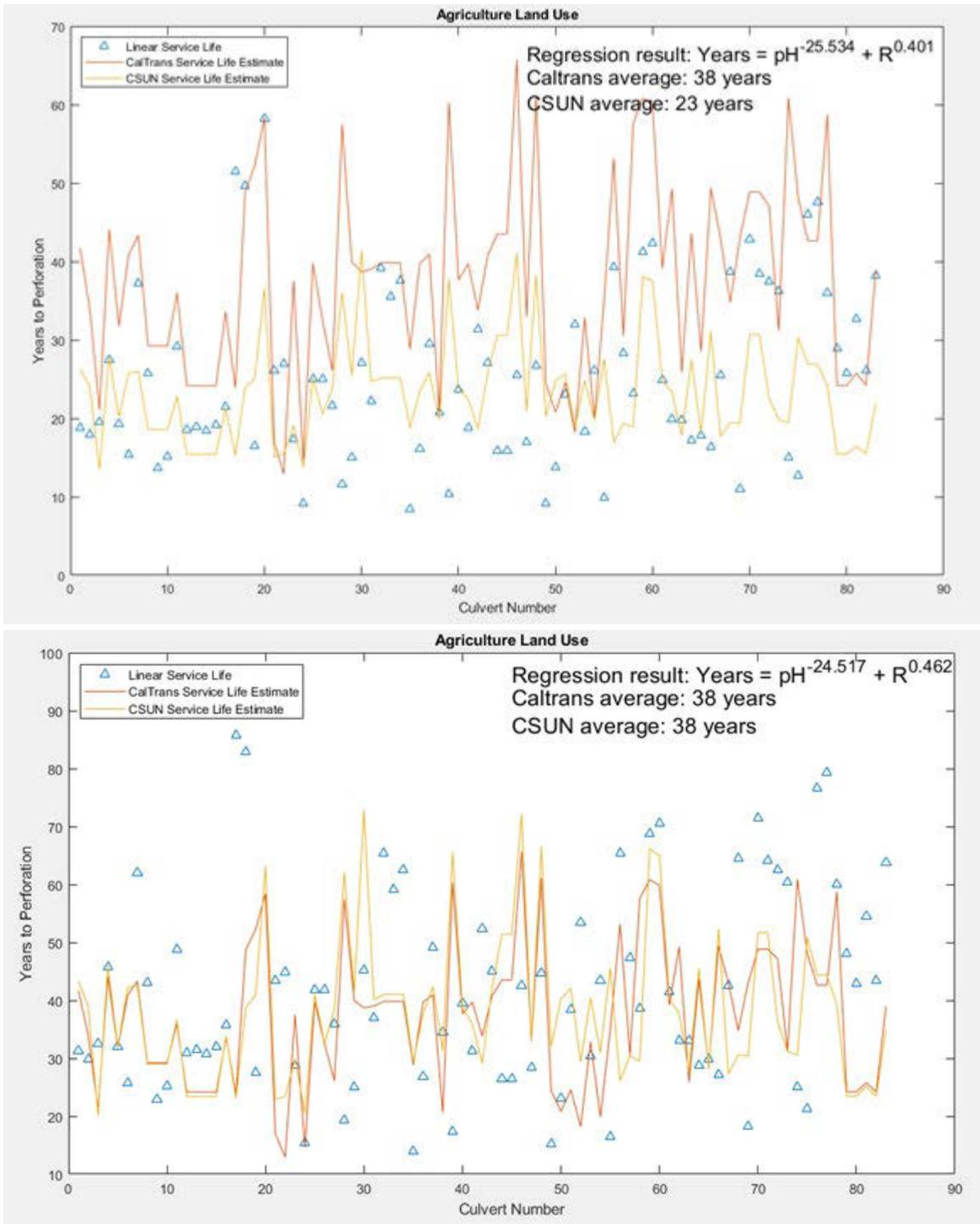
**Fig. 6.3** Comparison of Caltrans and CSUN service life equations for Agriculture regions at 15% failure criteria (top) and 25% failure criteria (bottom) \*
