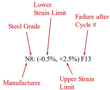
**Figure 5.13. Coding System for Identifying Test Bars**
