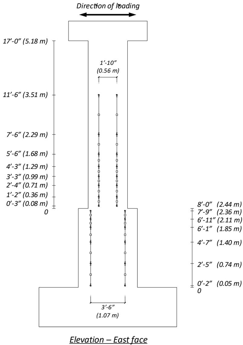
**Figure 3.14. Linear Potentiometers Along Height of Test Specimen**
