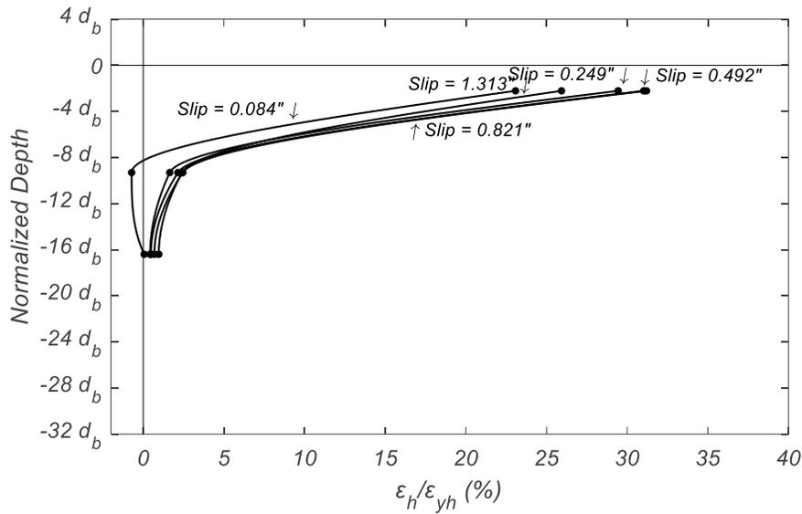
**Figure 2.24. Transverse Hoop Strain Profile in Specimen #3**
