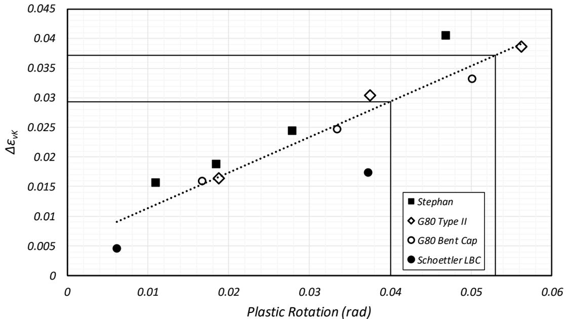
**Figure 5.35. von Karman Strain Amplitude vs Plastic Rotation from Experimental Data**
