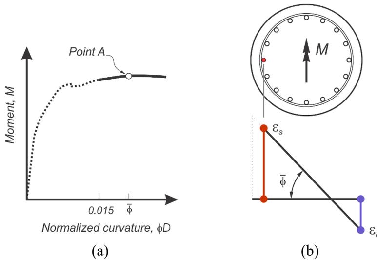
**Figure 3.38. Smear-Strain Compatible Method for Equivalent Plastic Hinge Length: (a) Domain Used in the Theoretical Moment-Curvature Response; (b) Section Strain Profile at Point "A" (Duck et al., 2018)**
