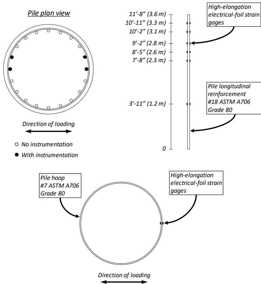
**Figure 3.13. Representative Pile Longitudinal and Transverse Reinforcement Instrumentation**
