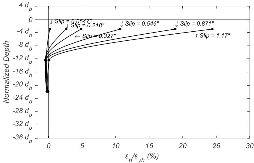
**Figure 2.28. Transverse Hoop Strain Profile in Specimen #4**
