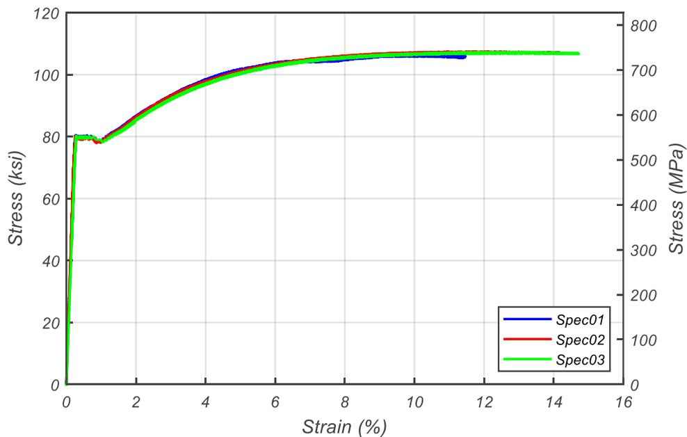
**Figure 5.9. Smoothed-Rib-Radii #14 ASTM A706 Grade 80 Tensile Test Data**
