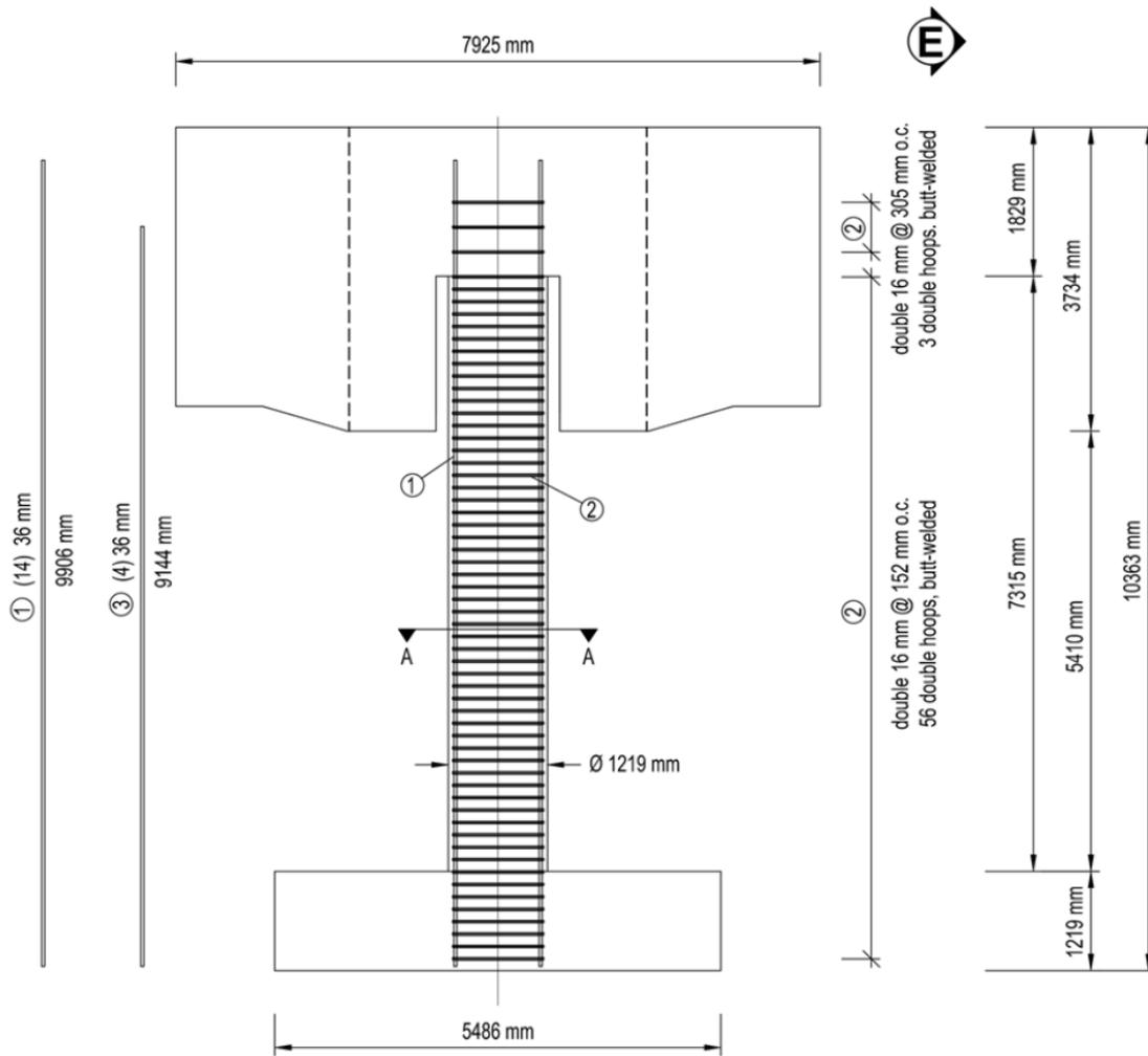
**Figure 3.47. Large Bridge Column (L.B.C.) Test Specimen from Schoettler et al.,
