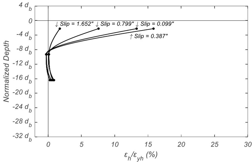
**Figure 2.16. Transverse Hoop Strain Profile in Specimen #1**
