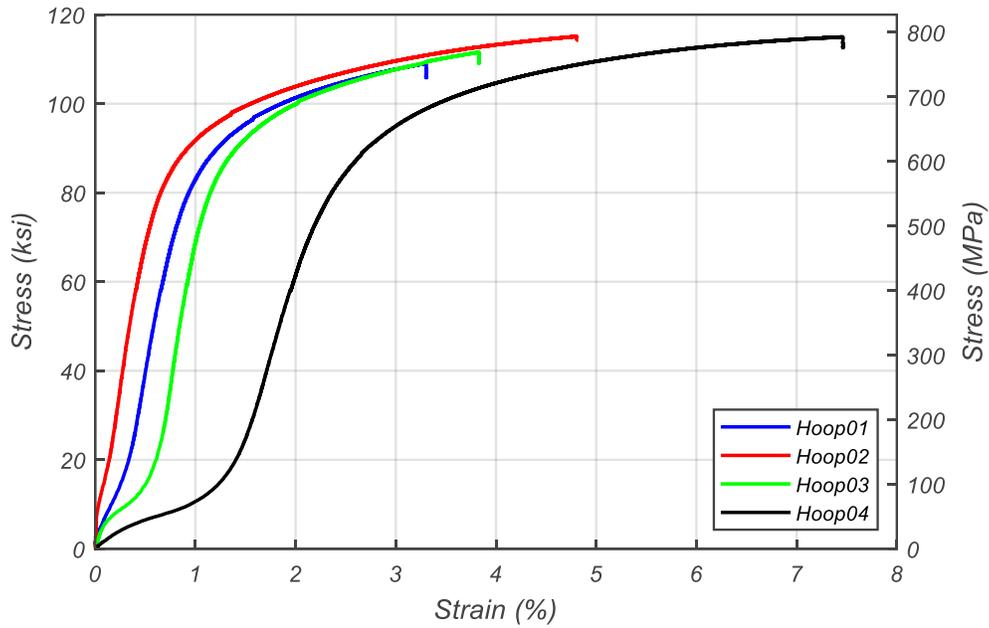
**Figure 3.5. Butt-Welded Column Hoop Validation Tensile Tests**
