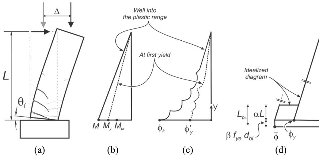
**Figure 3.37. Smear-Strain Compatible Method for Equivalent Plastic Hinge Length: (a) Deformed Column; (b) Bending Moment Diagram; (c) Curvature Diagram; (d) Idealized Curvature Diagram (Duck et al., 2018)**
