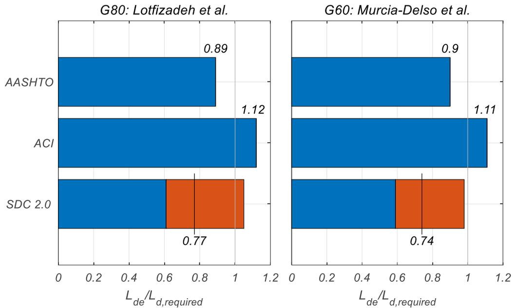
**Figure 3.9. Comparison of Column Longitudinal Bar Embedment Length**
