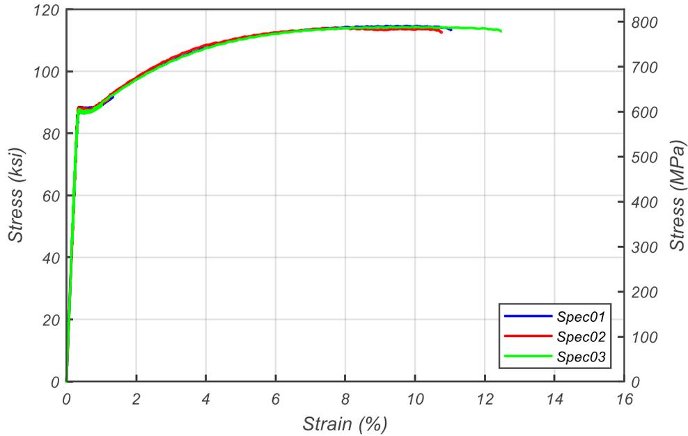
**Figure 5.8. Normal #14 ASTM A706 Grade 80 Tensile Test Data**
