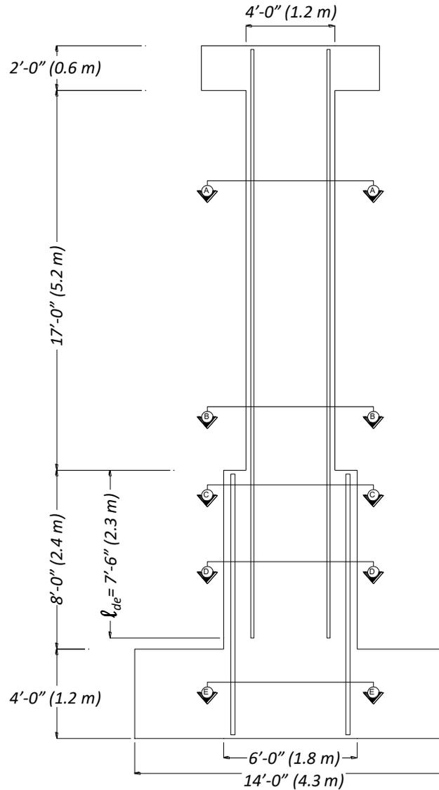
**Figure 3.3. General Dimensions of Test Specimen (Elevation View)**
