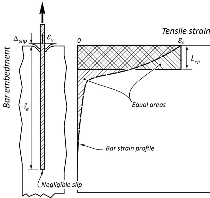
**Figure 2.31. Visual Representation of Equivalent Yield Penetration**
