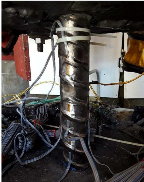
**Figure 5.12. Electrical-Foil Strain Gages Applied to Test Bar**
