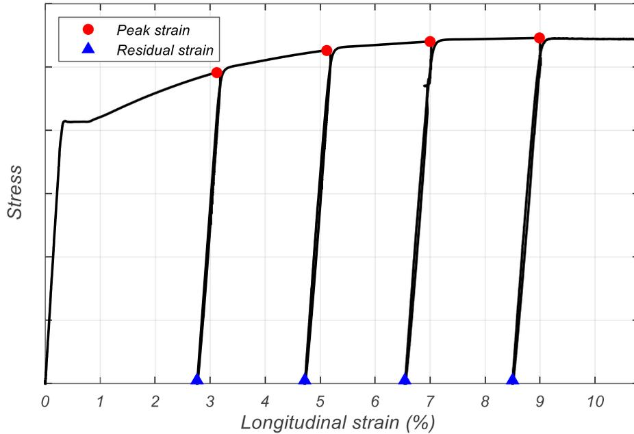
**Figure 2.8. Loading Scheme for Virgin Bar Tests**
