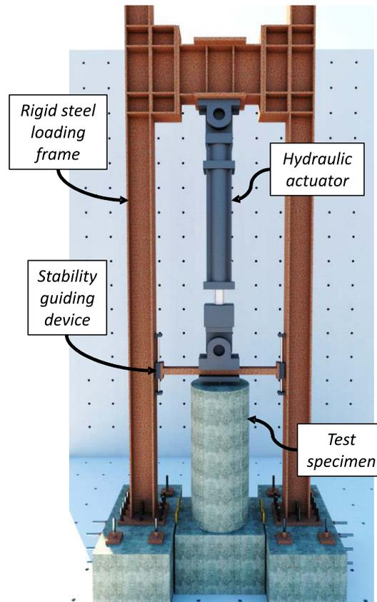
**Figure 2.5. 3D Rendering of Test Setup**
