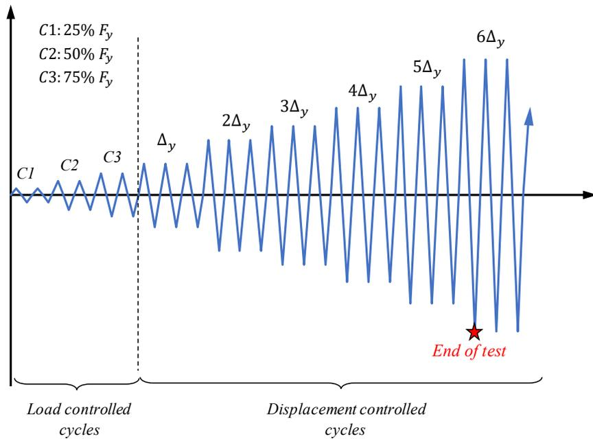
**Figure 4.12. Test Specimen Loading Protocol**
