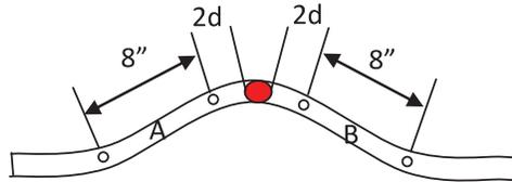
**Figure 2.4. California Test 670 Hoop Weld Validation Sample (California Test 670)**
