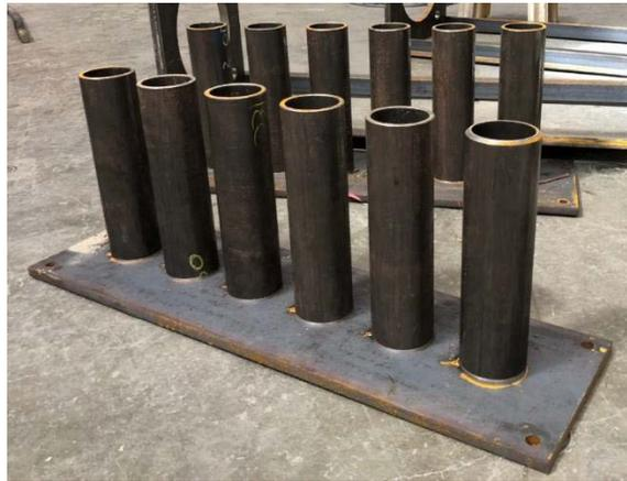
**Figure 4.2. Built-Up Steel Guide for Hinge at Column Base**
