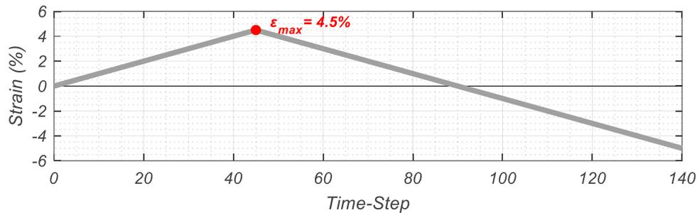
**Figure 5.25. Loading Protocol Strain History for FE Analysis**
