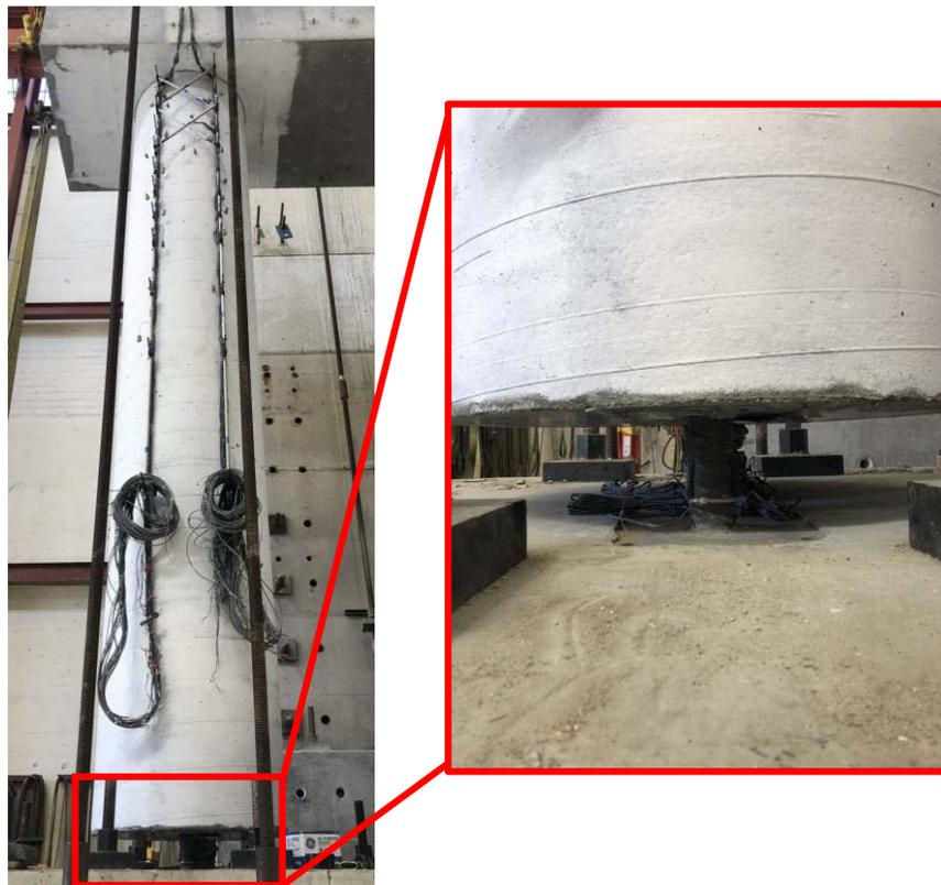
**Figure 4.3. Proprietary Hinge at Column Base**
