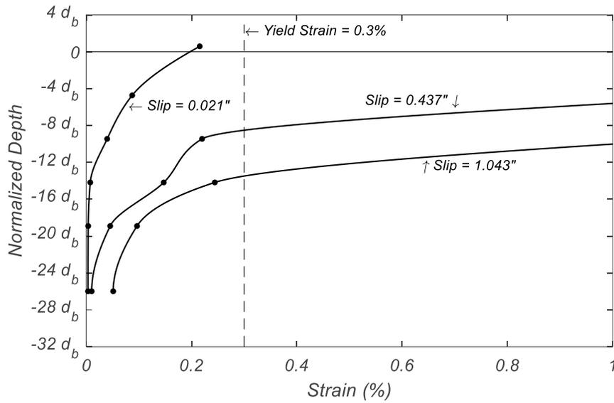
**Figure 2.20. Transverse Hoop Strain Profile in Specimen #2**
