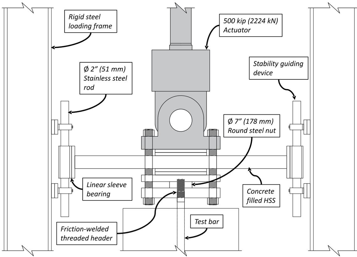
**Figure 2.6. Actuator-Test Bar Connection with Stability Guiding Device**
