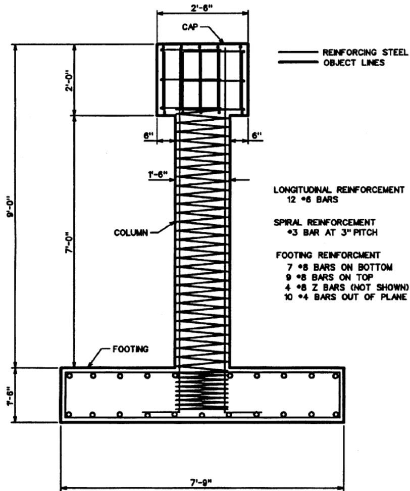
**Figure 5.37. Typical Test Specimen Dimensions and Reinforcement Layout (Moyer & Kowalsky, 2003)**
