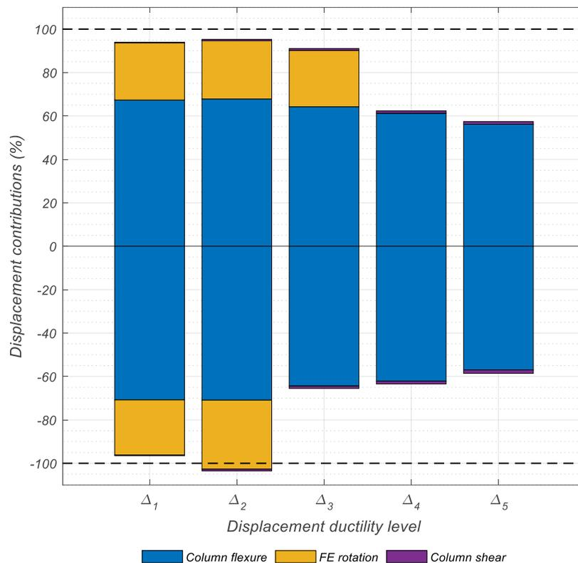
**Figure 4.30. Components of Lateral Displacement at Peak Displacement Ductility Levels**
