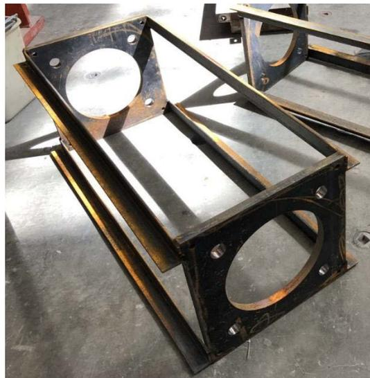
**Figure 4.11. Steel Loading Frame to Evenly Transfer Lateral Loads into Cap Beam**
