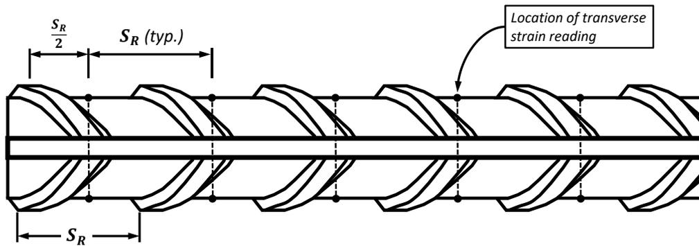
**Figure 2.7. Consistent Measurement Location Between Deformations on Bar**
