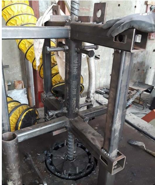
**Figure 5.11. Test Bar Embedded in Upper Pipe Grip Using the Aligning Steel Frame**
