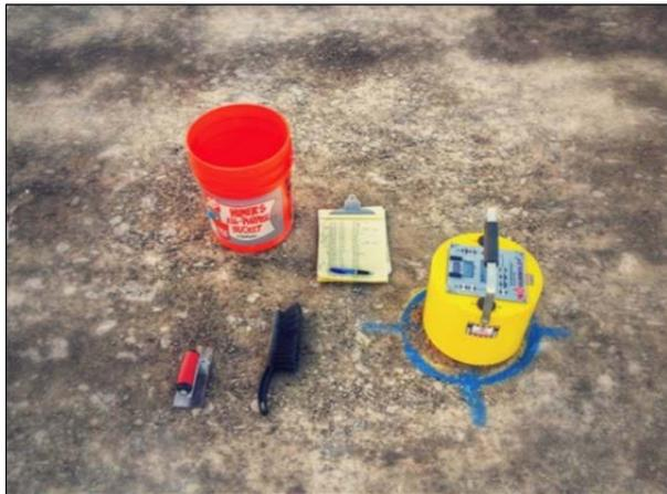
Figure 3.3: Soil stiffness gauge.
