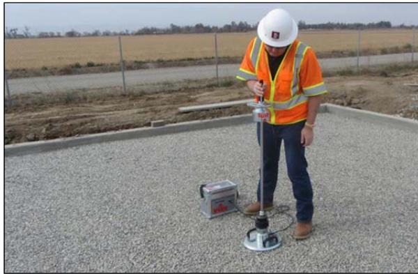
**Figure 3.2: Light weight deflectometer.**
