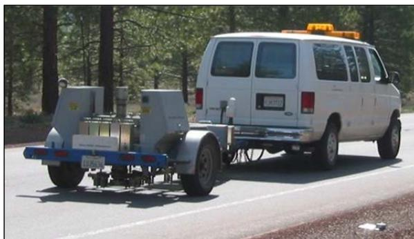
**Figure 3.1: Falling weight deflectometer.**
