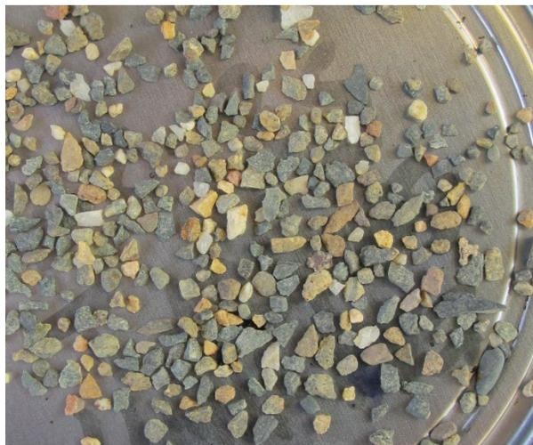
**(b) #16 sieve from ASTM concrete sand bin**
