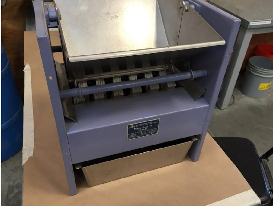
**Figure A.5: Small sample splitter.**
