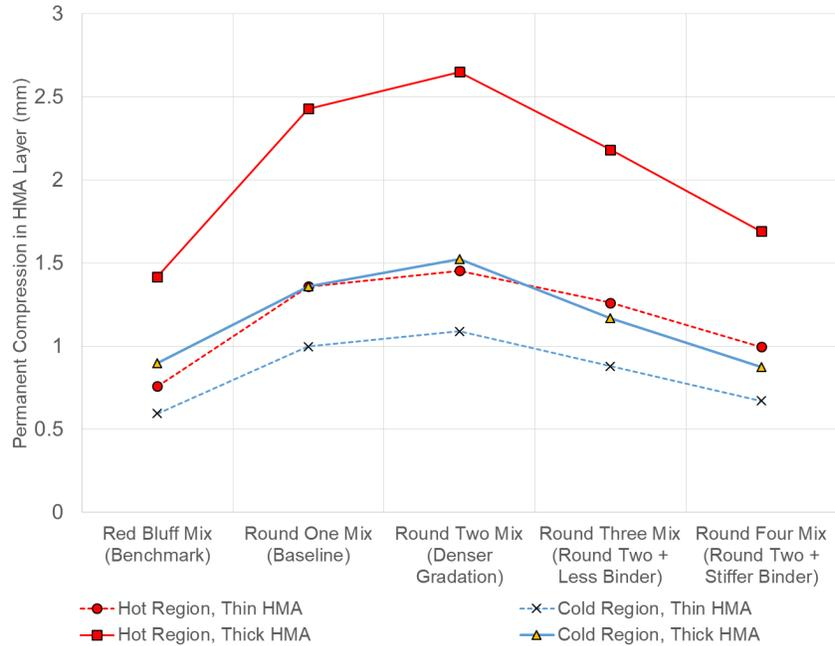
**Figure 8.3: Comparison of permanent compression in HMA layer.**
