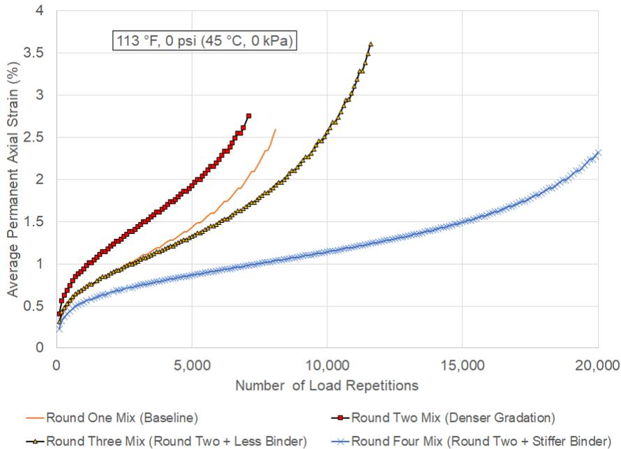
**Figure 7.10: Comparison of permanent axial strain accumulation curves of the Round One to Round Four mixes tested under 113°F (45°C) with no confinement.**
