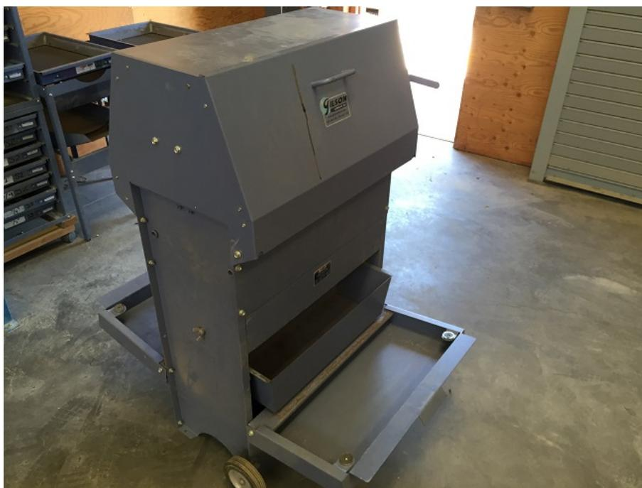
**Figure A.4: Large enclosed sample splitter.**
