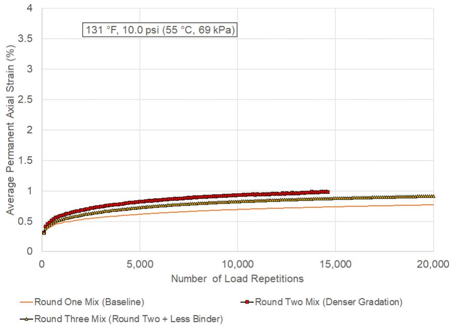
**Figure 6.11: Comparison of permanent axial strain accumulation curves for the Round One, Round Two, and Round Three mixes tested under 131°F (55°C) with 10 psi (69 kPa) confinement.**
