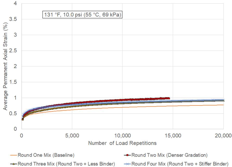
**Figure 7.11: Comparison of the permanent axial strain accumulation curves of the Round One to Round Four mixes tested under 131°F (55°C) with 69 kPa confinement.**
