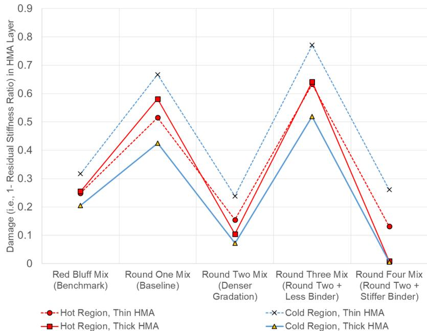
**Figure 8.2: Comparison of damage in the HMA layer.**
