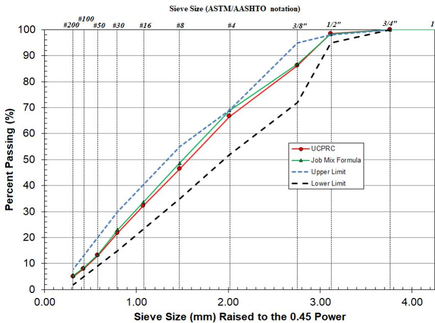
Figure 4.11: Aggregate gradation for the Round One mix.
