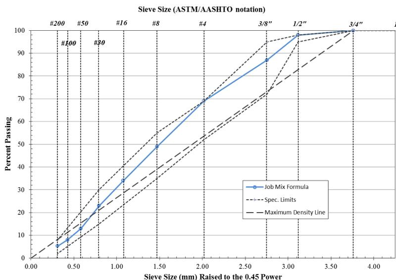
Figure 3.1: Gradation curve for the selected mix design.
