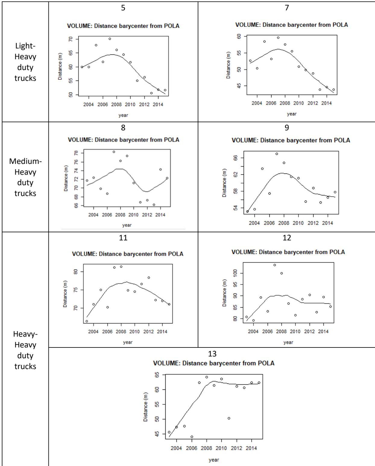
Additionally, this study identified the relationship of nine statistical measurement patterns for each combination of vehicle class and WIM station (vc-w) over time. The results demonstrated that GVW and LTR have a direct relationship, i.e., when GVW increases, LTR increases. In at least 30% of the vc-w combinations, there was an inverse relationship between volume and the mean of GVW, which mostly signifies more vehicles carrying less cargo.
