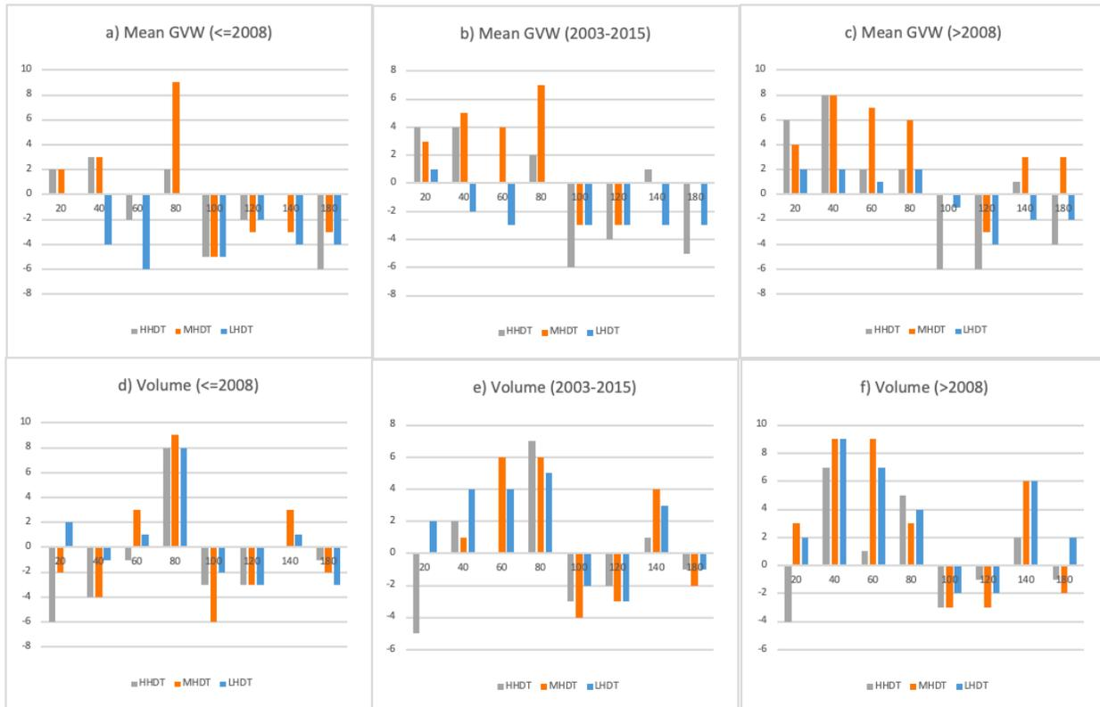
Including the temporal dimension, Figure 12 clearly shows the changes in average daily volumes for the different vehicle categories at each of the distance buffer-aggregated WIM stations.
