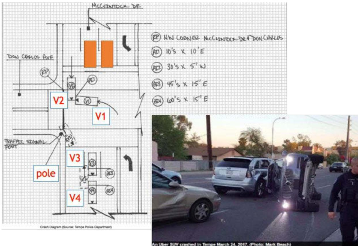
Figure 2.1: Left: diagram from the police report of an intersection where a Honda CRV ( $V_1$ ) traveling north made a left turn and collided with an Uber automated Volvo ( $V_2$ ) traveling south at 38 mph in a 40 mph zone. After the collision, the Uber Volvo hit a signal pole, and two other vehicles ( $V_3$ ,  $V_4$ ), shown in the inset. Right: the accident caused heavy damage but no one was seriously injured. Source: [23].
