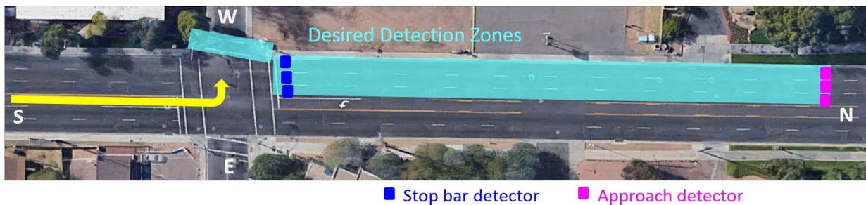
Figure 2.16: Desired detection for the south-to-west left turn movement.
