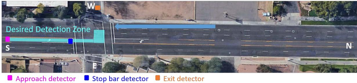
Figure 2.17: Desired detection for the north-to-south through movement.
