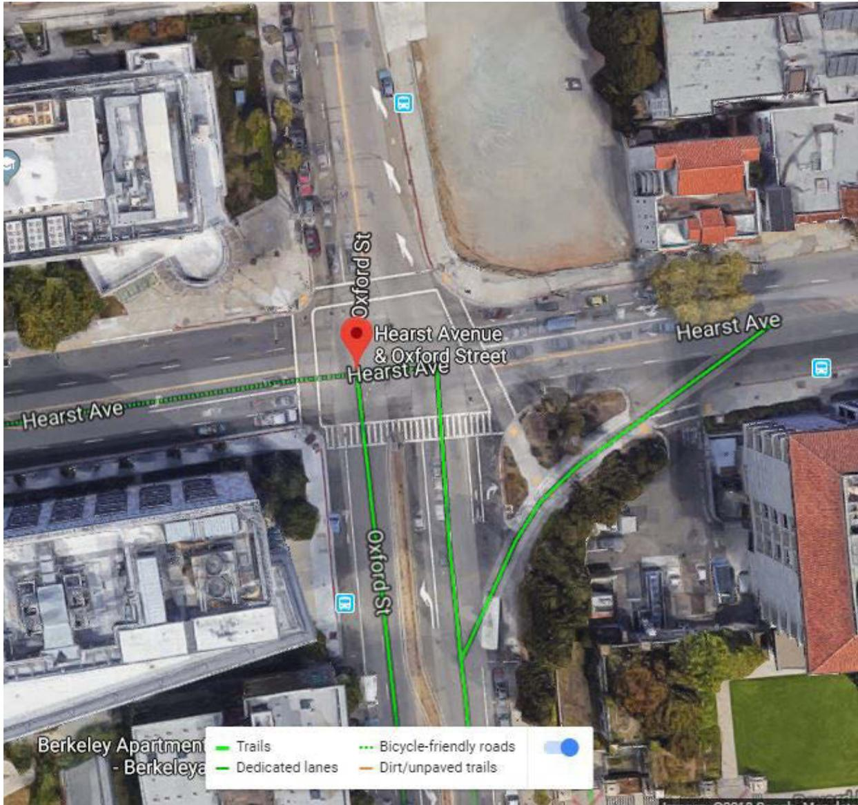
Figure 2.23: Sample intersection with 4 approaches, left-turn lane + bicycle lane
