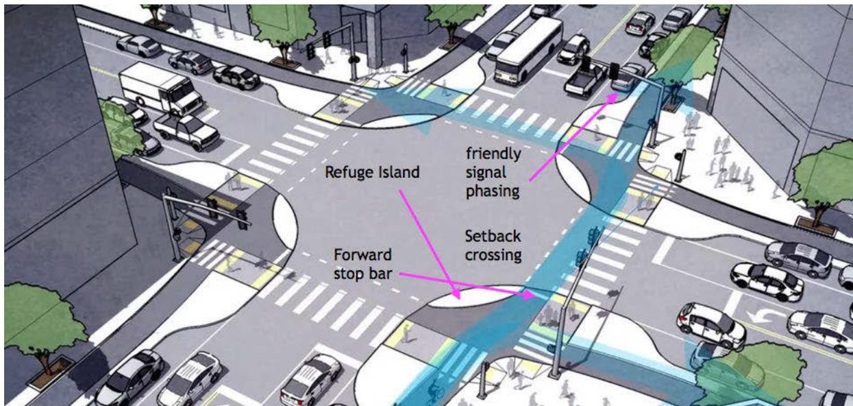
Figure 2.21: Schematic of a protected intersection. Source: [16]
