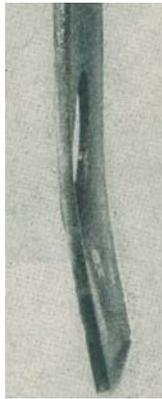
Figure 2-10: Dishing failure (Johnston, 1939).
