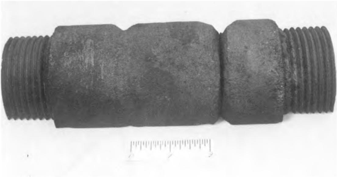
Figure 2-7: Cracked MoDOT pin removed from service.
