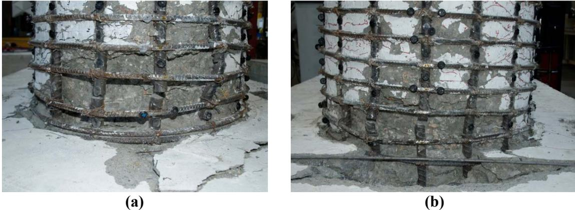
**Figure 4-7. (a) South side final damage state; (b) North side final damage state**
