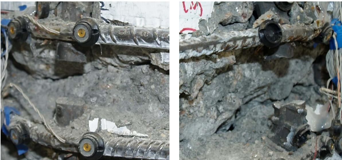
**Figure 7-5. Column test bar fracture surfaces**
