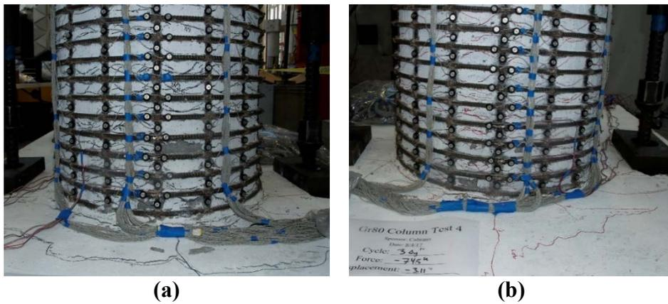
Figure 4-75. Onset of footing concrete "uplift": (a) South,  $\mu_4^{1+}$ ; (b) North,  $\mu_3^{1-}$
