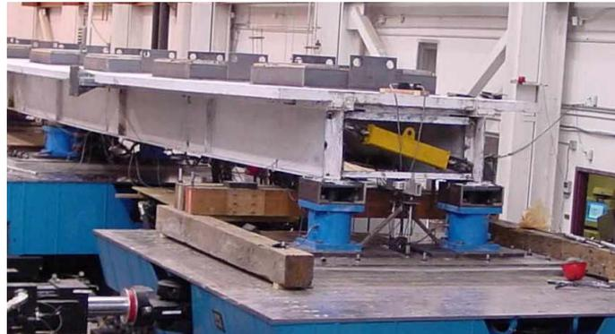
Figure 2.6 Ductile end diaphragm using BRB experimental setup by Carden et al. 2004.
