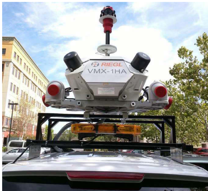
Figure 7.4: Riegl VMX-1HA sensor pod mounted on a custom roof rack
