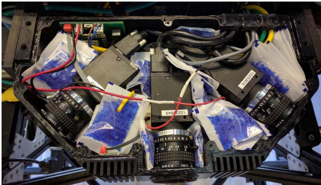
Figure 2.12: MX8 front camera housing packed with silica gel (blue packs) desiccant to keep the lenses from fogging
