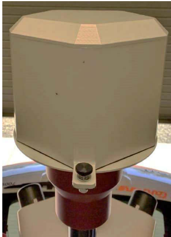
Figure 7.6: Custom 3D-printed Ladybug camera cap 3D-printed by DOE staff
