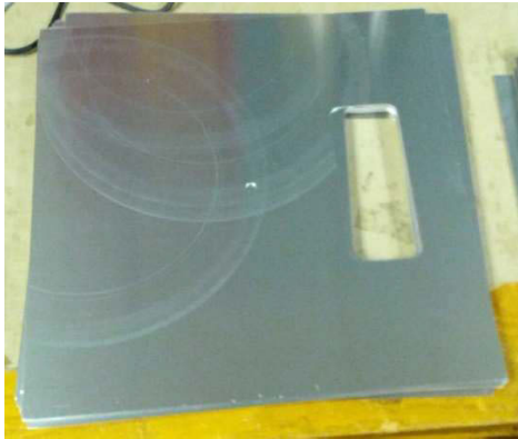
Figure 4.1: 2' x 2' MTLs target template (made by Caltrans DOE)
