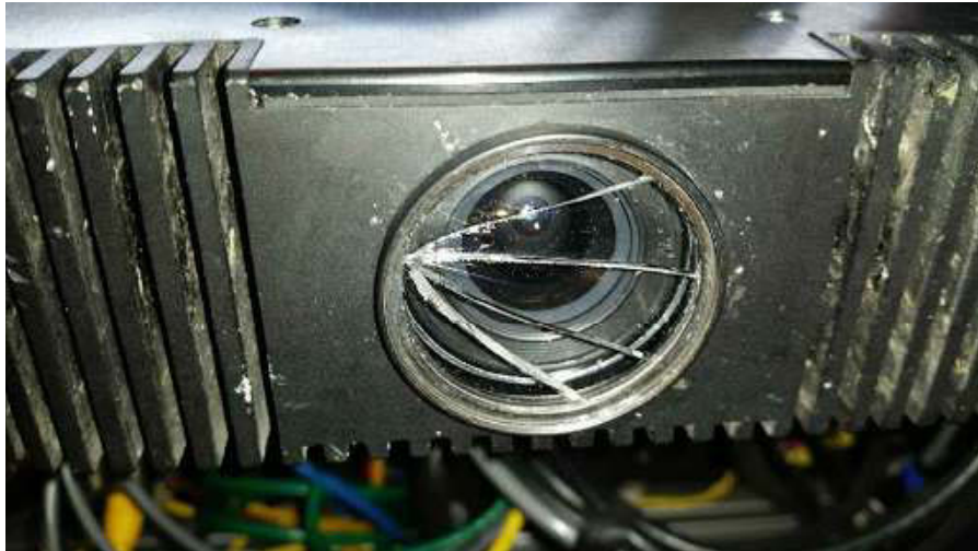
Figure 2.6: Broken front-center camera filter from shipping
