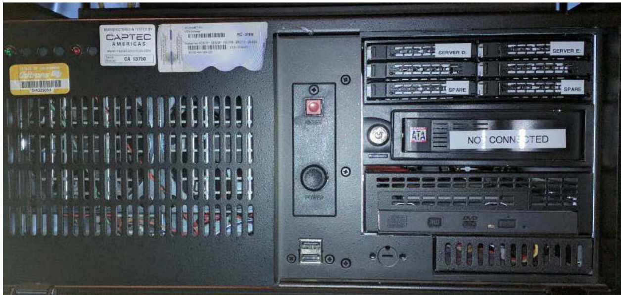
Figure 2.13: Six bay 2.5” trayless drive cage installed on the MX8 server
