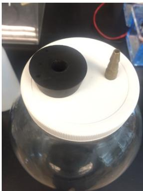
Image 1: Glass jar lid with #8 rubber stopper and air nozzle connector.
