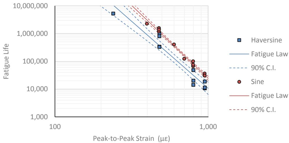
**Figure 3.5: Fatigue laws for mix DG20 C600 (50% stiffness reduction failure criterion).
