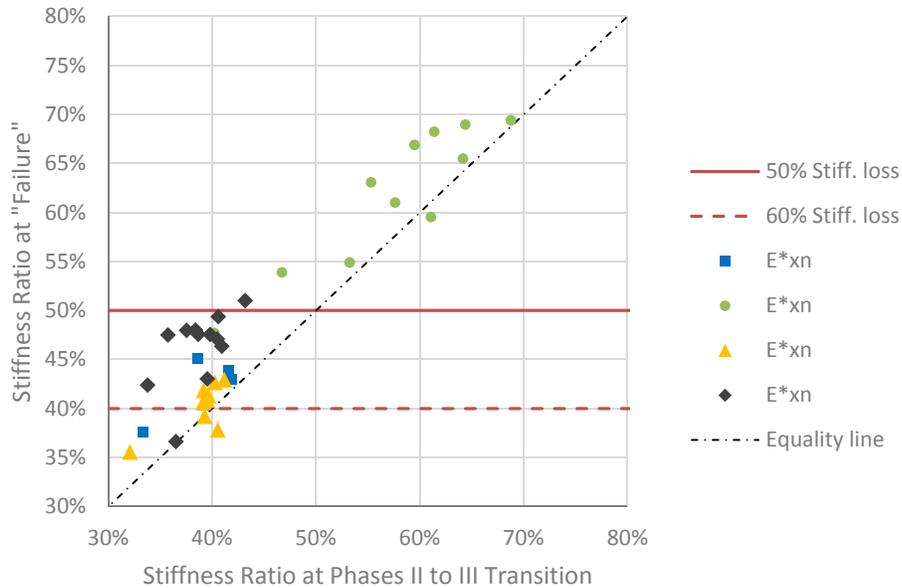
Figure 3.18: Stiffness ratio at failure, according to the three failure criteria (50 and 60 percent stiffness reduction and maximum of  $|E^*|_{xn}$ ).
