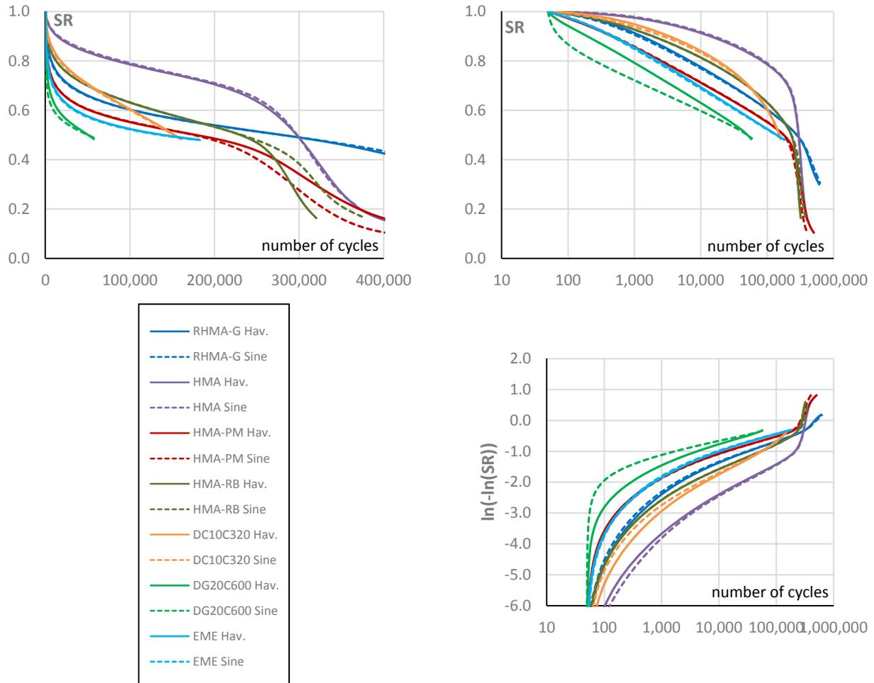
**Figure 3.12: Shape of the stiffness degradation curves (SR vs. number of cycles).**
