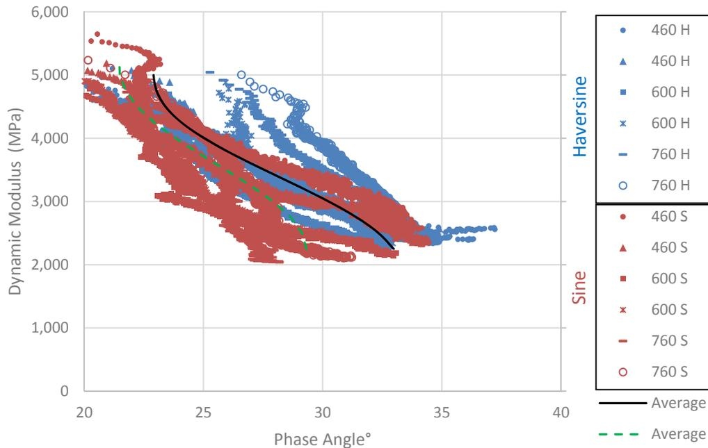
**Figure 3.14: Haversine versus sine comparison for mix EME in a Black space.**
