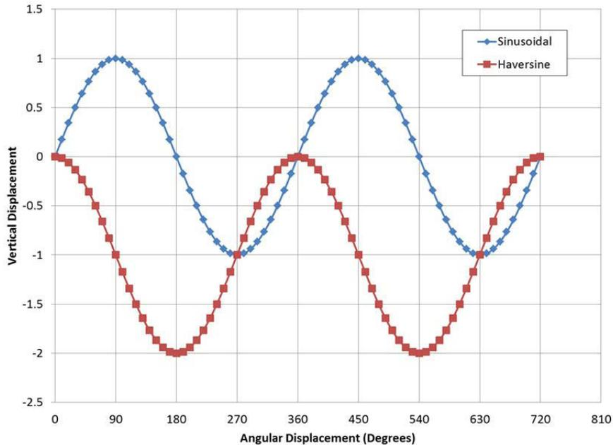
**Figure 1.1: Illustration of sinusoidal and haversine waveforms for vertical displacement.**
