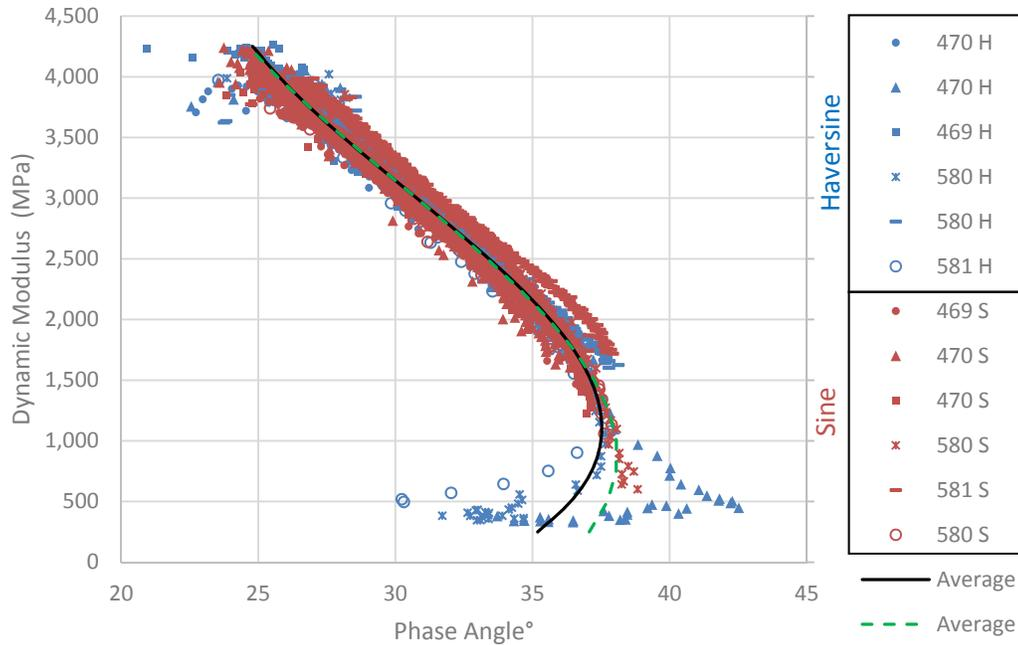
**Figure 3.13: Haversine versus sine comparison for mix RHMA-G in a Black space.**
