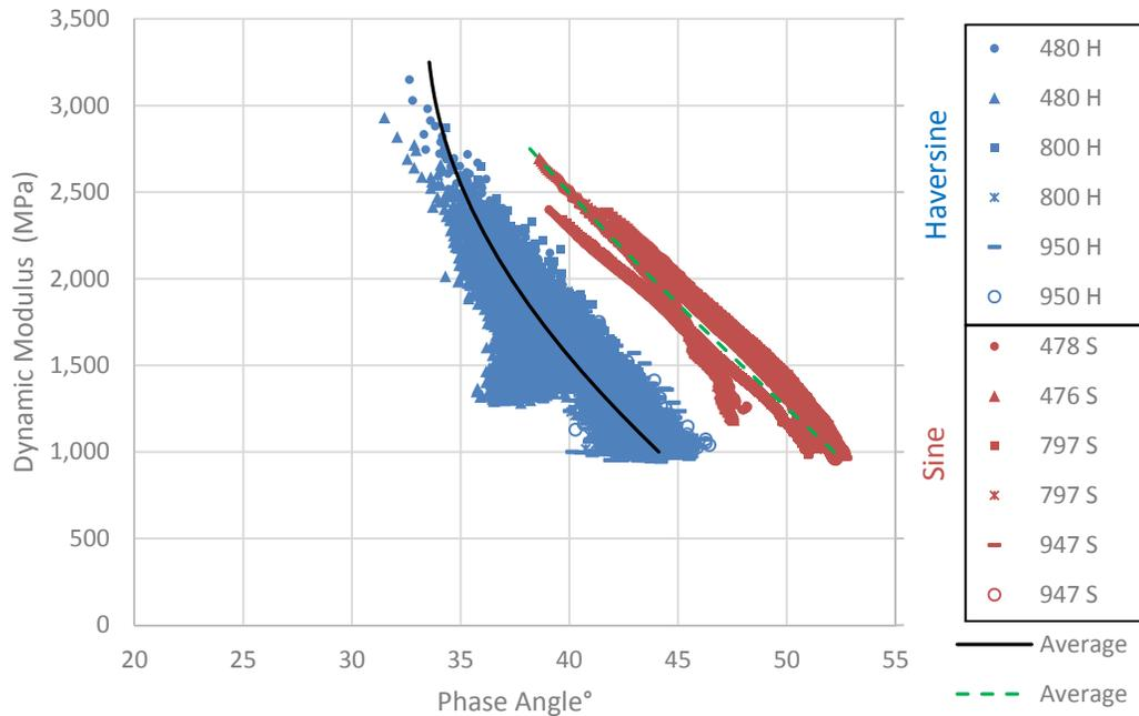
**Figure 3.15: Haversine versus sine comparison for mix DG20 C600 in a Black space.**
