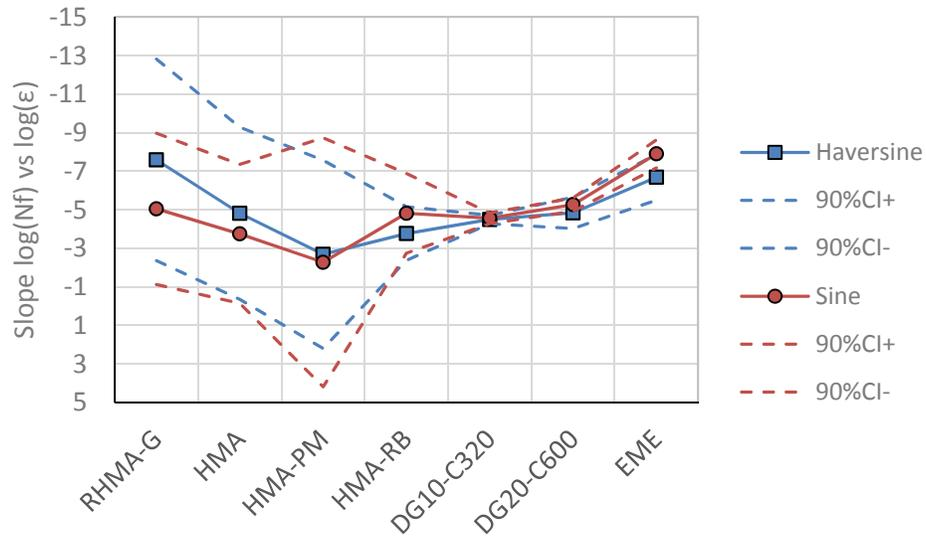
**Figure 3.7: Slope of the fatigue law,  $\log(N_f)$  versus  $\log(\epsilon)$  (50% stiffness reduction failure criterion).**
