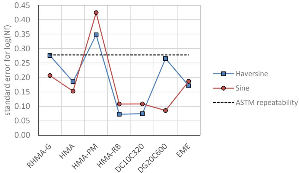
**Figure 3.8: Standard error of the fitting,  $\log(N_f)$  versus  $\log(\epsilon)$  (50% stiffness reduction failure criterion).**
