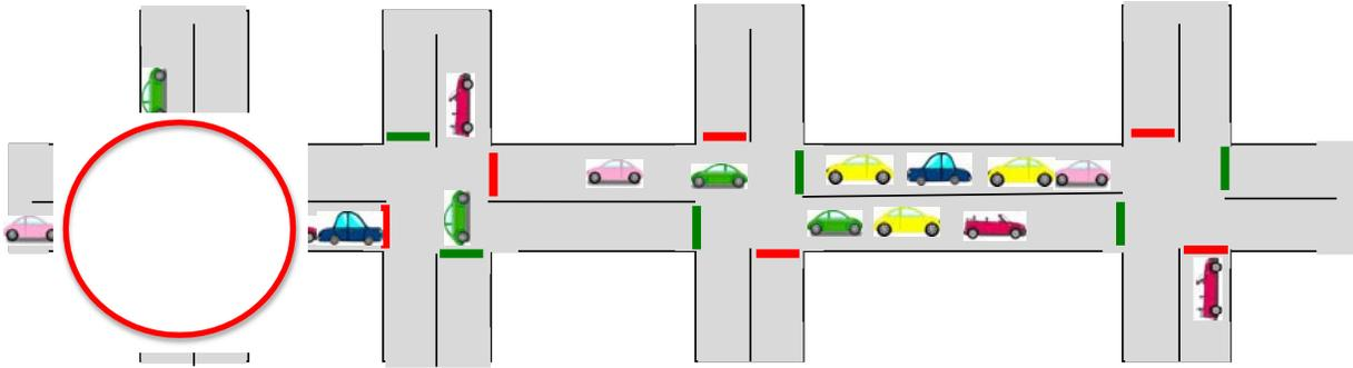
Figure 4.2 Queue Spillback at an Arterial Network
