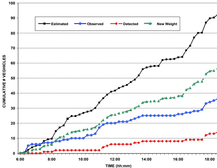
**Figure 3.5 Cumulative Count Curves: Leg 2 Through Movement**
