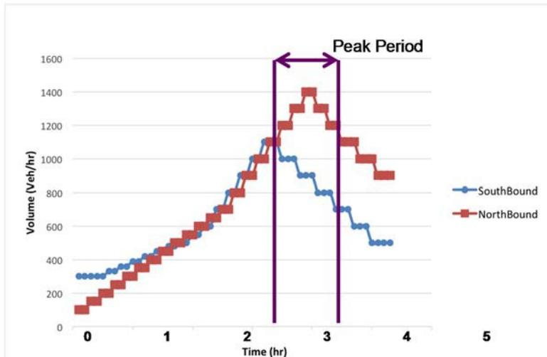
**Figure 5.3 San Pablo Avenue Flow Profile for Real Time Offset Adjustments**
