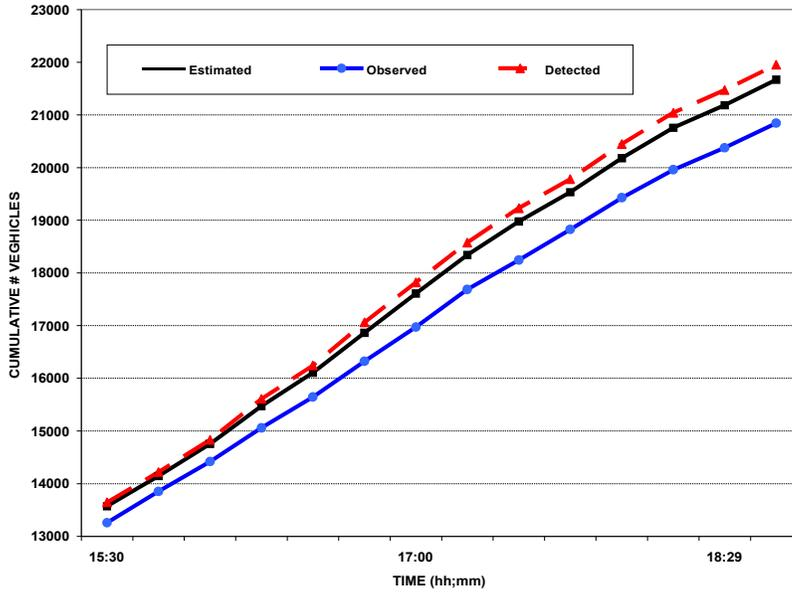
**Figure 3.4 Cumulative Count Curves: Leg 3 Through Movement-Peak Period**
