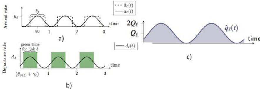
a) Vehicle arrival on non-entry links b) Vehicle departure over time c) Queue length over time
