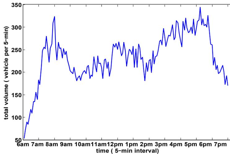
**Figure 2.2 Total Traffic Volume at Test Intersection (#veh/5-min)**
