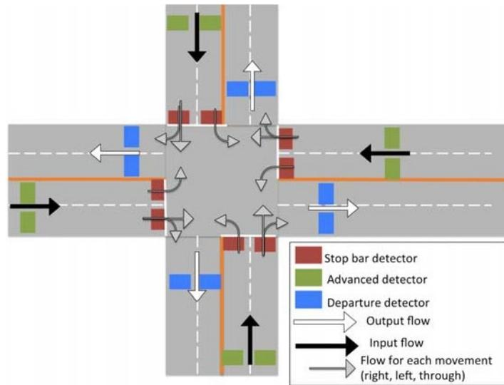
**Figure 3.1 Typical 4 Legged Signalized Intersection**
