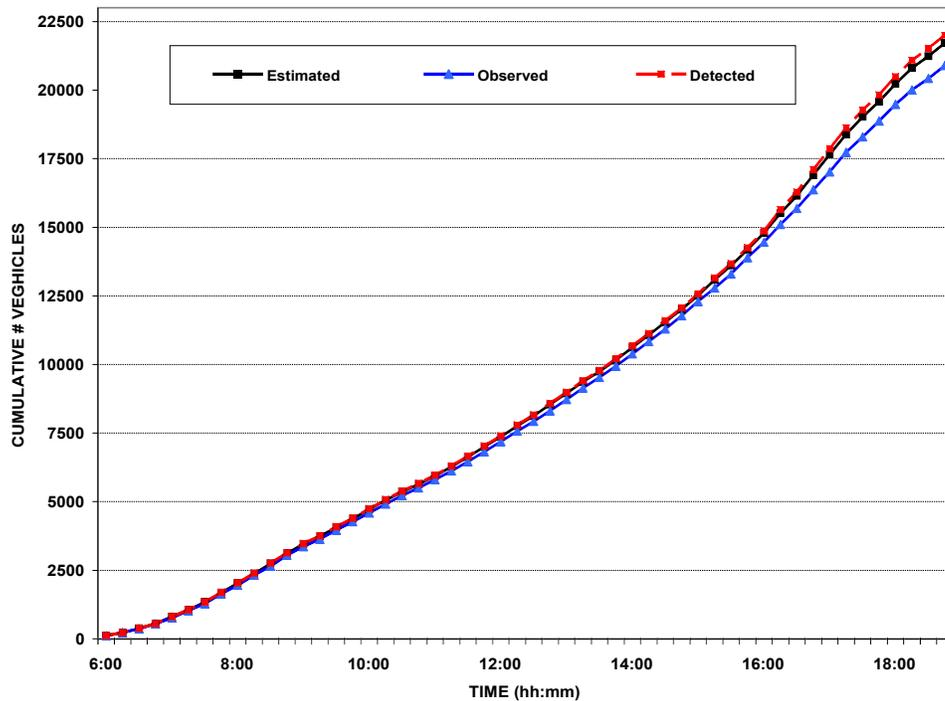
**Figure 3.3 Cumulative Count Curves: Leg 3 Through Movement - 13hr Time Period**
