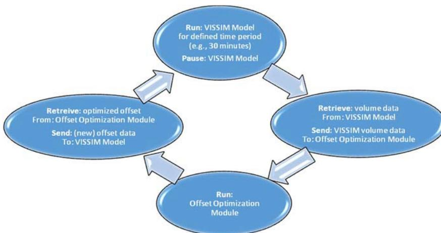
**Figure 5.2 Control of VISSIM Model and Offset Optimization Module**
