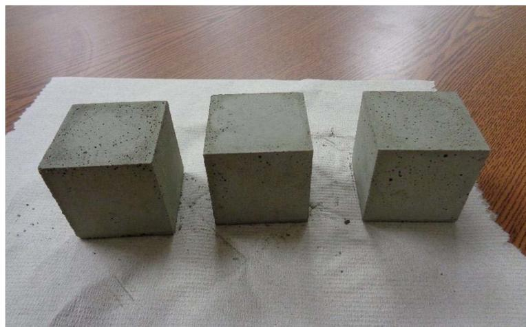
**Figure 2-14 Grout Samples for Compressive Strength Test**
