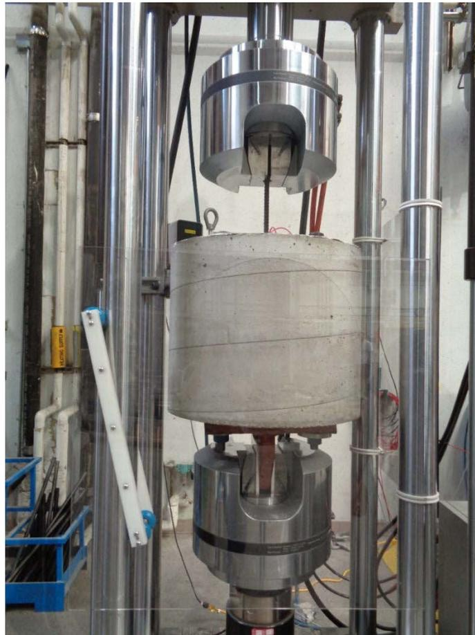
**Figure 2-47 Pullout Test Setup**
