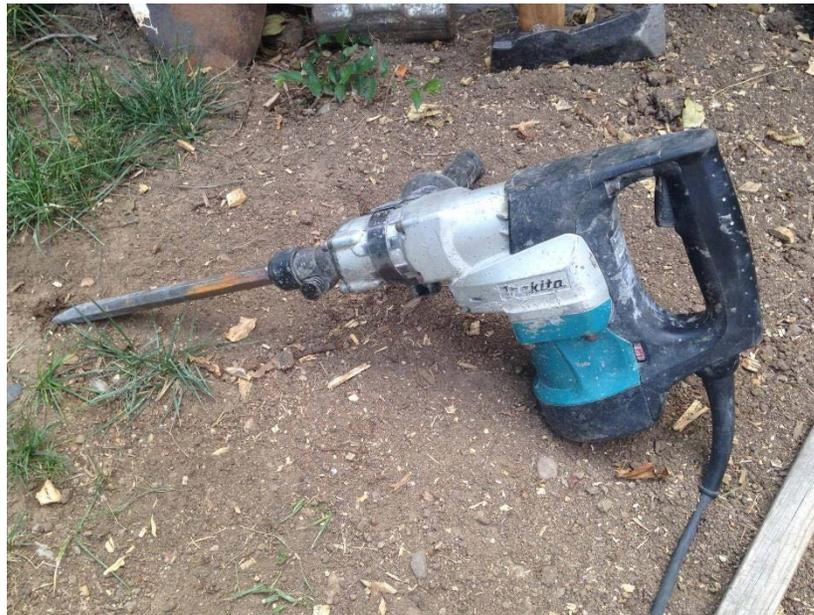
**Figure 2-34 Chipping Hammer used for Grout Removal**
