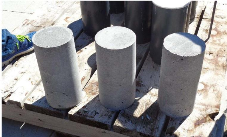
**Figure 2-12 Concrete Cylinders for Compressive Strength Test**
