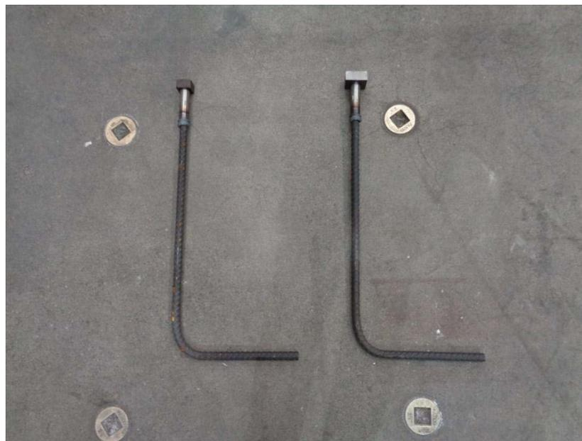
**Figure 2-19 Headed Anchor (Left: Head Area =  $4A_b$ ; Right: Head Area =  $9A_b$ )**
