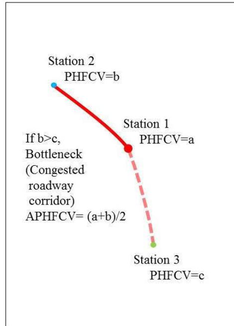
Figure 2.4-5 Steps of calculating average peak hour freight congestion value in the rest of California (using the PeMS data)
