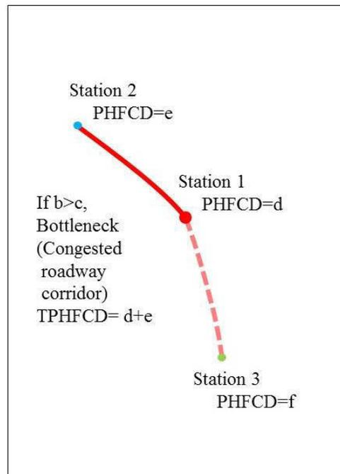
Figure 2.4-6 Steps of calculating total peak hour freight congestion delay in the rest of California (using the PeMS data)
