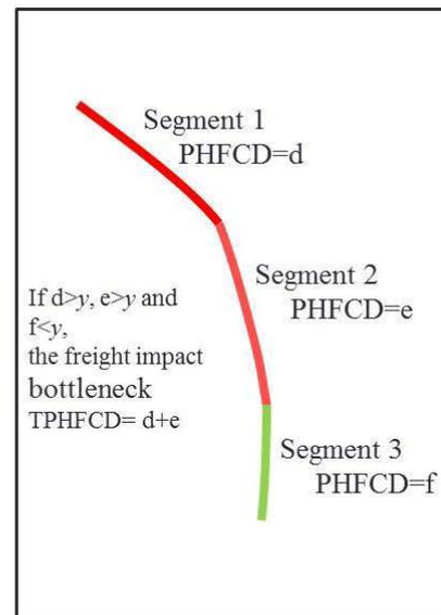
Figure 2.3-2 Steps for calculating total peak hour freight congestion delay
