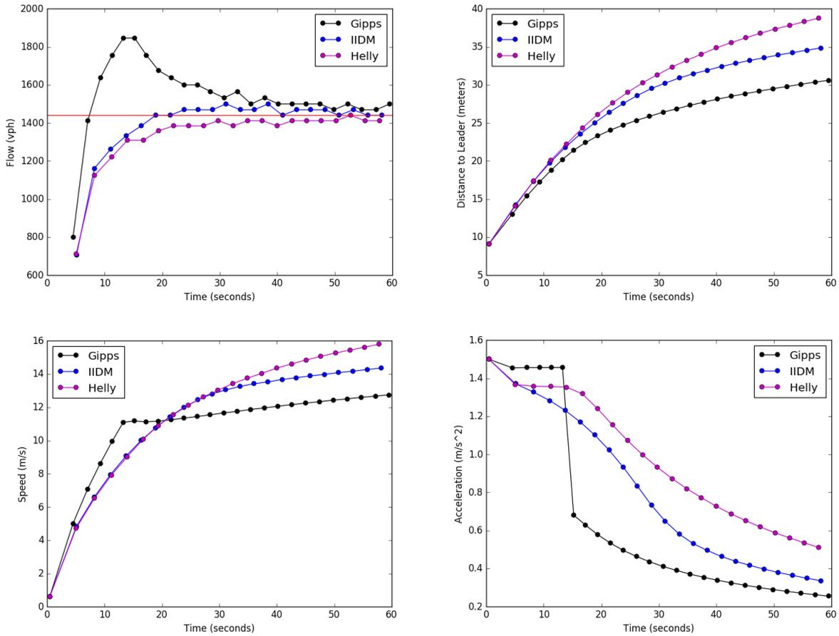
Figure 2.15: Experiment with a free road ahead: comparison of point measurements of flow, distance to leader, speed and acceleration at the detector location between the three car following models.
