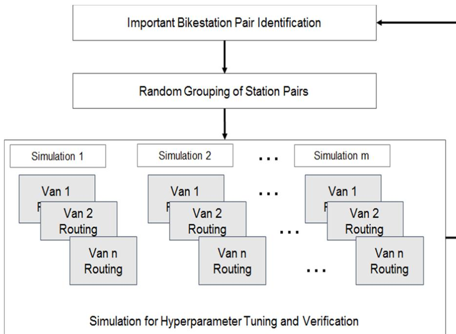
FIGURE 4.1 Conceptual Explanation of the Heuristic Solution Algorithm
