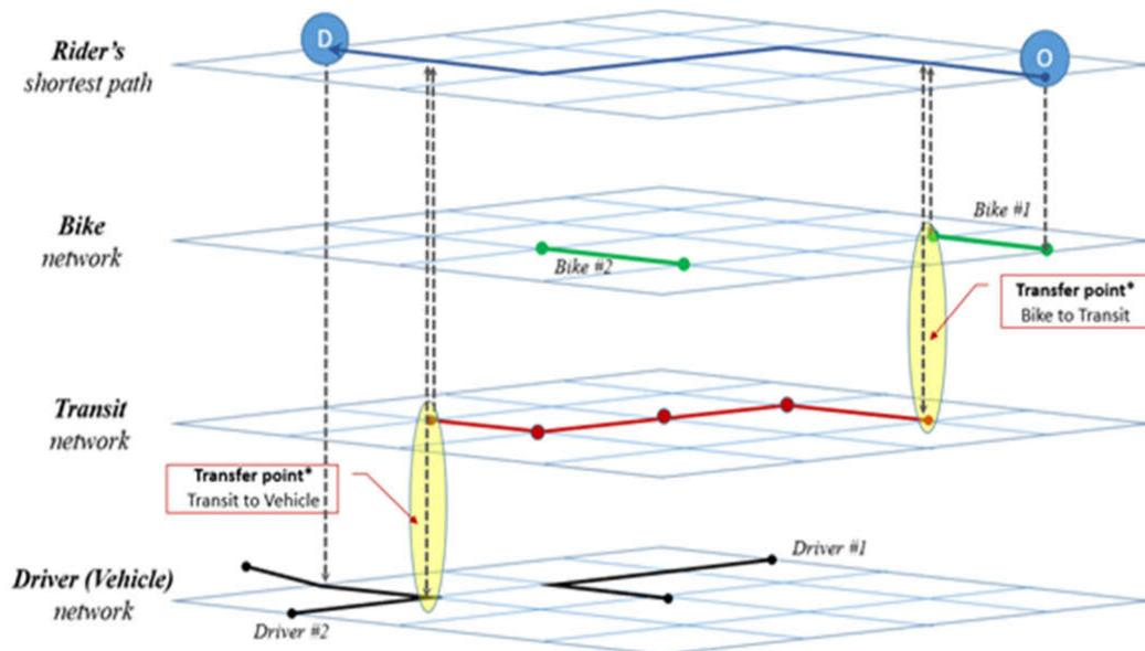
Figure 3.1 Multi-modal layers for the transit-feeder system.
