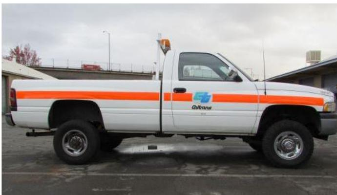
The addition of decals and a light bar to the pickup on the left is considered to be up fitting.
