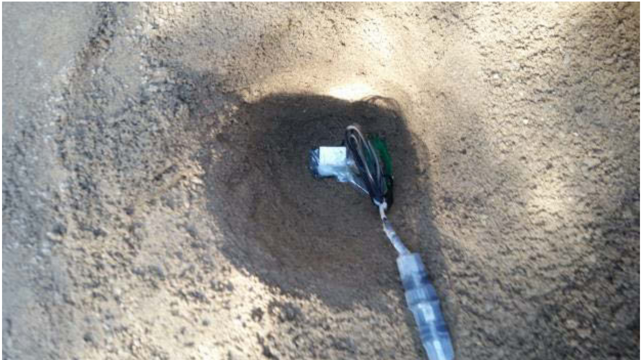
Figure A–10: Placement of accelerometer during backfilling
