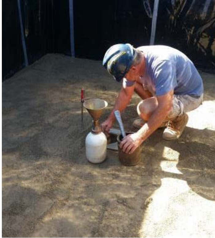
Figure A–9: Verification of the achieved soil density during backfilling from sand cone test
