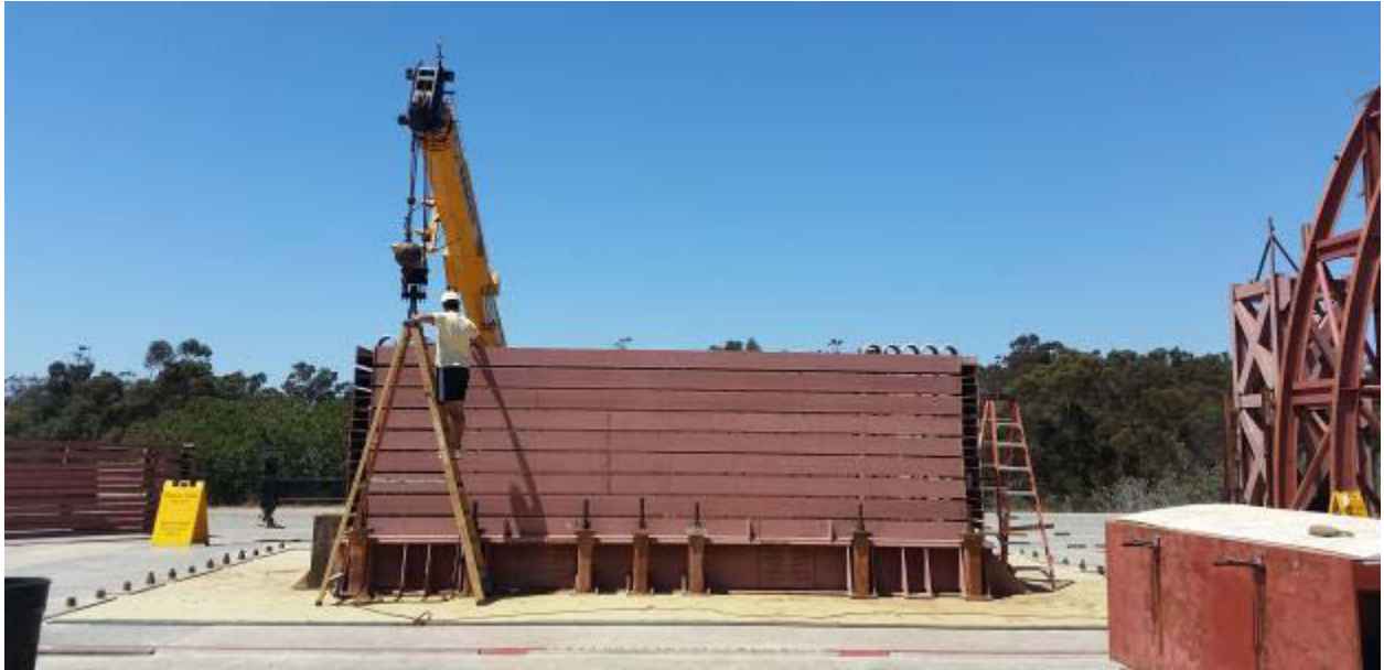
Figure A-3: Assembly of the laminar soil container frames
