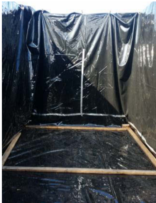
Figure A-4: Plastic lining inside the laminar soil container (the wood was removed during backfill)
