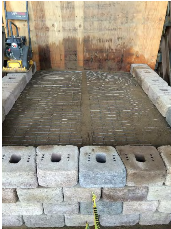
Figure A2.6 Transverse reinforcement layers for Test 5.
