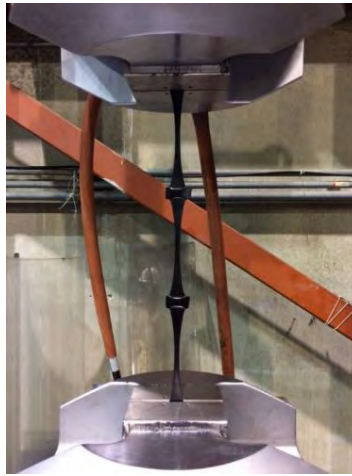
Figure 3.11 Single-rib tensile test setup.
