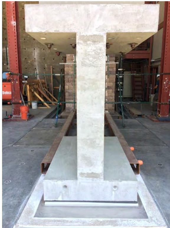
Figure A2.16 Support wall on the sliding platform.
