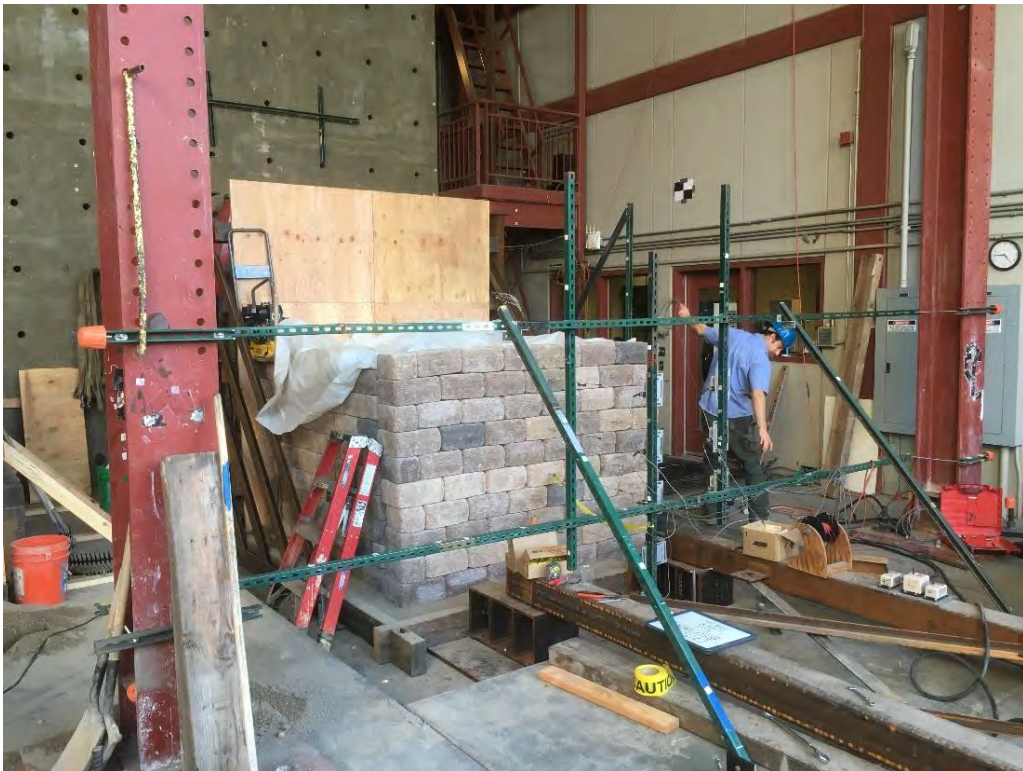
Figure A2.12 Placement of plastic cover to prevent loss of moisture.
