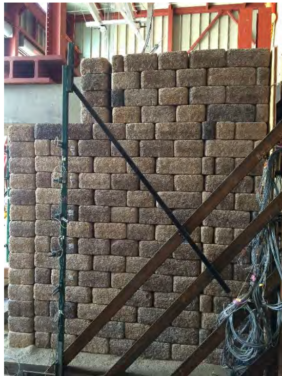
Figure A2.22 Constructed specimen for Test 1.
