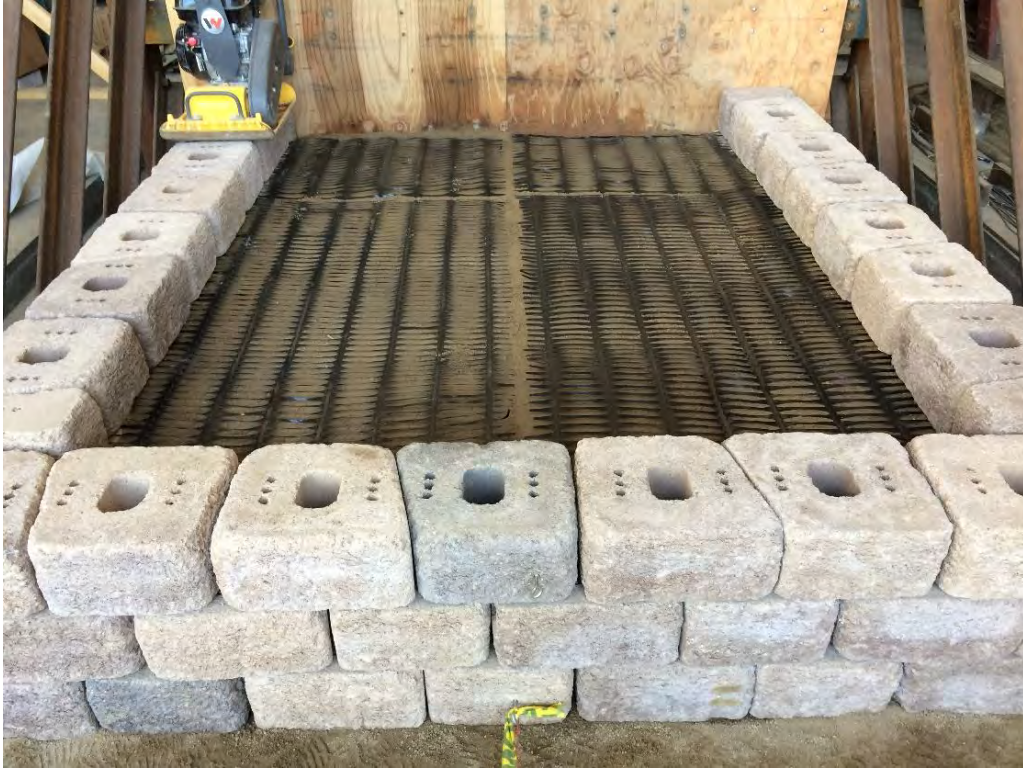
Figure A2.5 Transverse reinforcement layers.
