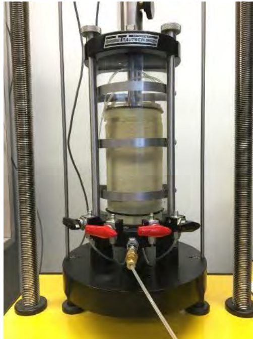
Figure 3.7 Consolidated drained triaxial compression test setup.
