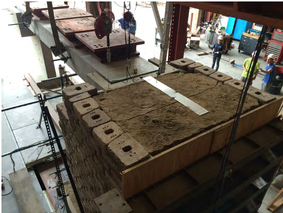
Figure A2.42 Top view after the Maule motion for Test 4.
