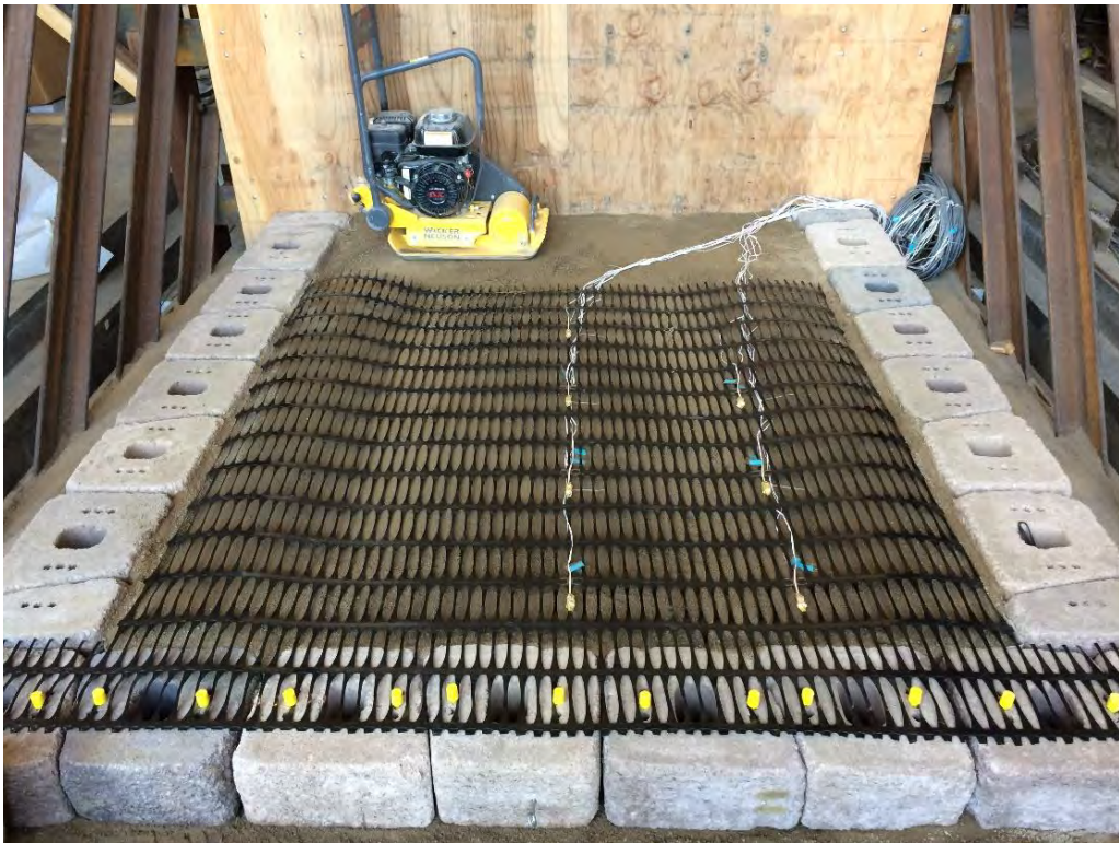
Figure A2.4 Longitudinal reinforcement layer.
