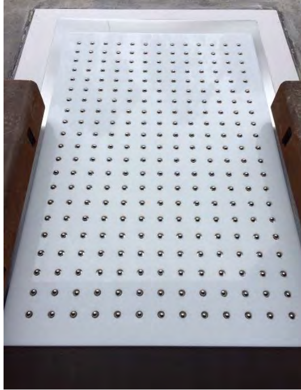
Figure A2.15 Ball bearings on the stainless steel plate.
