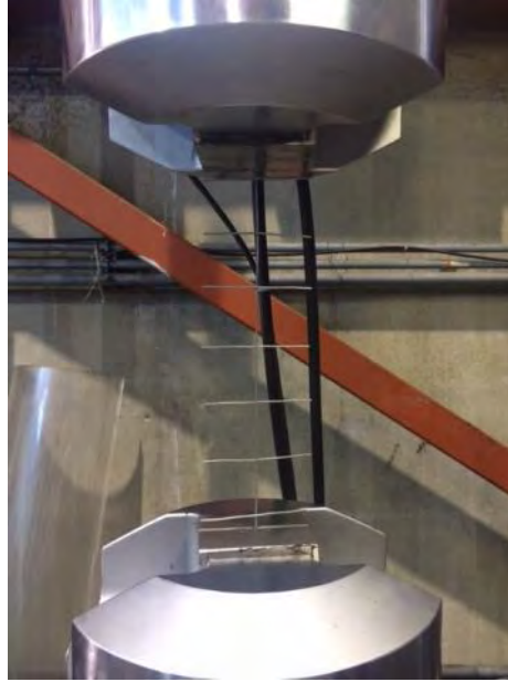
Figure 3.15 Tensile test on steel welded wire mesh.
