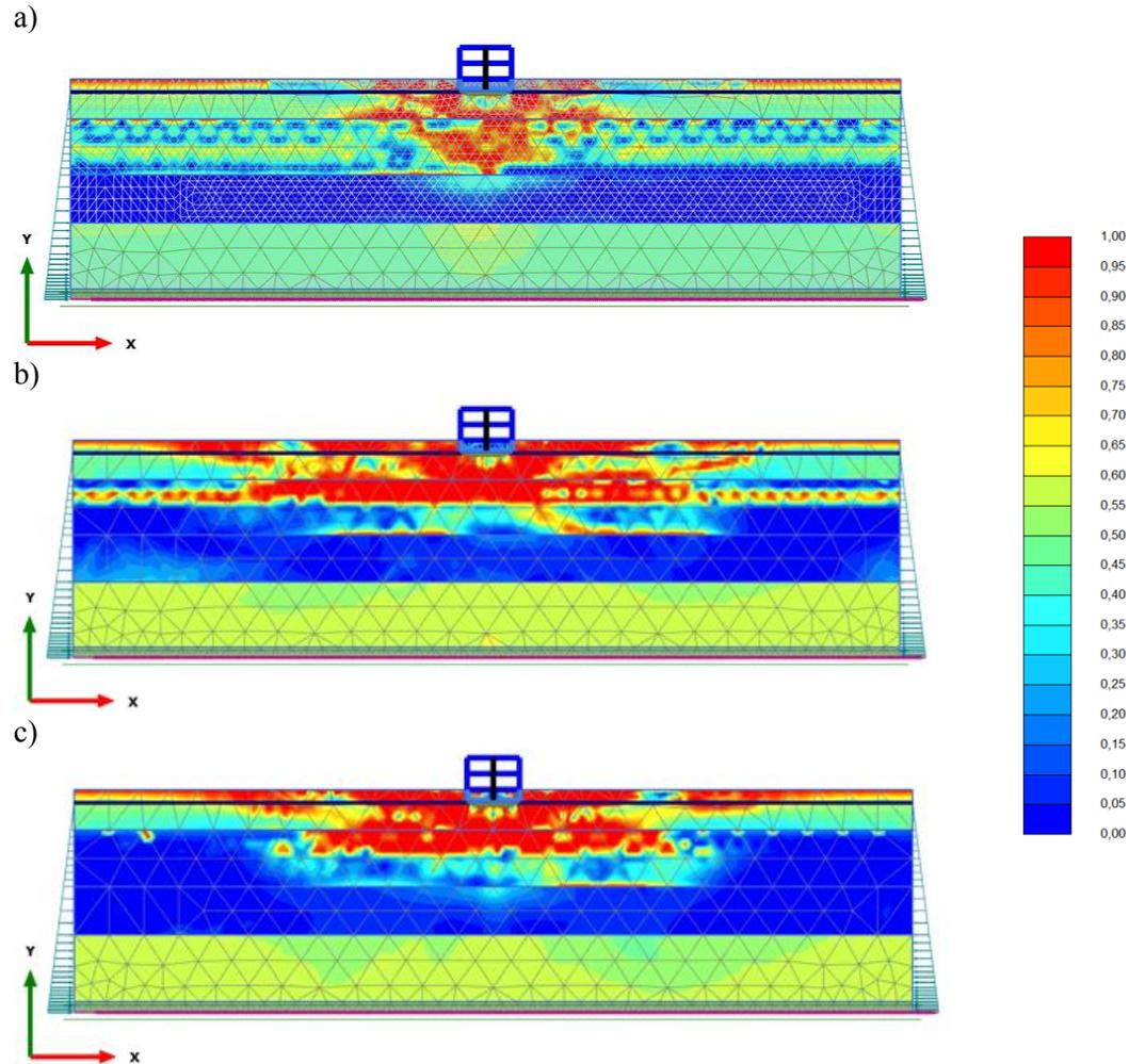
**Fig. 75.** Relative shear stress ( $\tau_{relative}$ ) contours for a site supporting a 2-story hypothetical structure when subjected to the OLE conditions: a) Whittier 1987, b) Imperial Valley 1979, and c) Superstition Hill 1987.
