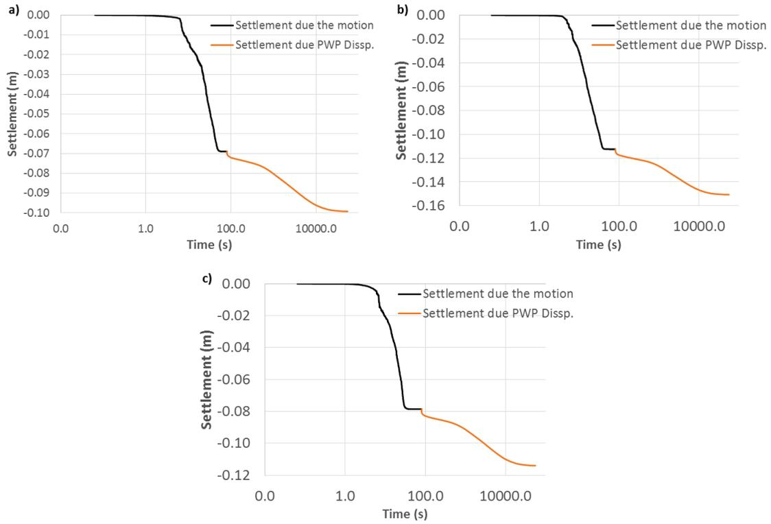
**Fig. 71.** Development of ground surface settlements versus time as induced during the earthquake and during the pore water pressure dissipation phase for OLE condition: a) Whittier 1987, b) Imperial Valley 1979, and c) Superstition Hill 1987.
