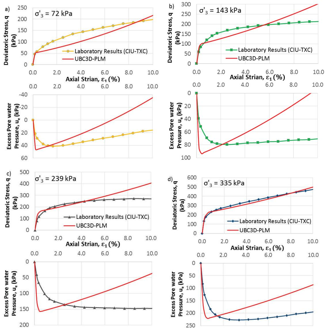
**Fig. 50.** Comparison of CIU-TXC test results and numerical simulations using UBC3D-PLM model in PLAXIS 2D for different confining pressures: a)  $\sigma'_c=72$  kPa, b)  $\sigma'_c=143$  kPa, c)  $\sigma'_c=239$  kPa and d)  $\sigma'_c=335$  kPa.
