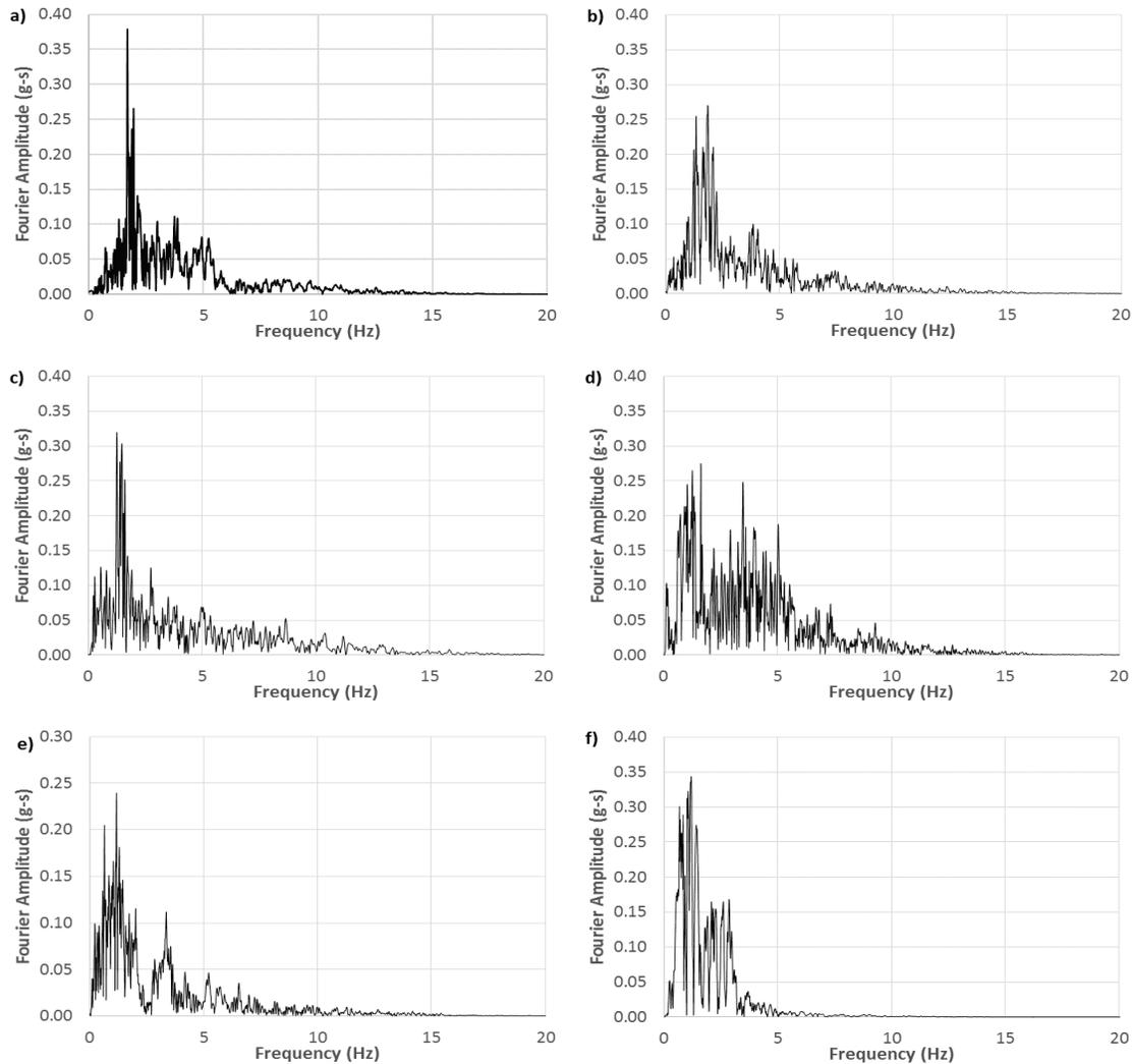
**Fig. 67.** Fast Fourier amplitude at the top ground surface with DEEPSOIL for the OLE condition a) Whittier 1987, b) Imperial Valley 1979, c) Superstition Hill 1987 and CLE condition d) Duzce 1999 e) Imperial Valley 1979 and f) Kobe 1995.
