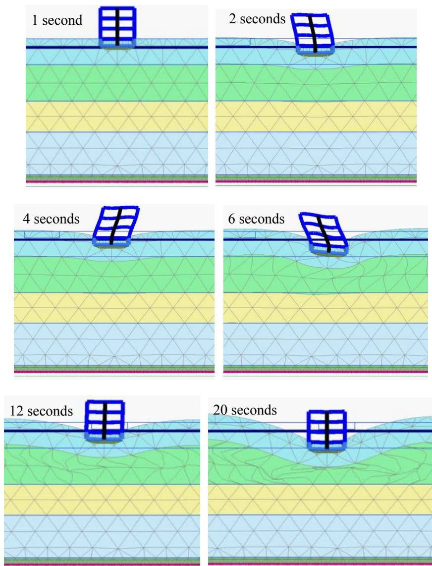
**Fig. 79.** Deformation contours of hypothetical 3-story structure for different times during the Imperial Valley CLE earthquake.
