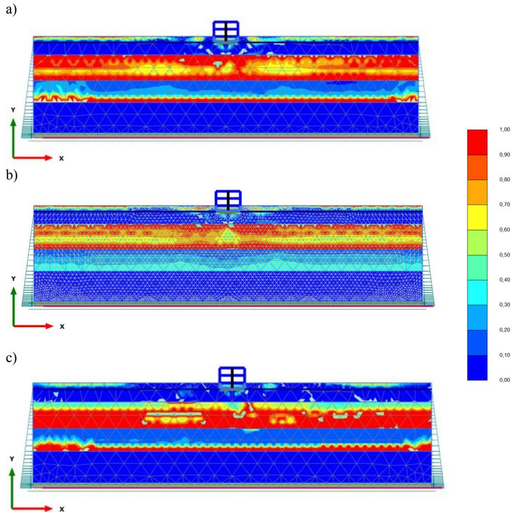
**Fig. 74.** Pore water pressure ratio ( $r_u$ ) contours for a site supporting a 2-story hypothetical structure when subjected to the CLE conditions: a) Duzce 1999 b) Imperial Valley 1979, and c) Kobe 1995.
