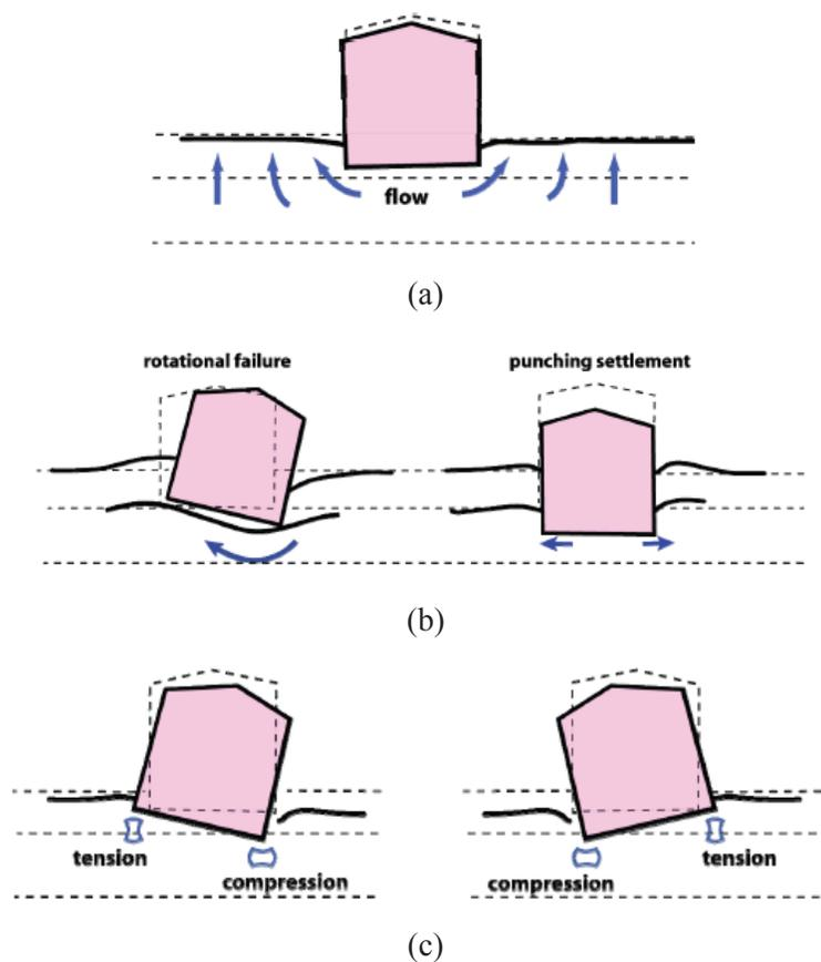
**Fig. 15.** Primary liquefaction-induced displacement mechanisms: (a) volumetric strains caused by water flow in response to transient gradients; (b) partial bearing capacity failure as a result of soil softening; (c) liquefaction-induced building ratcheting during earthquake loading (Dashti and Bray 2013).
