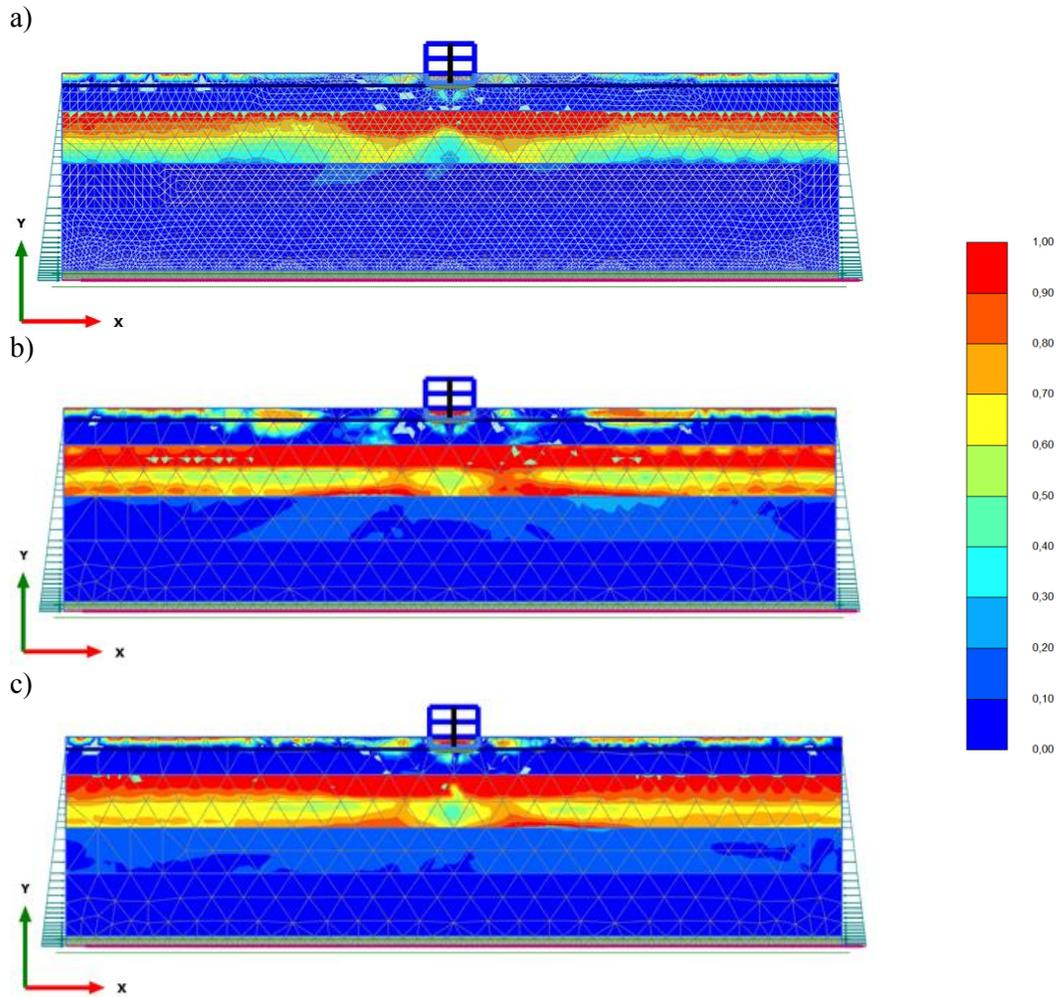
**Fig. 73.** Pore water pressure ratio ( $r_u$ ) contours for a site supporting a 2-story hypothetical structure when subjected to the OLE conditions: a) Whittier 1987, b) Imperial Valley 1979, and c) Superstition Hill 1987.
