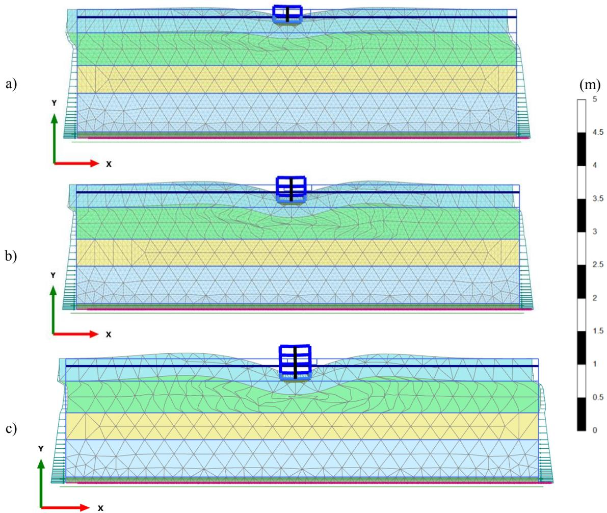
**Fig. 78.** Deformation contours for different hypothetical structure types including one basement level when subjected to the Imperial Valley CLE earthquake: a) 1-story structure, b) 2-story structure, and c) 3-story structure.
