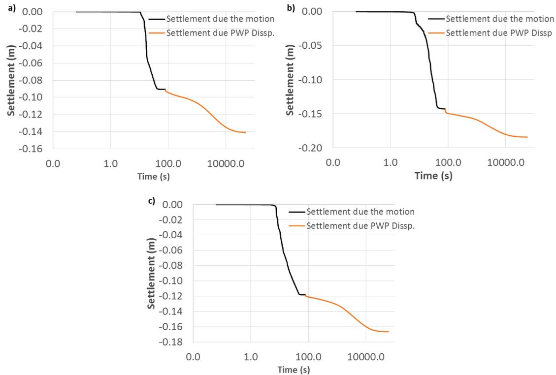
**Fig. 72.** Development of ground surface settlements versus time as induced during the earthquake and during the pore water pressure dissipation phase for CLE condition: a) Duzce 1999 b) Imperial Valley 1979, and c) Kobe 1995.
