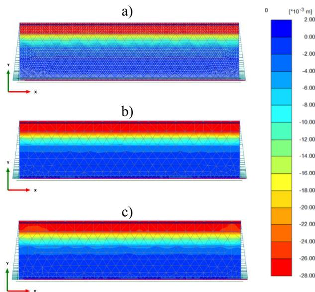
**Fig. 60.** Maximum vertical deformation contours for the OLE condition after the pore water pressure dissipation a) Whittier 1987, b) Imperial Valley 1979, and c) Superstition Hill 1987.
