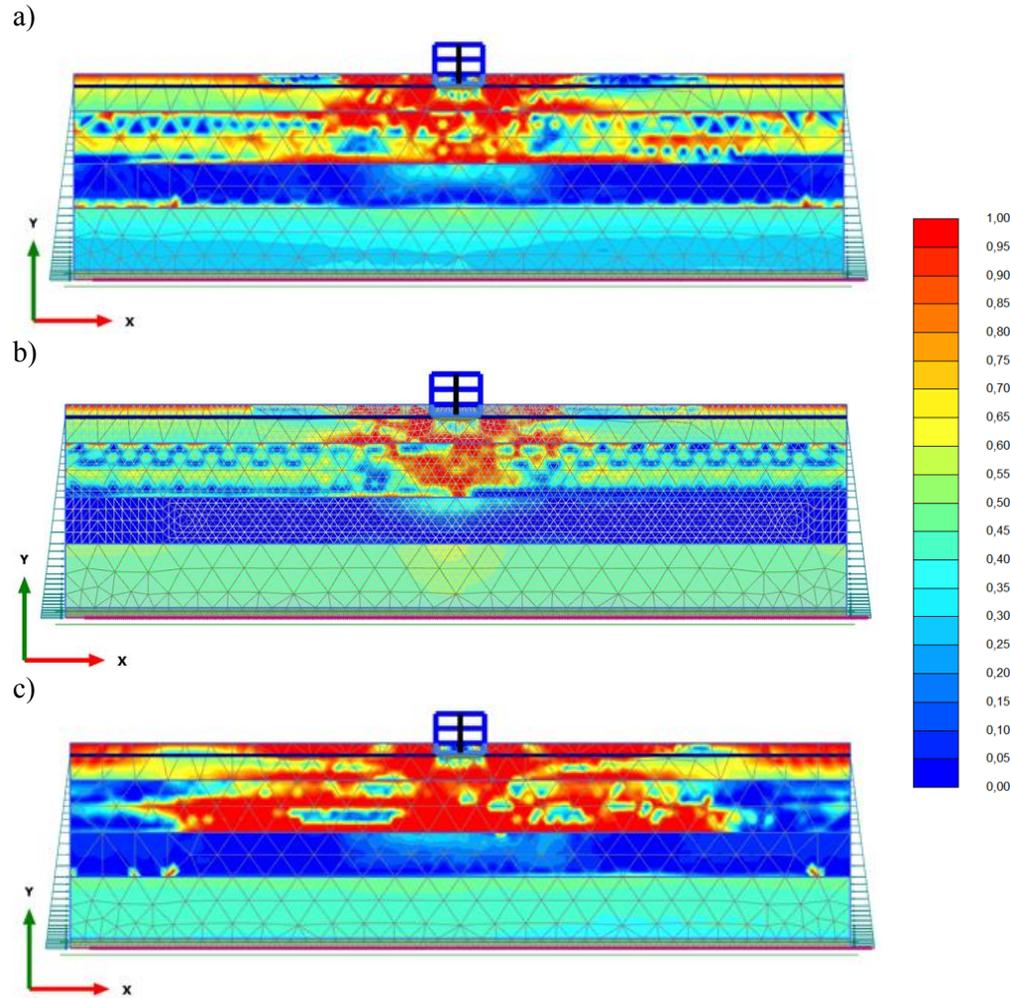
**Fig. 76.** Relative shear stress ( $\tau_{relative}$ ) contours for a site supporting a 2-story hypothetical structure when subjected to the CLE conditions: a) Duzce 1999 b) Imperial Valley 1979, and c) Kobe 1995.
