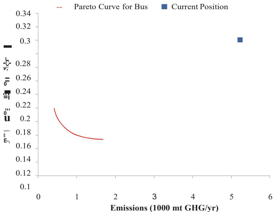
**Figure 6.1 The current state of the MUNI network and the Pareto frontier**
