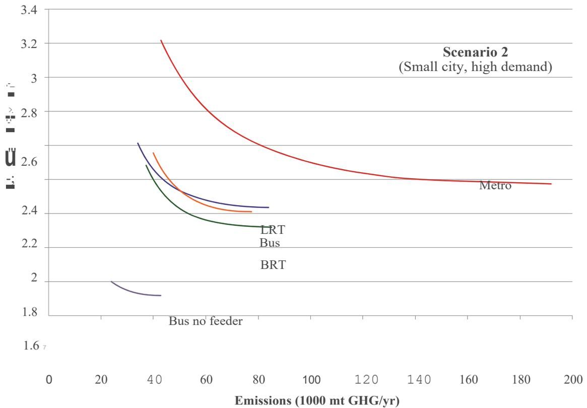
**Figure 4.2** Technology-specific Pareto curves of system costs with varying transit emissions
