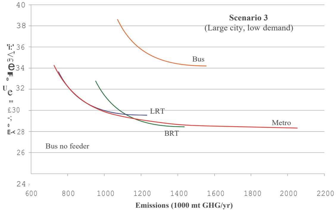
**Figure 4.3 Technology-specific Pareto curves of system costs with varying transit emissions (scenario 3)**
