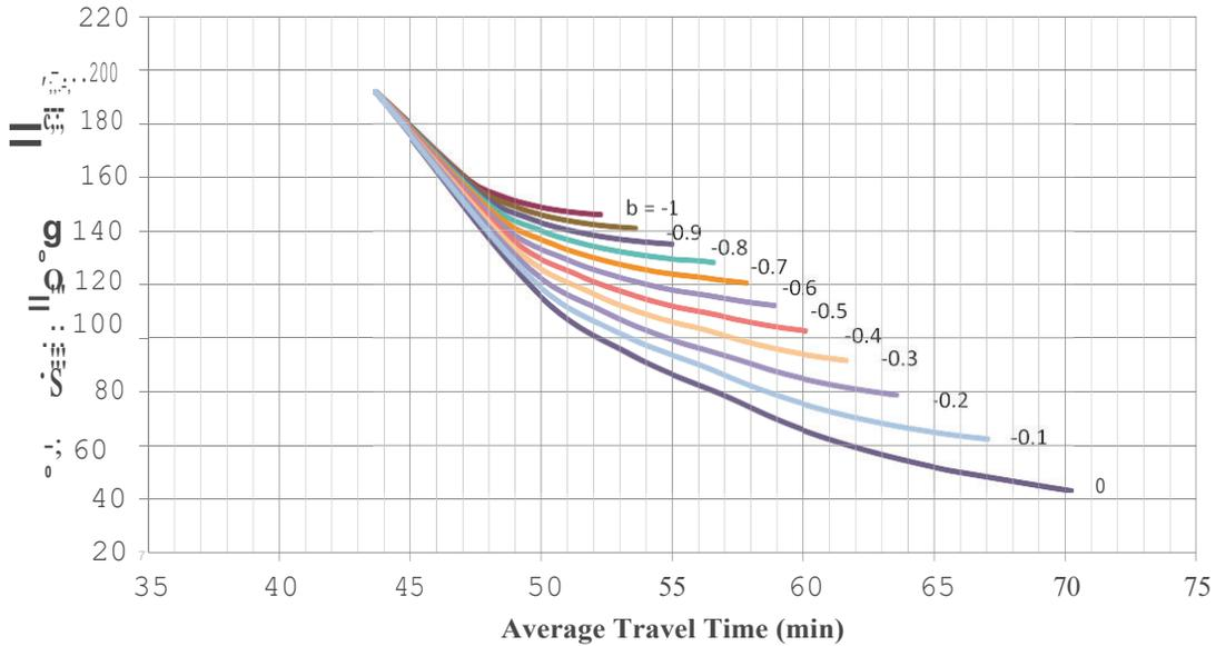
**Figure 4.11 Change in total emissions as LOS is reduced for metro under a city-wide emissions budget (scenario 2)**
