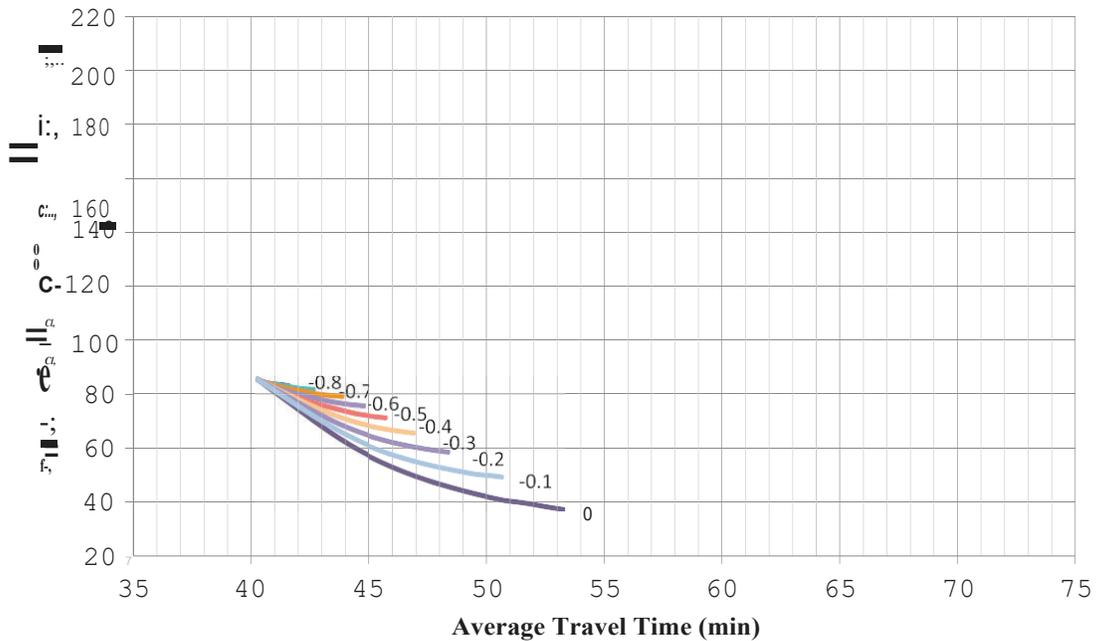
Figure 4.10 Change in total emissions as LOS is reduced for BRT under a city-wide emissions budget (scenario 2)
