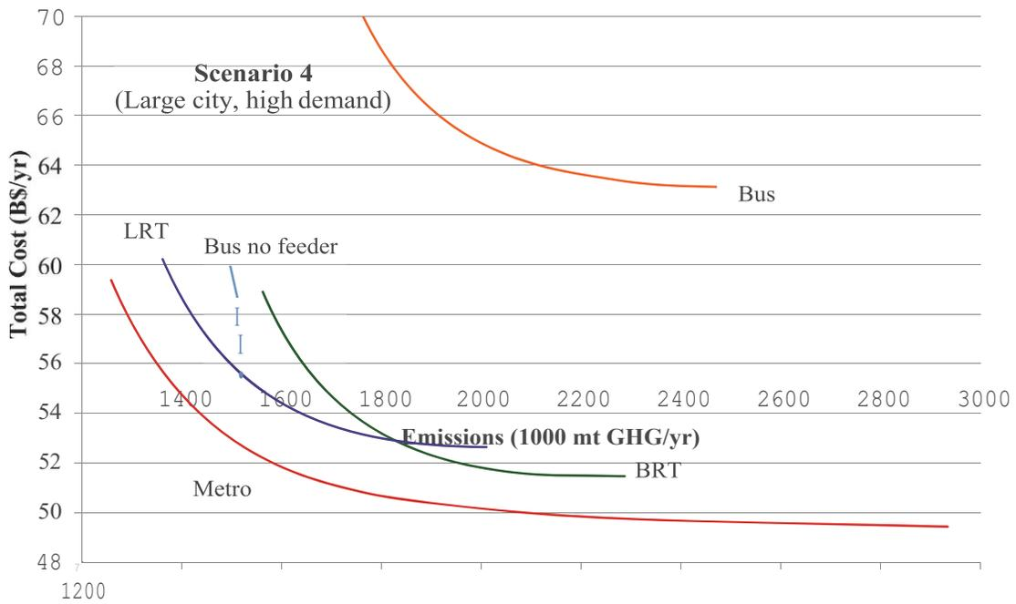
**Figure 4.4 Technology-specific Pareto curves of system costs with varying transit emissions (scenario 4)**
